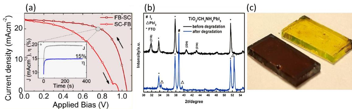
**Figure 11:** (a) Hysteresis of PSCs. Figure adapted from ref<sup>87</sup>. (b) XRD of perovskite-sensitized  $\text{TiO}_2$  before and after degradation. Figure adapted from ref<sup>89</sup>. (c) Appearance of perovskite film before and after degradation.
