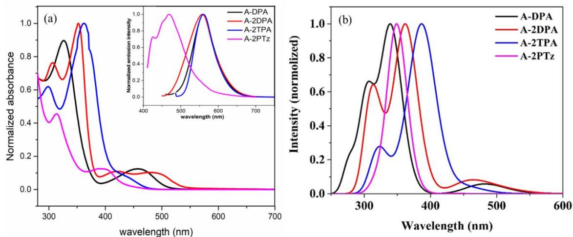
Figure 8 : (a) Experimental absorption spectra and emission spectra (inset) and (b) theoretical absorption spectra of studied compound in dilute dichloromethane
