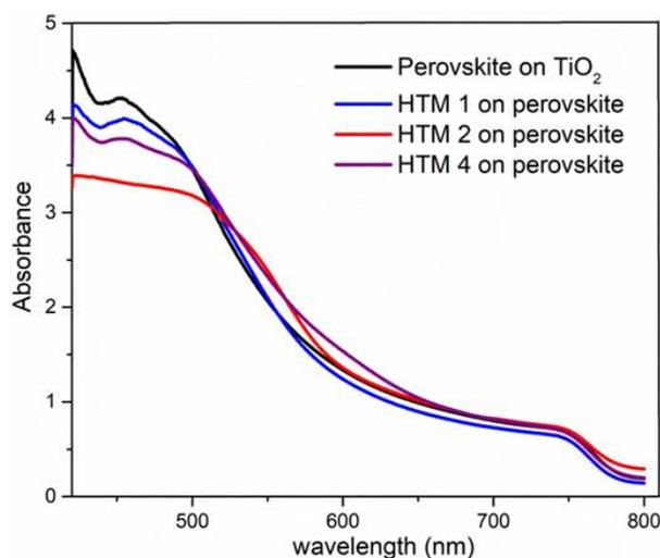
Figure 7: Comparison of absorbance of MAPbI<sub>3</sub>/TiO<sub>2</sub> and HTMs/MAPbI<sub>3</sub> films.
