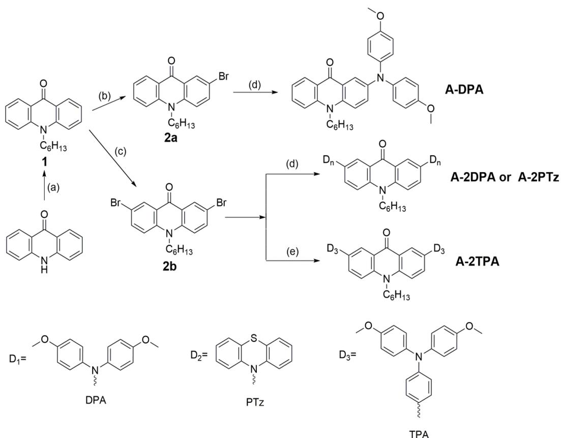
*Scheme 1: Synthesis of acridone derivatives. Reagents and conditions: (a) NaOH, C<sub>6</sub>H<sub>13</sub>Br, DMSO, 140<sup>o</sup>C, 24h. (b) NBS, CHCl<sub>3</sub>, rt, 16h. (c) NBS, DMF, 70<sup>o</sup>C, 24h. (d) D<sub>n</sub>-H, NaO<sup>t</sup>Bu, Pd(OAc)<sub>2</sub>, tBu<sub>3</sub>P, Toluene, 110<sup>o</sup>C, 48h. (e) D<sub>3</sub>-H, Pd(PPh<sub>3</sub>)<sub>4</sub>, K<sub>2</sub>CO<sub>3</sub>, Toluene, 110<sup>o</sup>C, 48h.*
