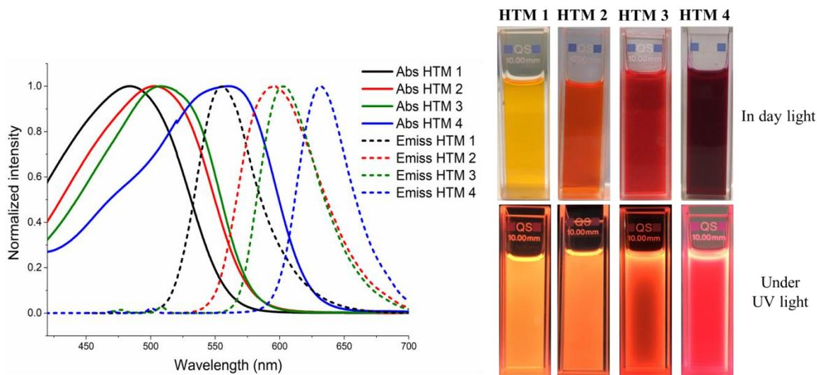
**Figure 5:** Normalized absorption- emission in solution of studied molecules in diluted dichloromethane (left) and in the right, appearance of these solutions in daily light (top) and under UV 365 nm (bottom).
