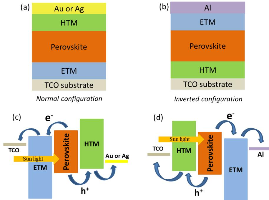
**Figure 6:** (a) Normal structure of PSCs with n-type ETM facing incoming light. (b) Inverted structure of PSCs with p-type HTM facing incoming light. (c) Mechanism of carrier transport in normal configuration and (d) Mechanism of carrier transport in inverted configuration.
