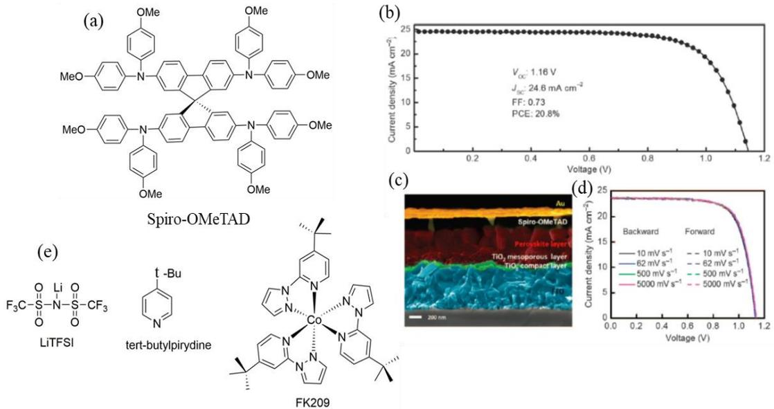
Figure 14: (a) Chemical structure of *p,p*-Spiro-OMeTAD (b) J-V characteristic of champion PSCs used Spiro-OMeTAD under AM 1.5 G illumination. (c) Cross-sectional SEM image of champion device. (d) Hysteresis measurements of one device at different scanning speeds under AM 1.5 G illumination. Figure (b-d) adapted from ref<sup>121</sup>, (e) additives/dopants most used in PSCs are Li-TFSI, *t*-BP, FK209.
