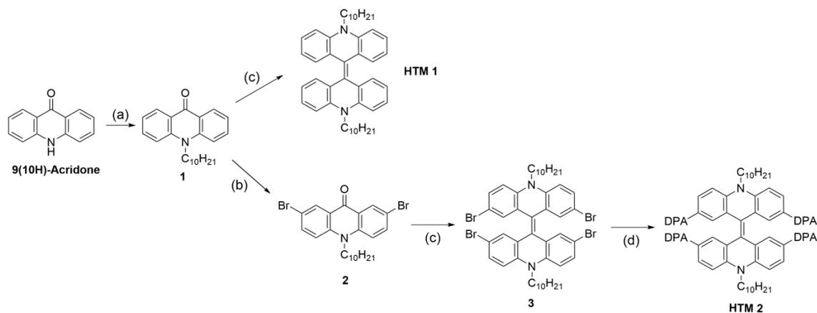
**Scheme 45:** Synthetic route of these new materials. Reagents and conditions: (a) NaOH, 1-bromodecane, DMSO, Aliquat 336, 110°C, 24h. (b) NBS, DMF, 70°C (c) Zn, THF, 0°C, TiCl<sub>4</sub>, pyridine and (d) Pd(OAc)<sub>2</sub>, tBu<sub>3</sub>P, NaOtBu, Toluene, 110°C.
