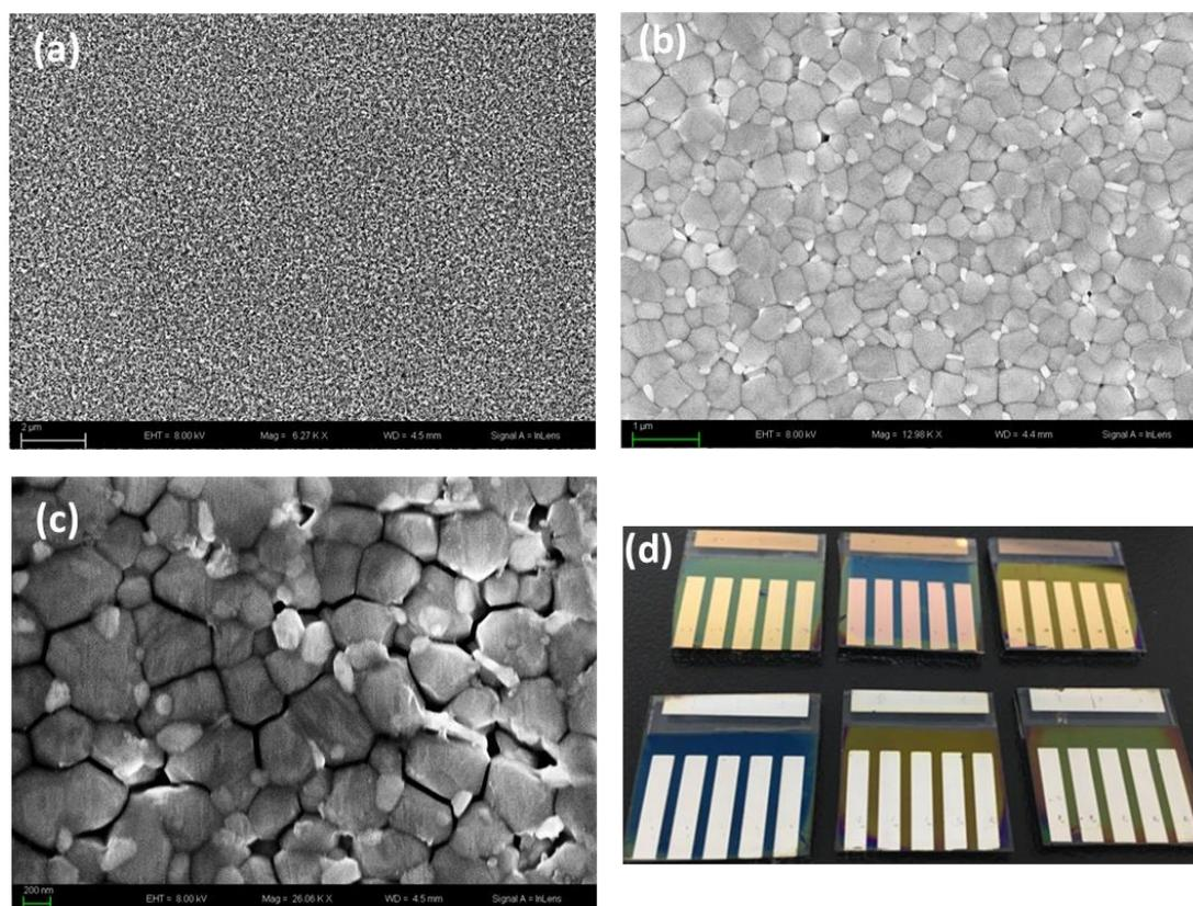
**Figure 20 :** SEM images of (a) Mesoporous  $\text{TiO}_2$  layer (scale:  $2\mu\text{m}$ ). (b) Perovskite film coated on mesoporous  $\text{TiO}_2$  layer (scale:  $1\mu\text{m}$ ) (c) Zoom in of perovskite layer with grain boundaries (scale: 200 nm). (d) Real devices with different HTMs and gold/silver as metal electrodes.
