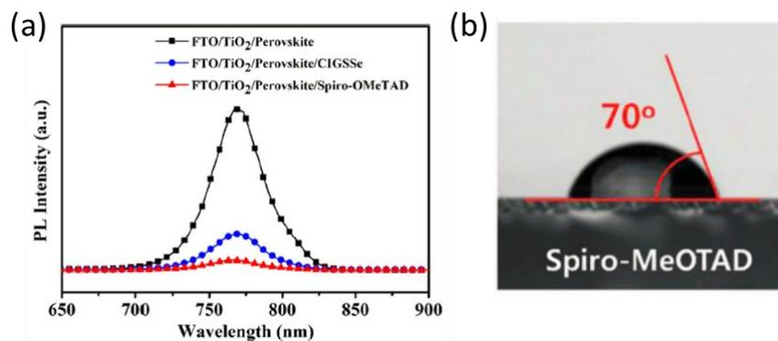
Figure 15: (a) Steady-state photoluminescence (PL) spectra for MAPbI<sub>3</sub>, MAPbI<sub>3</sub>/copper indium gallium disulfoselenide (CIGSSe), and MAPbI<sub>3</sub>/ Spiro-OMeTAD layers deposited on FTO/bl-TiO<sub>2</sub>/mp-TiO<sub>2</sub> substrates. Figure adapted from ref<sup>123</sup> (b) Water contact angles of the spiro-MeOTAD coated on FTO substrate. Figure adapted from ref<sup>124</sup>.
