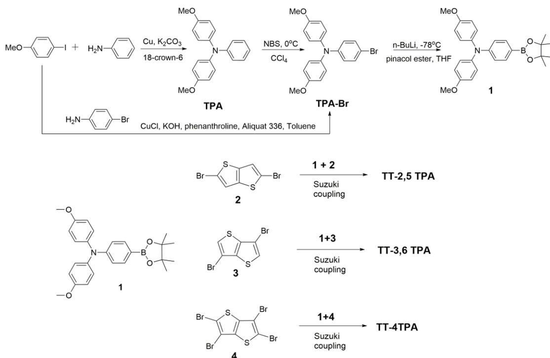
**Scheme 1: Synthetic route of Thienothiophene-based HTMs and precursors. Suzuki coupling reaction conditions : Pd(PPh<sub>3</sub>)<sub>4</sub>, K<sub>2</sub>CO<sub>3</sub>, Aliquat 336, Toluene, 110°C, 24h.**
