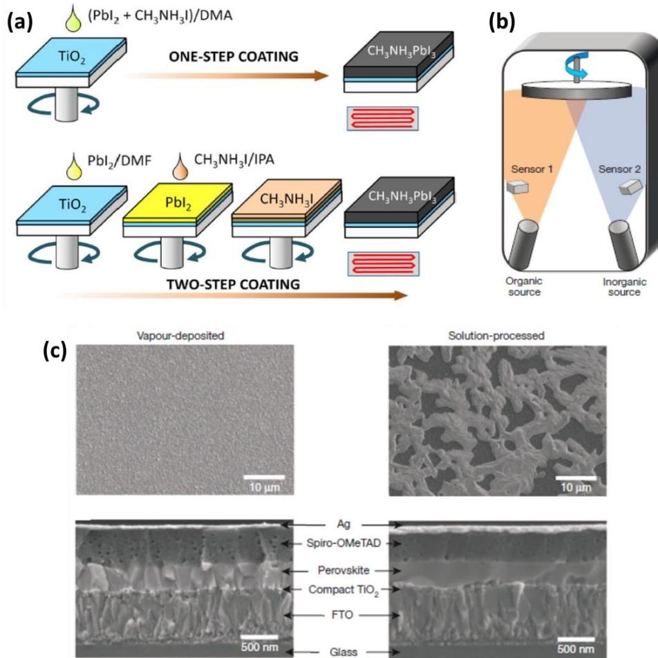
**Figure 7:** (a) One-step and two-step spin-coating procedures for  $\text{CH}_3\text{CH}_3\text{PbI}_3$  formation. Figure adapted from ref<sup>66</sup>. (b) Dual-source thermal evaporation system for depositing the perovskite absorber. Figure adapted from ref<sup>24</sup>. (c) SEM top viewed (top) and cross-sectional viewed (bottom) of complete solar cells constructed by vapor-deposited and solution-processed methods. Figure adapted from ref<sup>24</sup>.
