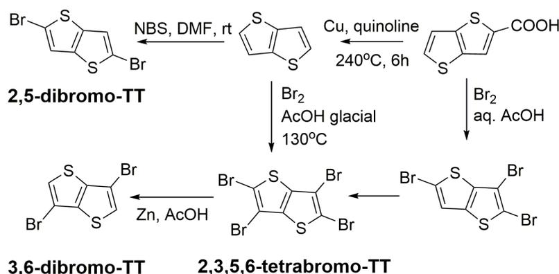
*Scheme 2: Synthetic route of thieno[3,2-*b*]thiophene ring systems. Figure adapted from reference<sup>33</sup>*
