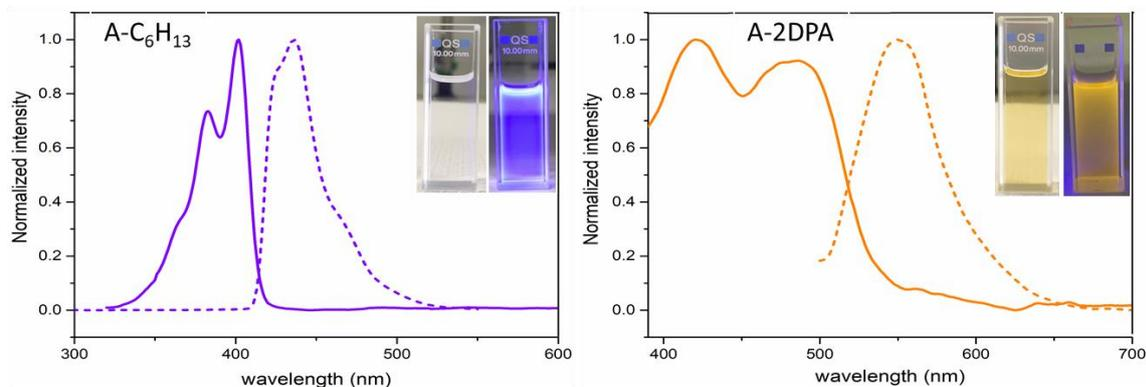
**Figure 9 :** Absorption (solid line) and emission (dashed line) spectra of A-C<sub>6</sub>H<sub>13</sub> and A-2DPA measured in diluted DCM. Inset: photographs of these solutions under daylight and UV 365 nm.
