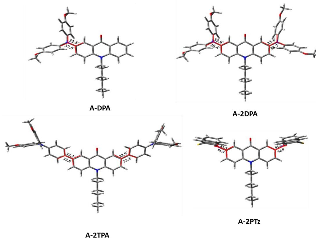
*Figure 7 : Optimized structures along with the dihedral angles (°) of all compounds simulated by B3LYP/6-31G(d) in dichloromethane*
