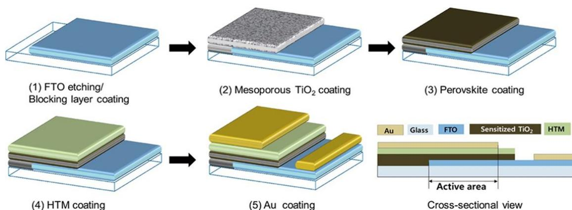
**Figure 19** : Procedure to fabrication of typical mesoscopic perovskite solar cells.
