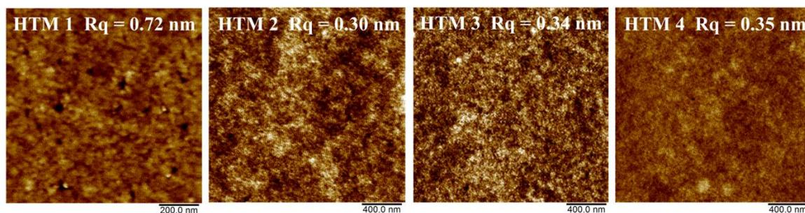
**Figure 10: AFM images of these compounds coated on glass substrates.**
