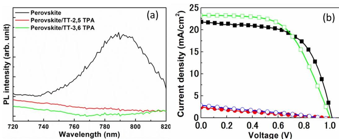
**Figure 14:** (a) Photoluminescence spectra for different materials as films on glass and (b)  $J$ - $V$  characteristics in the forward (filled symbols) or reverse bias (empty symbols) directions of PSCs utilizing TT-2,5 TPA (rectangles) or TT-3,6 TPA (circles) HTMs.
