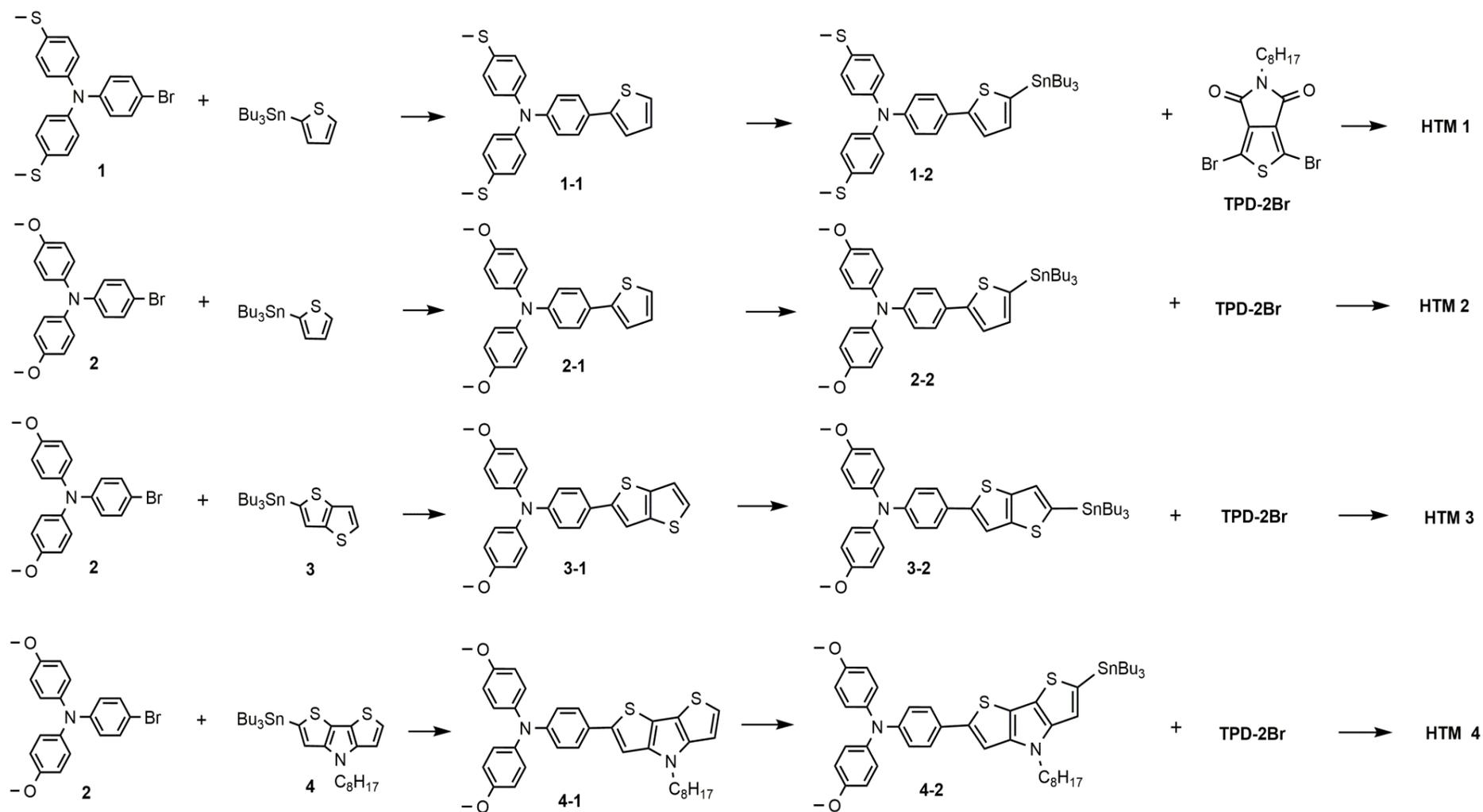
**Scheme 3: Synthetic route of TPD-based planar structure molecules. Conditions and reagents: Stille coupling reaction:  $\text{Pd}(\text{PPh}_3)_4$ , Toluene,  $110^\circ\text{C}$ , 24h and Lithium-bromine exchange reaction:  $n\text{-BuLi}$ , THF,  $-78^\circ\text{C}$ ,  $\text{Cl-SnBu}_3$ , 8h.**
