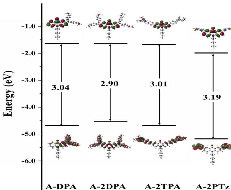
Figure 11 : Frontier molecular energy diagram of all molecular structures
