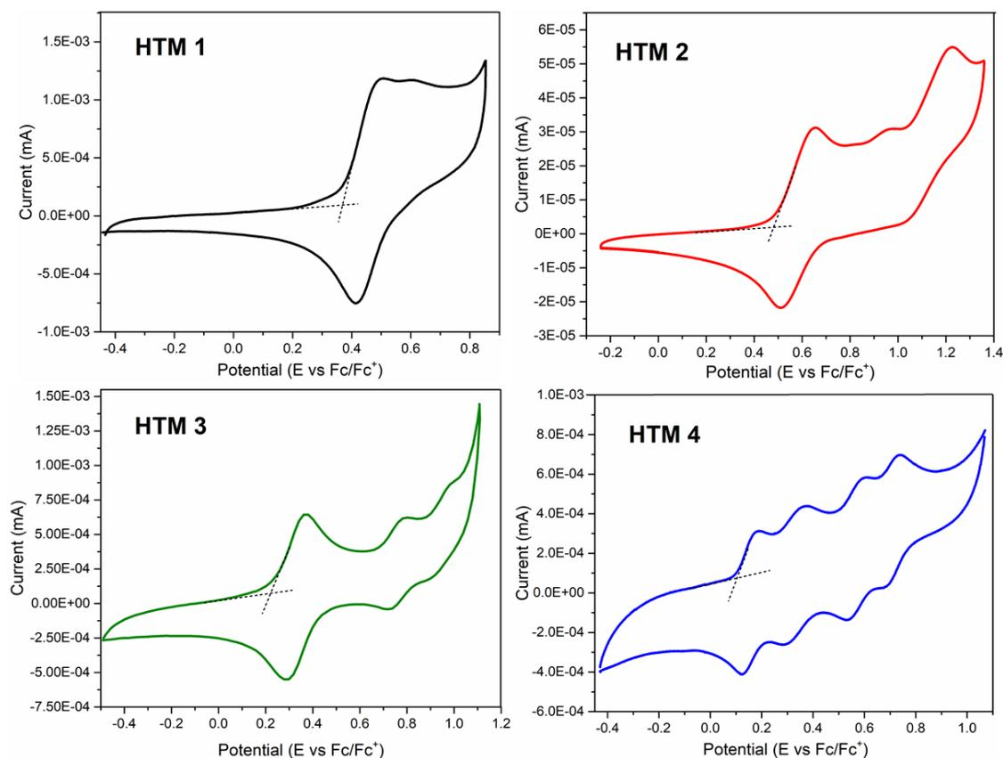
Figure 8: Cyclic voltammograms of studied molecules-based TPD measured in 0.1 M  $(n\text{-Bu})_4\text{N}^+\text{PF}_6^-$  electrolyte solution at scan rate 50 mV/s (the  $\text{Fc}/\text{Fc}^+$  redox couple is used as internal standard).
