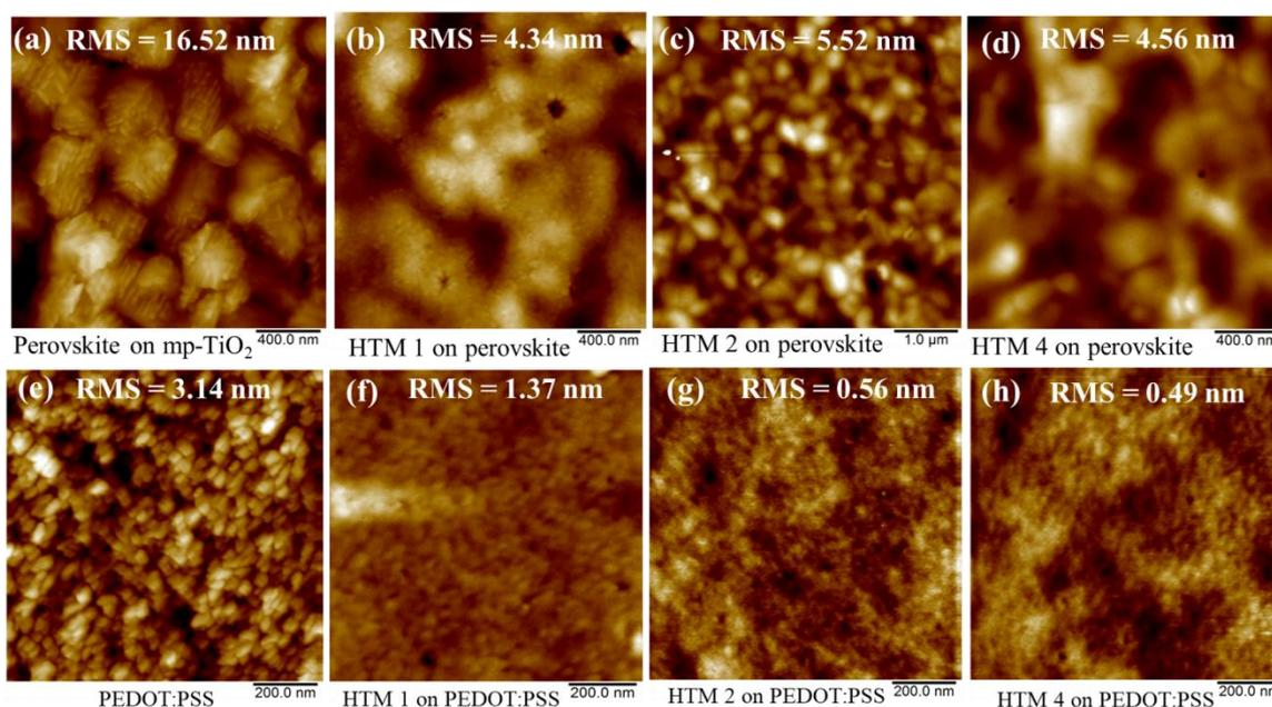
**Figure 11: AFM images of  $\text{MAPbI}_3$  on  $\text{TiO}_2$  (a), HTM 1 on  $\text{MAPbI}_3$  (b), HTM 2 on  $\text{MAPbI}_3$  (c), HTM 4 on  $\text{MAPbI}_3$  (d), PEDOT:PSS on ITO (e), HTM 1 on PEDOT:PSS (f), HTM 2 on PEDOT:PSS (g) and HTM 4 on PEDOT:PSS (h).**
