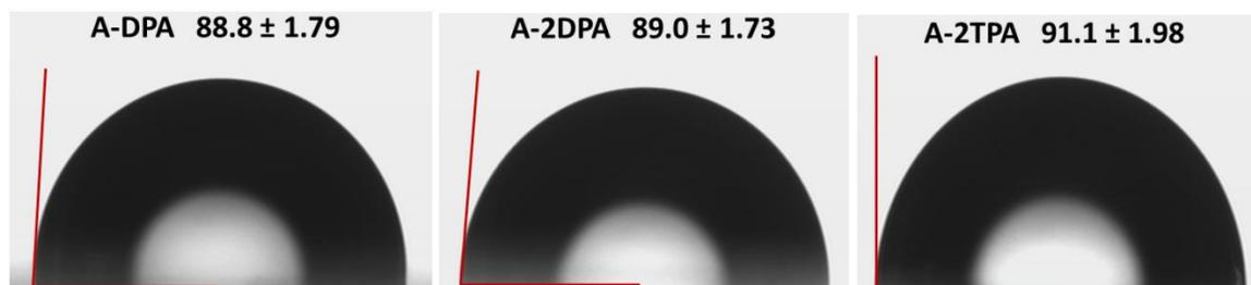
**Figure 18** : Contact angle measurement (°) of A-DPA, A-2DPA and A-2TPA films coated on glass substrate.
