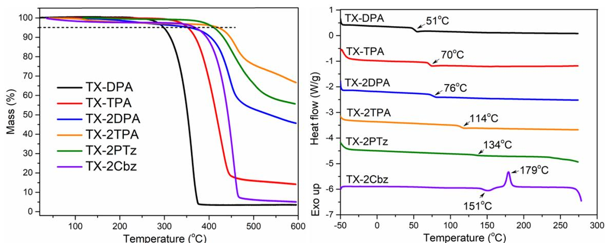
**Figure 24:** TGA (left) and DSC (right) curves of studied Thioxanthone molecules. Glass transition temperature  $T_g$  is obtained from the onset values of DSC and decomposition temperature  $T_d$  is recorded by 5% weight loss in TGA.
