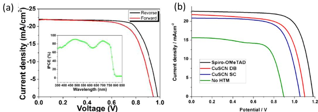
**Figure 10:** (a) Forward-reverse bias current density–voltage characteristics of the HTM-free PSCs and IPCE spectrum (inset). Figure adapter from ref<sup>83</sup>. (b) *J–V* curves of mixed perovskite solar cells based on CuSCN, spiro-OMeTAD, and no hole-transporting materials. Figure adapted from ref<sup>84</sup>.
