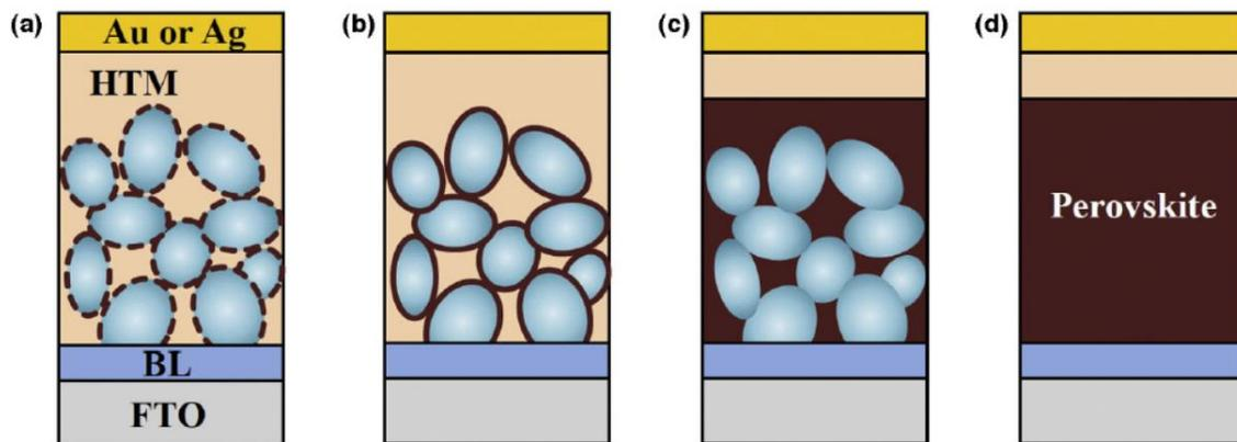
**Figure 4: Structural evolution of perovskite solar cells. (a) Sensitization concept with surface absorption of nanodot perovskite, (b) PSCs with non-injecting Al<sub>2</sub>O<sub>3</sub> scaffold layer, (c) pillared structure PSCs and (d) planar *p-i-n* heterojunction concept. Figure adapted from ref<sup>44</sup>.**
