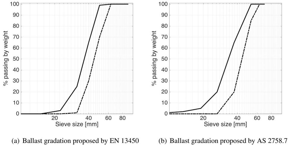
FIGURE 1.2: Ballast gradation proposed for railway ballast. The solid line represents the maximum limit, and the dashed line the minimum limit.
