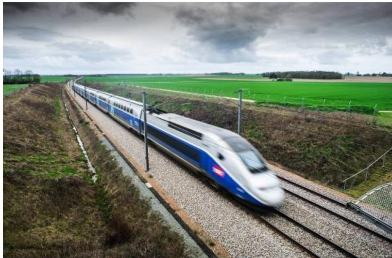
(a) French high-speed train in a ballasted railway track [248]
