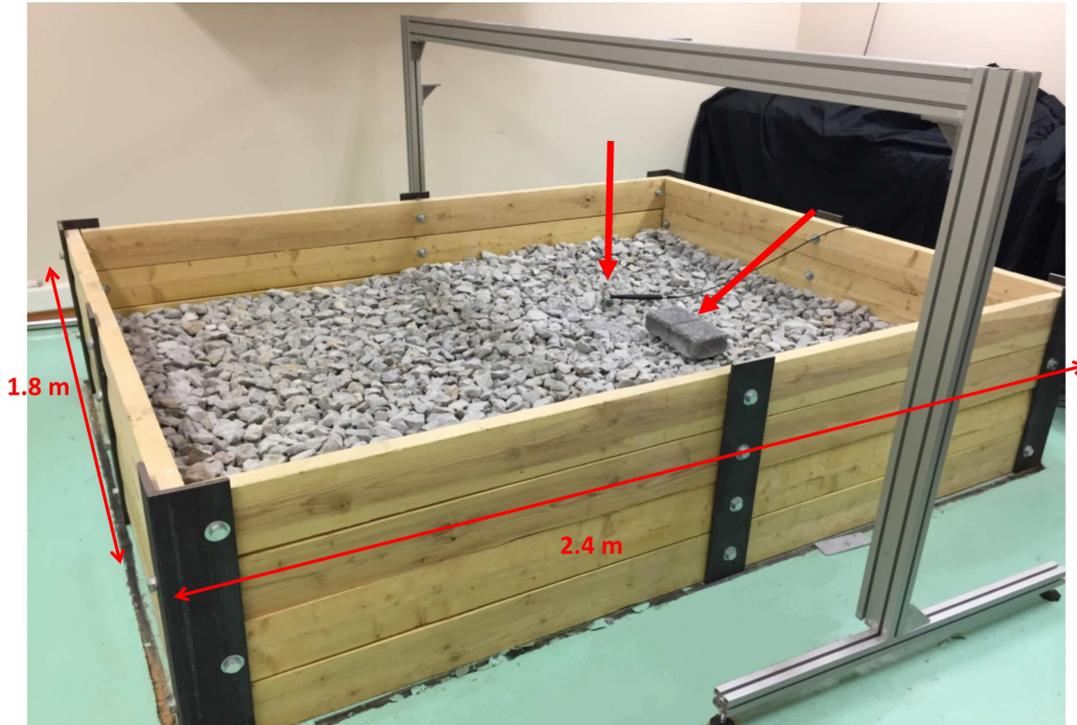
FIGURE 4.1: Experimental setup. Wooden box filled with ballast grains with  $1.8 \times 2.4 \text{ m}^2$  and variable thickness. Concrete block, placed at source position 1, (see Fig. 4.2), and impact hammer used in the tests are indicated by the red arrows.
