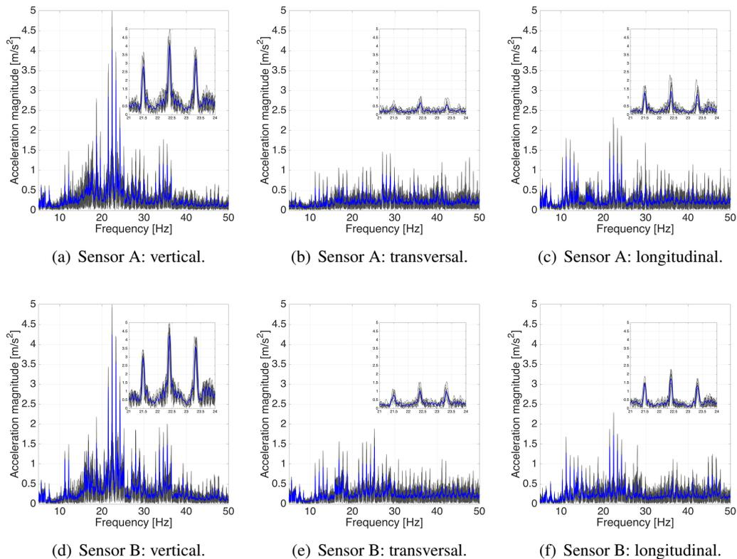
FIGURE 4.26: Acceleration spectrum magnitude of 9 trains passages, gray line, the blue line represents the mean between the values. The upper line corresponds to the vertical, transversal, and longitudinal accelerations for the sensor A. The second line shows the same quantities for the accelerometer B.
