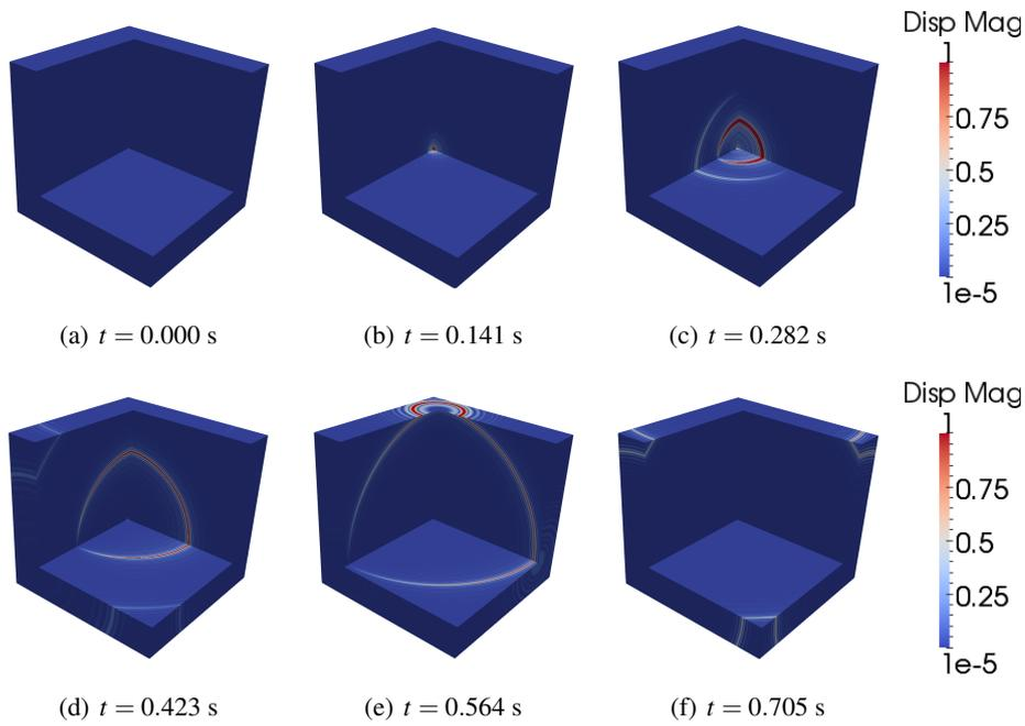
FIGURE 3.6: Displacement fields in an unbounded homogeneous model. The color scale represents the normalized magnitude of the displacement field, the color scale goes from  $1 \times 10^{-5}$  (blue color) up to 1 (red color).
