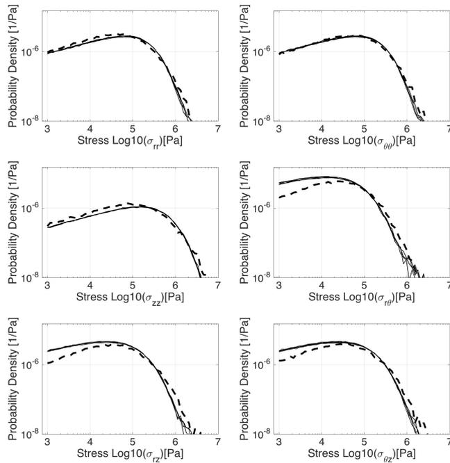
FIGURE 2.11: Distribution of the logarithm of the equivalent stresses for the discrete samples and averaging volume  $V = (4 \text{ cm})^3$  (dashed line), and for the identified continuum model with Gamma first-order marginal density (solid line).
