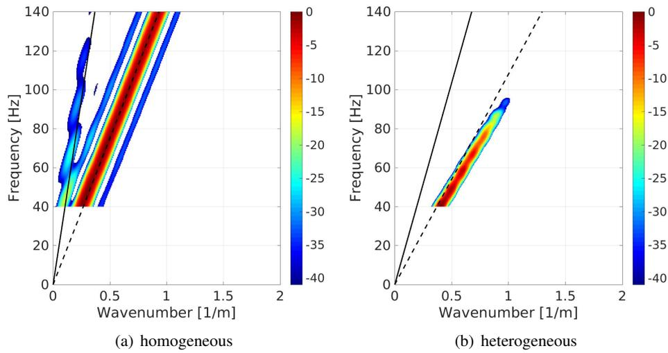
FIGURE 3.16: Dispersion curves for unbounded homogeneous and heterogeneous media. The color scale is the amplitude of  $H_{pq}$  evaluated in Eq. (3.10), limited to values above  $-40$  dB. The dotted black line is the analytical solution for the homogenized pressure waves dispersion relation. The dashed black line is the analytical solution for the homogenized shear wave.
