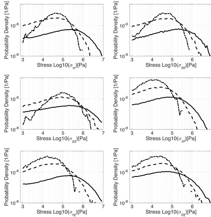
FIGURE 2.4: Probability distribution functions of the different components of the equivalent stress  $\sigma^V$ , as a function of the averaging volume:  $V = (2 \text{ cm})^3$  (solid line),  $V = (4 \text{ cm})^3$  (dashed line) and  $V = (8 \text{ cm})^3$  (dash-dotted line).
