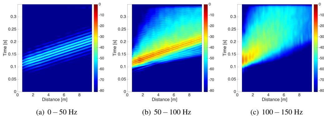
FIGURE 3.18: Displacement magnitude in an unbounded heterogeneous medium. The color scale is the amplitude of the displacement field, limited to values above  $-80$  dB.
