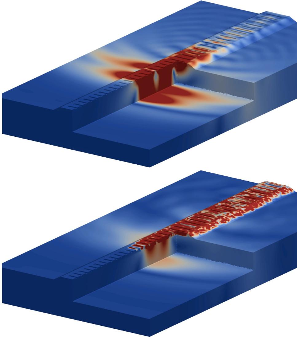
FIGURE 3.2: Displacement fields at time  $t = 0.27$  s. The upper figure corresponds to the simulation with homogeneous ballast, while the lower one corresponds to simulation with heterogeneous ballast.
