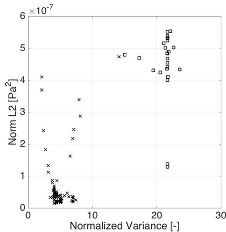
FIGURE 2.16: Evolution of the  $L^2$  distance during the optimization process at  $V = (4 \text{ cm})^3$  as a function of the normalized variance  $\sigma_E^2/E^2$ . The crosses represents the realizations where the departure point, for the optimization process, were below 10,  $\sigma_E^2/E^2 \leq 10$ . The squares represent the realization where the departure point was greater than 10,  $\sigma_E^2/E^2 \geq 10$ .
