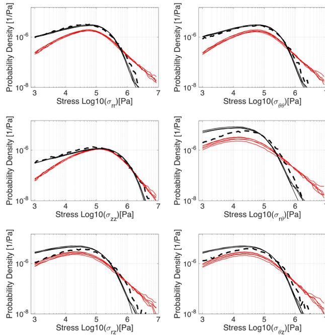
FIGURE 2.15: Distribution of the logarithm of the equivalent stresses for the discrete samples and averaging volume  $V = (4 \text{ cm})^3$  (black dashed line), for the identified continuum model with Gamma first-order marginal density (black solid line), and for the identified continuum model with Log-normal first-order marginal density (red solid line).
