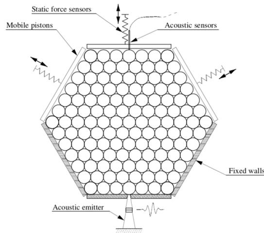
FIGURE 1.7: Experimental setup for the isotropic confinement stress, extracted from Gilles and Coste [96].
