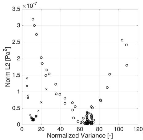
FIGURE 2.14: Evolution of the  $L^2$  distance during the optimization process at  $V = (4 \text{ cm})^3$  as a function of the normalized variance  $\sigma_E^2/\underline{E}^2$ , for a Gamma (crosses) and log-normal (circles) first-order marginal distribution.
