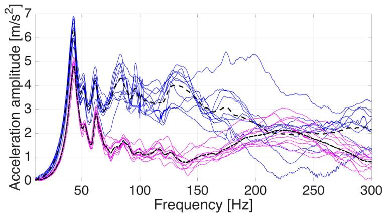
FIGURE 4.5: Acceleration amplitude vs. frequency, each solid line represents one experiment. The blue lines represent the set S1d10h25, with the black dashed lines as the average. The solid magenta lines represent set S1d25h25, with the black dash-dotted line as the average.
