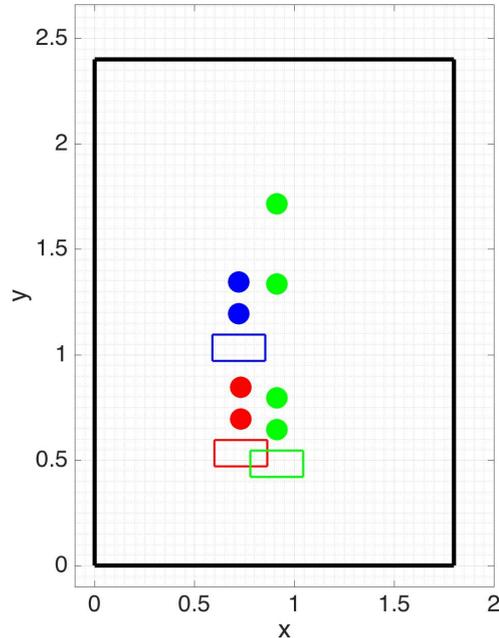
FIGURE 4.2: Schematic representation of the position of the sources and accelerometers in the  $x - y$  plane. The red rectangle represents the position of the concrete block for all the sets with source position 1 (S1), the green and blue one represent the same information for source positions 2 (S2) and 3 (S3), respectively. The filled circles are the positions of the accelerometers, the red ones for the set S1, the green ones for S2 and blue ones for S3.
