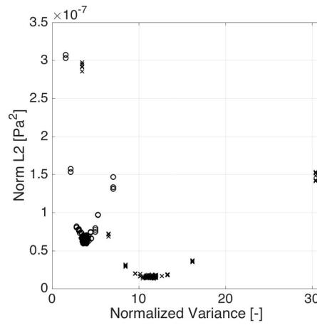
FIGURE 2.12: Evolution of the  $L^2$  distance during the optimization process for a Gamma first-order marginal distribution and different averaging volumes:  $V = (4 \text{ cm})^3$  (crosses), and  $V = (8 \text{ cm})^3$  (circles), as a function of the normalized variance  $\sigma_E^2/\underline{E}^2$ .
