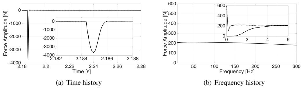
FIGURE 4.3: Force recorded by the impact hammer for the 5th trial of sets S1d10h25 and S1d25h25. Fig. 4.3(a) presents the time history recorded in the impact hammer, Fig. 4.3(b) presents the amplitude of the FFT of the time signal. The solid line is the filtered signal and the dashed line is the non filtered signal.
