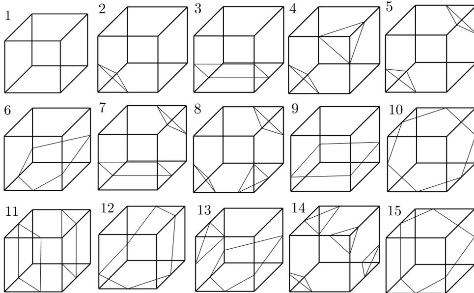
FIGURE A.4: Intersection of the cut surface in the hexahedra element, extracted from Kudela *et al.* [133]).
