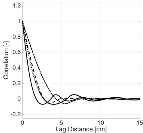
FIGURE 2.5: Correlation function for an impenetrable sphere packing with constant diameter  $\underline{d}$  and volume ratio  $\underline{\phi}$ . Four cases were presented here:  $\underline{d} = 3.9$  cm and  $\underline{\phi} = 0.5682$  (solid line);  $\underline{d} = 3.9$  cm and  $\underline{\phi} = 0.2$  (dashed line);  $\underline{d} = 6$  cm and  $\underline{\phi} = 0.5682$  (dotted line);  $\underline{d} = 6$  cm and  $\underline{\phi} = 0.2$  (dash-dotted line).
