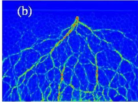
FIGURE 1.3: Photoelastic experiment in granular medium subjected to a point load and gravity, extracted from Geng *et al.* [91]. The color scale represent the amplitude of the load from high loads (red) to lower loads (blue).
