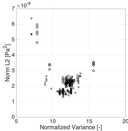
FIGURE 2.18: Evolution of the  $L^2$  distance during the optimization process for a Gamma first-order marginal distribution at  $V = (4 \text{ cm})^3$  and  $\underline{E} = 80 \text{ MPa}$  (crosses), and for  $V = (4 \text{ cm})^3$  and  $\underline{E} = 800 \text{ MPa}$  (circles), as a function of the normalized variance  $\sigma_E^2/\underline{E}^2$ .
