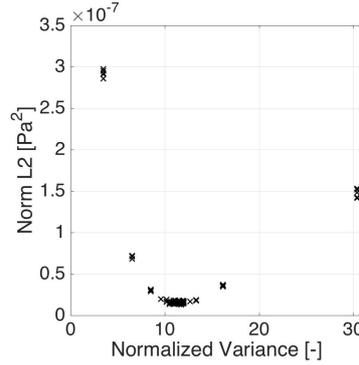
FIGURE 2.10: Evolution of the  $L^2$  distance during the optimization process for a Gamma first-order marginal distribution and averaging volume  $V = (4 \text{ cm})^3$  as a function of the normalized variance  $\sigma_E^2/\underline{E}^2$ .
