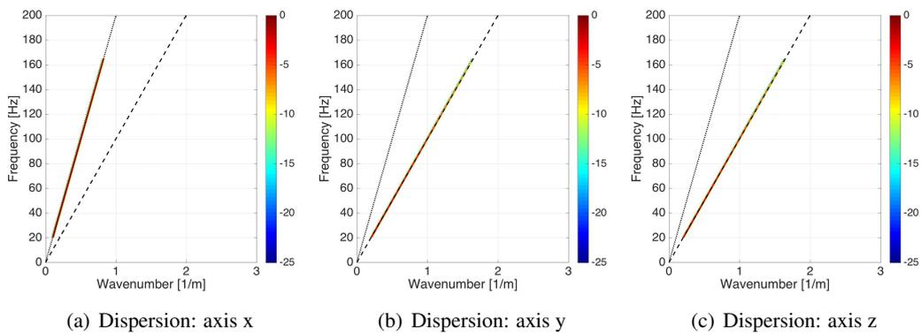
FIGURE 3.7: Dispersion curves for an unbounded homogeneous media. The color scale is the amplitude of  $H_{pq}$  evaluated in Eq. (3.10), limited to values above  $-25$  dB. The dotted black line is the analytical solution for the pressure waves dispersion relation. The dashed black line is the analytical solution for the shear wave.
