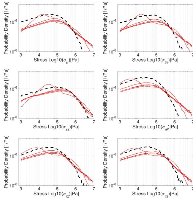
FIGURE 2.17: Distribution of the logarithm of the equivalent stresses for the discrete samples and averaging volume  $V = (4 \text{ cm})^3$  (black dashed line), for the identified continuum models with Gamma first-order marginal density and cardinal sine correlation model (red solid lines).
