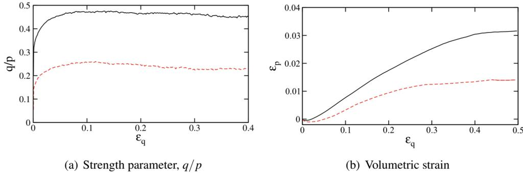
FIGURE 1.10: Complex behavior of granular media as a function of shear strain  $\epsilon_q$ , with irregular ballast grains (black line) and spheres (red line) under quasistatic shearing, extracted from Azéma *et al.* [25].
