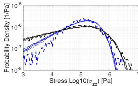
FIGURE 2.13: Distribution of the logarithm of the vertical equivalent stresses,  $\sigma_{zz}$  for the discrete samples (dashed lines) and for the identified continuum models with Gamma first-order marginal density (solid lines), for averaging volumes  $V = (4 \text{ cm})^3$  (black lines) and  $V = (8 \text{ cm})^3$  (blue lines).
