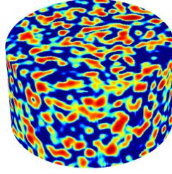
FIGURE 2.7: One realization of the random model of Young's modulus ( $\underline{d} = 3.9$  cm and  $\underline{\phi} = 0.5830$ ) for a cylinder of the same size as in Fig. 2.1: radius  $R = 35$  cm and height  $H = 39$  cm.
