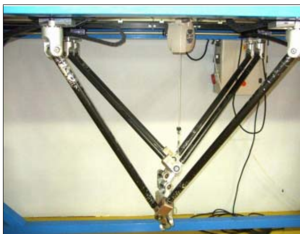
Fig. 1-48: \lambda -Quadriglide-V1 (ANCUTA, 2008): schematic, graph diagram and prototype photo.
