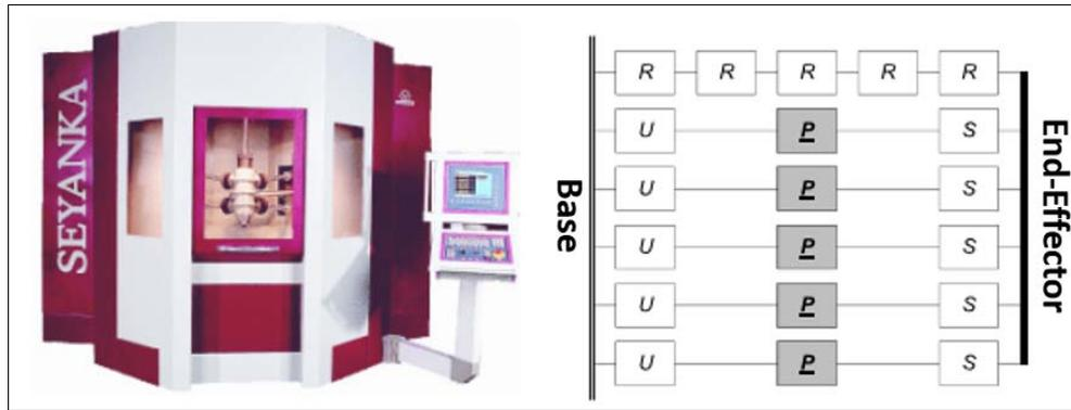
Fig. 1-23: Seyanka (Tekniker): photo and graph diagram.
