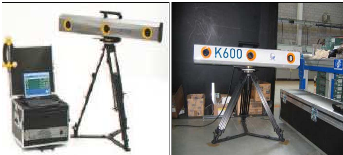
Fig. Ap-4: Metris K600 CMM measuring device.
