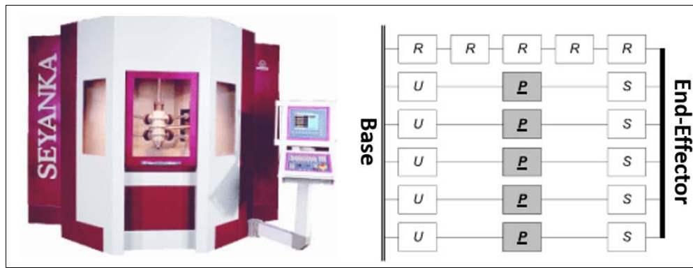
Fig. 1-23: Seyanka (Tekniker): photo and graph diagram.
