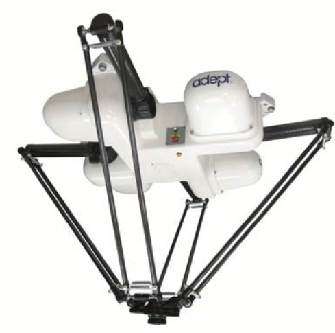
Fig. 1-45: Industrialized version of Par4 (Adept Quattro).
