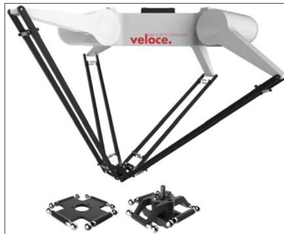
Fig. 1-47: Veloce (Penta Robotics): photo and platforms (on the left corresponds to the case of three dofs (3T), and on the right corresponds to the case of four dofs (3T-1R)).
