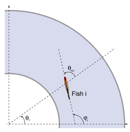
Figure 4.6: Variables used to describe the position, heading and relative orientation of fish relative to the wall in the experimental set-up:  $\theta_i$  is the angle formed by the position vector of fish i and the horizontal line,  $\varphi_i$  is the heading of fish i, and  $\theta_{wi}$  is the angle of incidence of fish i relative to the wall w.
