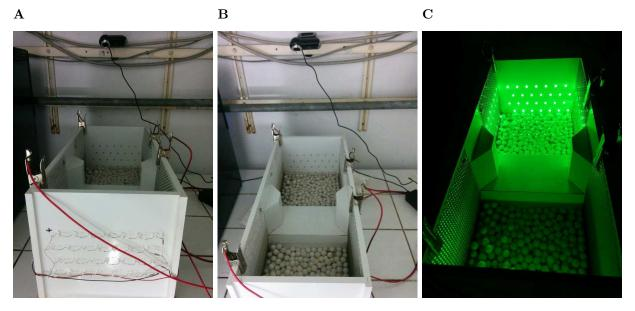
Figure 5.1: Pictures of the shuttle box  $(46 \times 23 \times 21 \text{ cm})$  used for the aversive conditioning. In (C), the conditioned stimulus is turned on in one of the two compartments.
