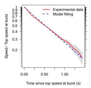
Figure 3.6: Decay of speed during coasting phases relative to top speed in experimental data (red curve) and as modelled by a drag due to water frictions with exponential decay of parameter  $D \approx 0.71$  (blue). The grey shade shows the bootstrapped 95% confidence interval.
