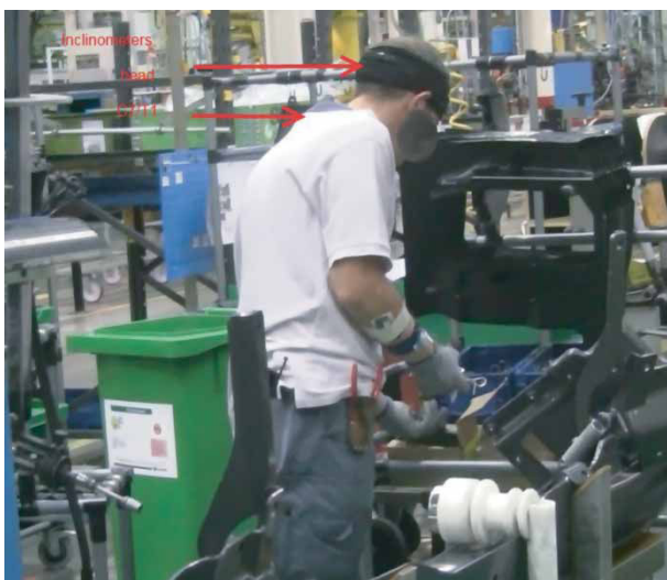
Figure 3. Operator in the working position with two inclinometers placed behind the head and adhered to C7/T1. This figure shows the difficulty of the observer in assessing movement of the head.
