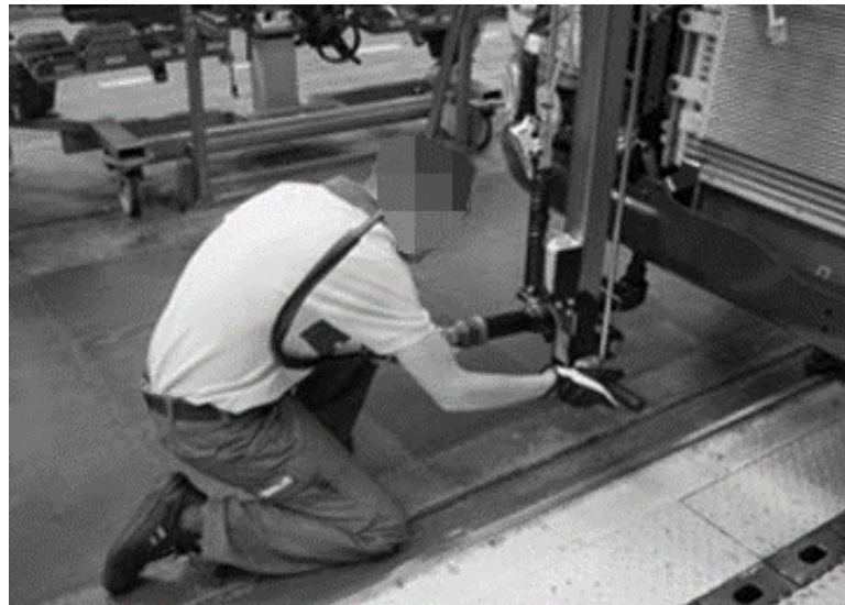
Figure 2: Tightening screws at 'Mounting bumper on chassis' workstation caused awkward trunk and neck postures
