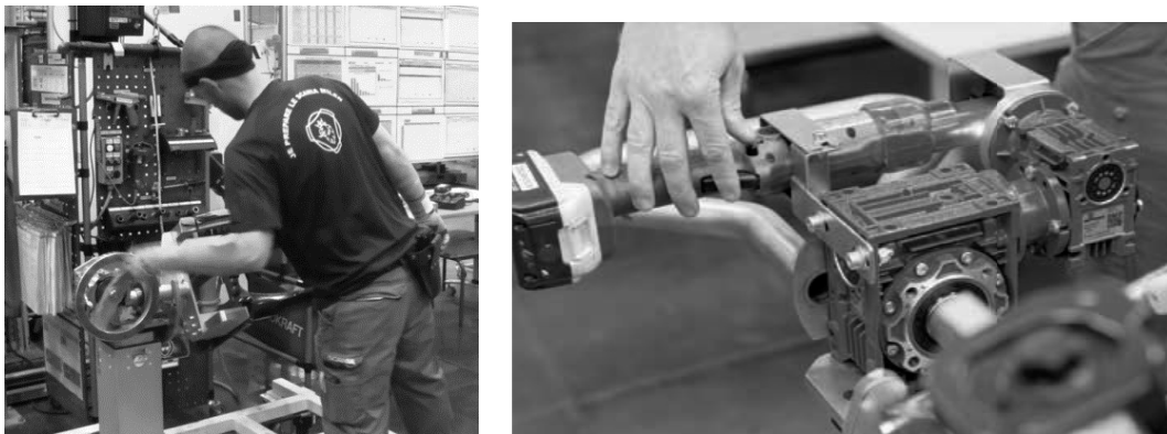
Figure 6a: Manually turning the SCR wagon handle (intensive repeated action) b) A screwdriver replaced the manual turning handle which eliminated repeated actions
