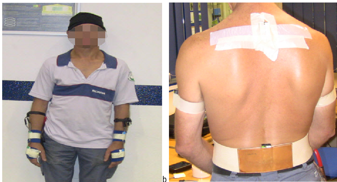
Figure 1: Localization of seven sensors used to measure the body segment postures; (a) two goniometers on the right/left wrists and one inclinometer on the head (occipital bone); (b) two accelerometers on the right/left arms in the middle of humerus, one accelerometer on the lower back (L3) and one inclinometer on the upper back at C7-T1.
