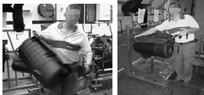
Figure 3: Lifting and carrying air filter (12-16 kg) caused low back pain and awkward posture Gripping tool for handling air filter
