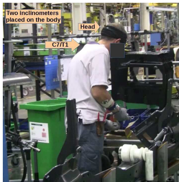
Figure 3: Operator in the workstation with two inclinometers placed at the behind of the head and adhered to C7/T1. This picture shows the difficulty of the observer to assess the movements of head from just one viewpoint as it is constrained by the actual work situation inappropriate for evaluating head bending
