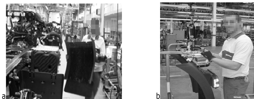
Figure 5a: Lifting and carrying of rear mudguards (15kg) manually, major risk factor for low back pain; b) new lifting tool used for lifting and carrying mudguards
