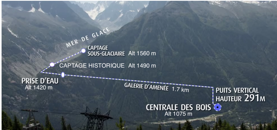
Figure I.9: Scheme of the Waterpower Development under the Mer de Glace-Leschaux glacier. Figure based on an image taken from EDF, 2016 .
