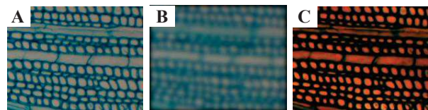
Figure 3. Difference of Gaussian filtering on a cross-section of Mahogany stained with toluidine blue. A: the image obtained by applying a small Gaussian blurring ( \sigma = 3 pixels). B: the image resulting from a strong Gaussian blurring ( \sigma = (\text{image width})/10 ). C: subtraction of images A and B which increases the contrast wall / lumen.
