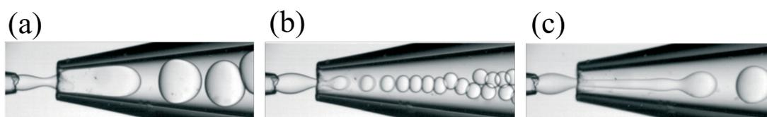
**Fig. 2.2** Example of different droplet breakup modes for a flow-focusing production junction: (a) Squeezing, (b) Dripping (c) Jetting. Reprinted from Zhu *et al.* [18].
