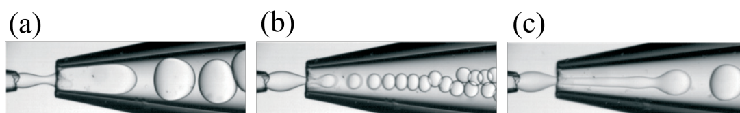
Fig. 2.2 Example of different droplet breakup modes for a flow-focusing production junction: (a) Squeezing, (b) Dripping (c) Jetting. Reprinted from Zhu et al. [18].
