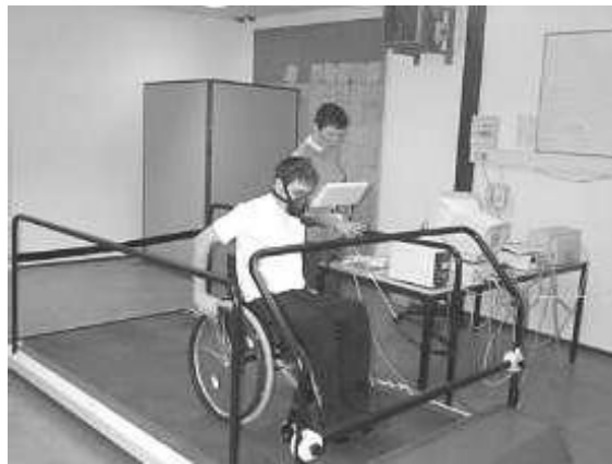
Figure A.3: Exercise testing on a motor driven treadmill [Van der Woude et al., 2006]
