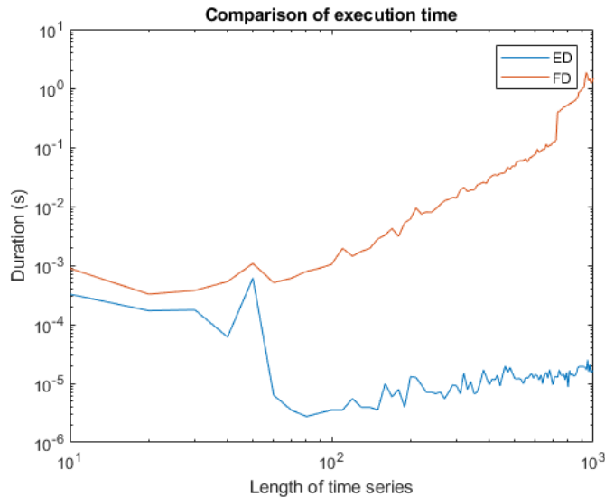
Figure 3.6: The execution time of ED and FOTS score is a function of the length of time series. The computation time of ED is smaller than that of FOTS.
