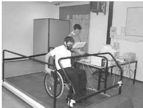
Figure A.3: Exercise testing on a motor driven treadmill [Van der Woude et al., 2006]
