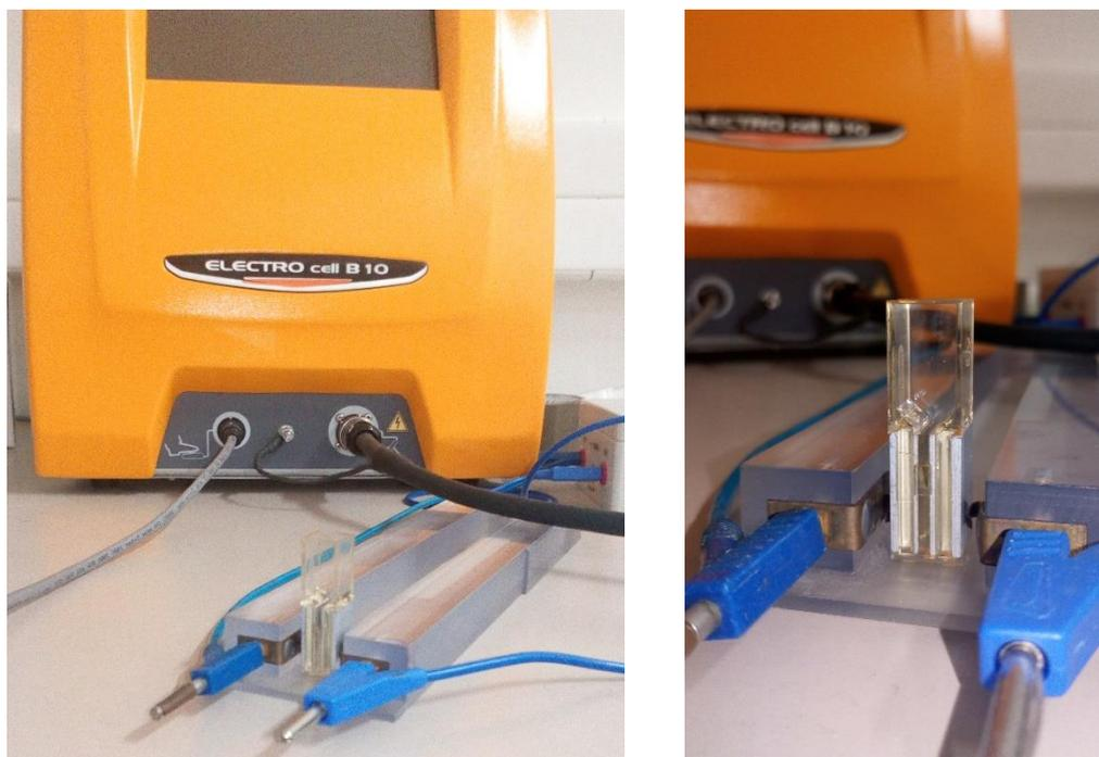
**Figure 13:** Experimental setup for the PEF treatment. The left image shows the pulse generator and the cuvette holder containing the cuvette and the right image focuses on the electroporation cuvette (1mm electrode gap).
