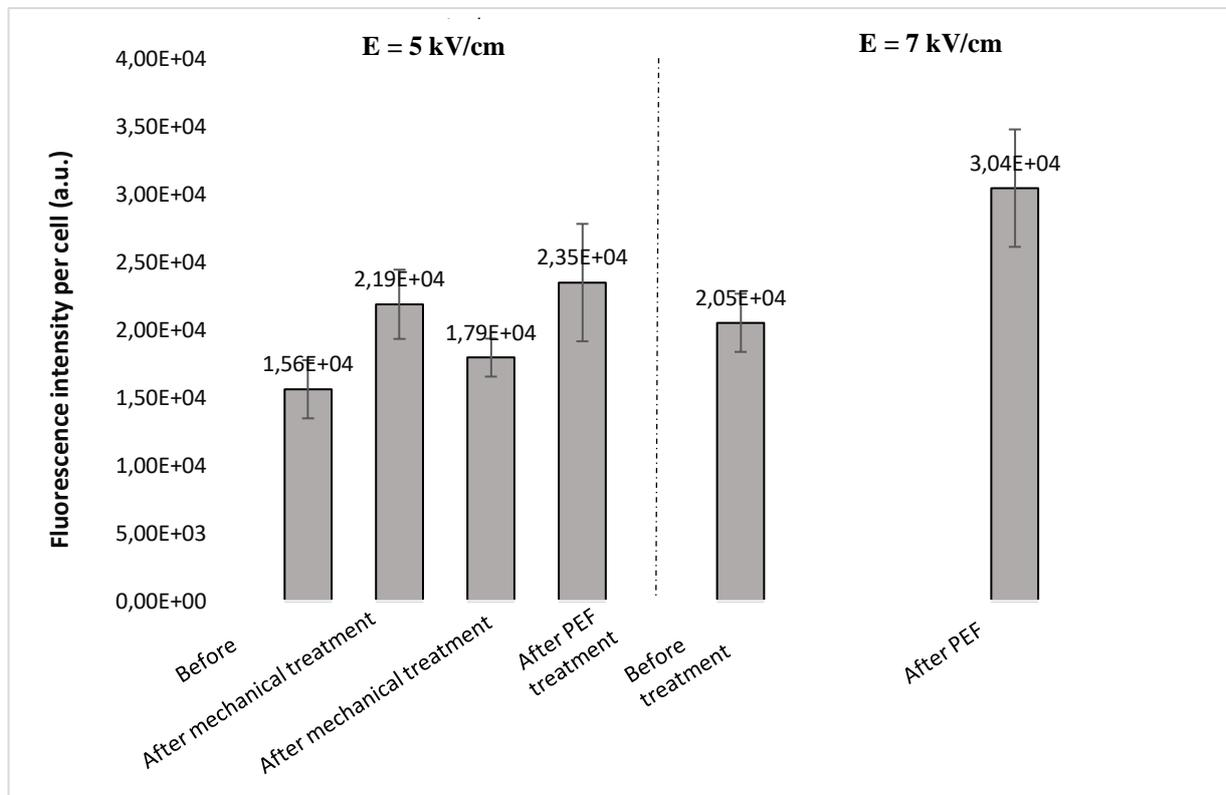
**Figure 10** Representative cytometric results of the fluorescence intensity emitted by Bodipy 505/515 after the different conditions of treatments. (The cell suspensions were stained with bodipy after each treatment). Electroporation conditions: 10 unipolar pulses of 5  $\mu\text{s}$  each, 10 Hz, 5,5 kV/cm for the left side of the graph and 7kV/cm for the right side of the graph.
