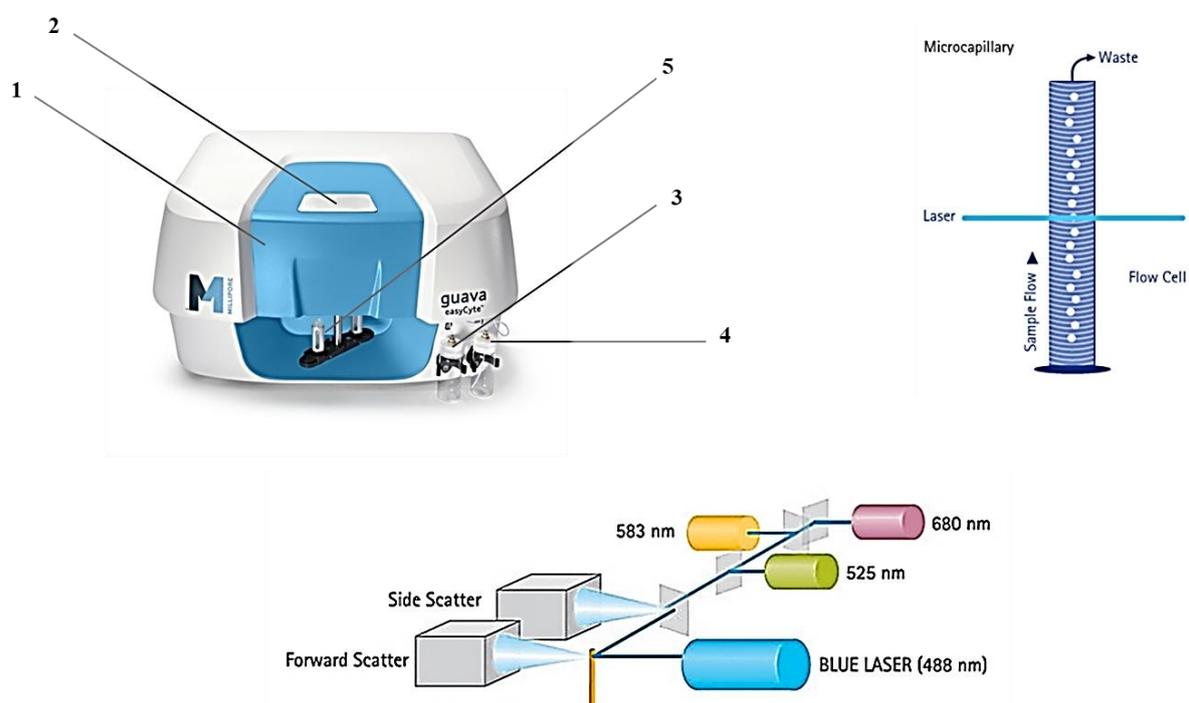
**Figure 2: Flow cytometer used during our experiments for the analysis of cell concentration, viability and permeability. 1: detection zone (up to 12 parameters); 2: Microcapillary flow cell (shown also on the upper right); 3: waste vial; 4: cleaning solution vial; 5: sample loader. On the bottom of the figure: the blue laser trajectory through the forward and side scatter and the 3 fluorescence detector channels (Source: Guava InCyte manual).**
