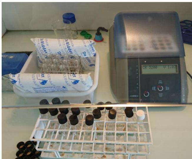
Figure 18: Tube heater (WTW CR3200) and ice cooling
