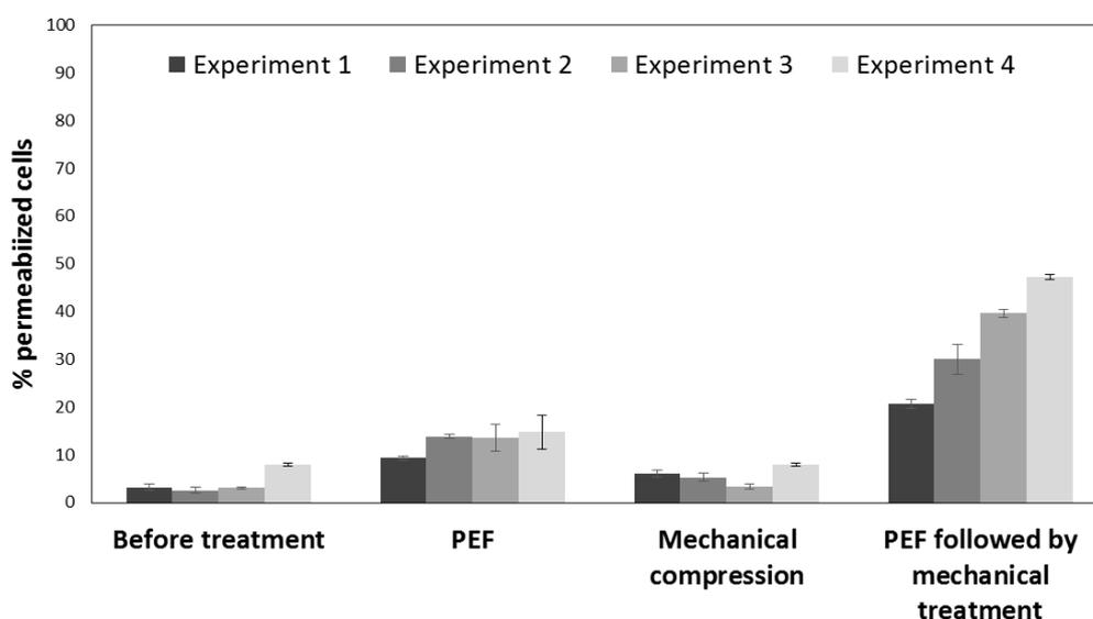
**Fig. 3** Percentage of permeabilized cells (Sytox Green uptake) before and after being submitted to the following pretreatments: Pulsed electric field treatment, mechanical compression and a combination of both pretreatments. Results were analyzed by flow cytometry. Data show four independent experiments performed on four different algae cultures. Error bars represent the standard deviation of triplicate samples.
