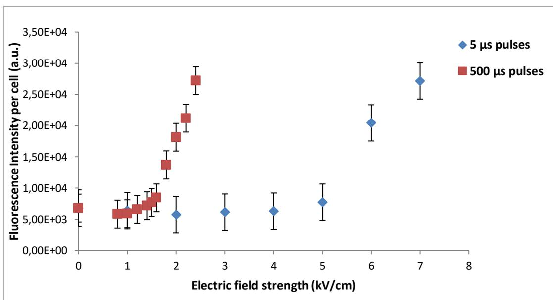
**Figure 11** Evolution of the fluorescence intensity emitted by Bodipy with the electric field strength applied for two pulse durations. The experiment was held on *C. reinhardtii* wild type after being stressed for 7 days.
