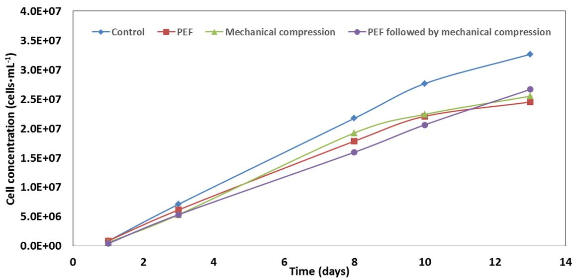
**Fig. 4** *Chlamydomonas reinhardtii*'s growth after different pretreatments: Pulsed electric field, mechanical compression and a combination of both pretreatments. The control corresponds to cell that have only been submitted to 7 days of stress and weren't submitted to any pretreatment.
