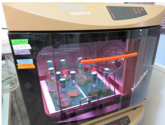
**Figure 1: Shake incubator used for the growth cultivation step.**
