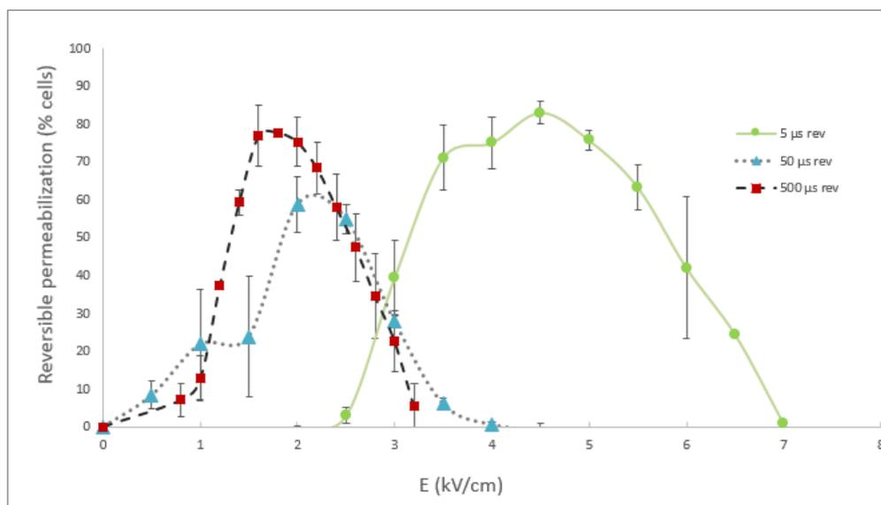
Figure 2: Impact of the electric field on the reversible permeabilization (RP cells) obtained using 5, 50 and 500  $\mu\text{s}$  pulses respectively (burst 10 square pulses with 10 Hz frequency). Experiments were performed on *Chlamydomonas reinhardtii* cells at 7 days of stress. Error bars corresponds to standard deviation (SD). Means and associated SD are obtained from two independent assays.
