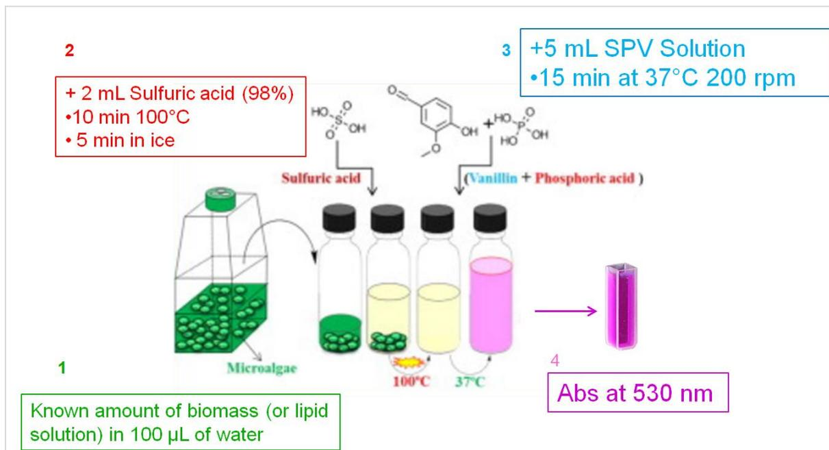
Figure 17: Principle of the method (Mishra *et al.*, 2014)
