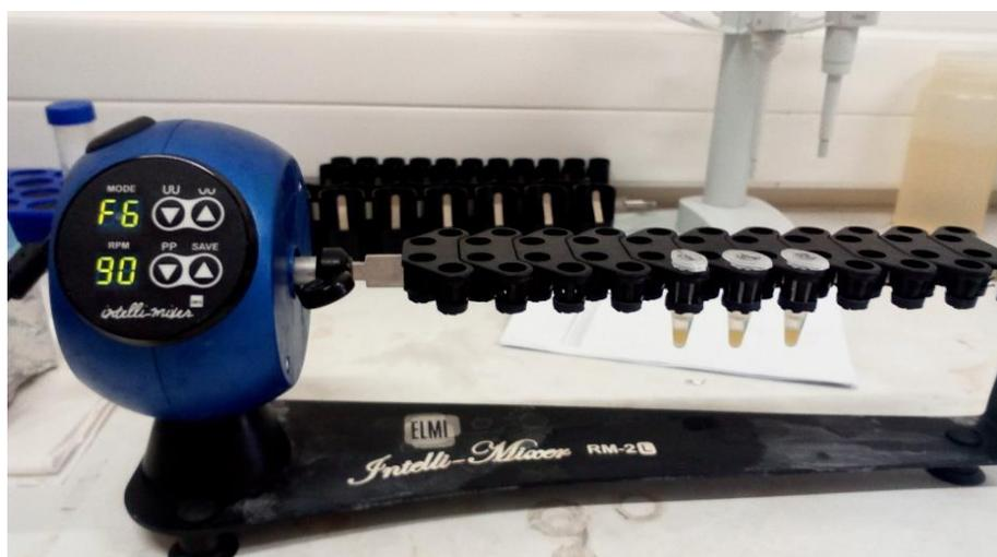
Figure 14: Agitating system used for the lipid extraction using solvents.
