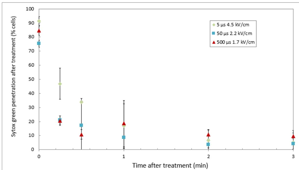
Figure 7: Sytox green penetration after reversible pulse treatment conditions measured from 0 to 3 minutes at 20°C. Experiments were performed on *Chlamydomonas reinhardtii* cells at 7 days of stress. Error bars corresponds to standard deviation (SD). Means and associated SD are obtained from two independent assays.
