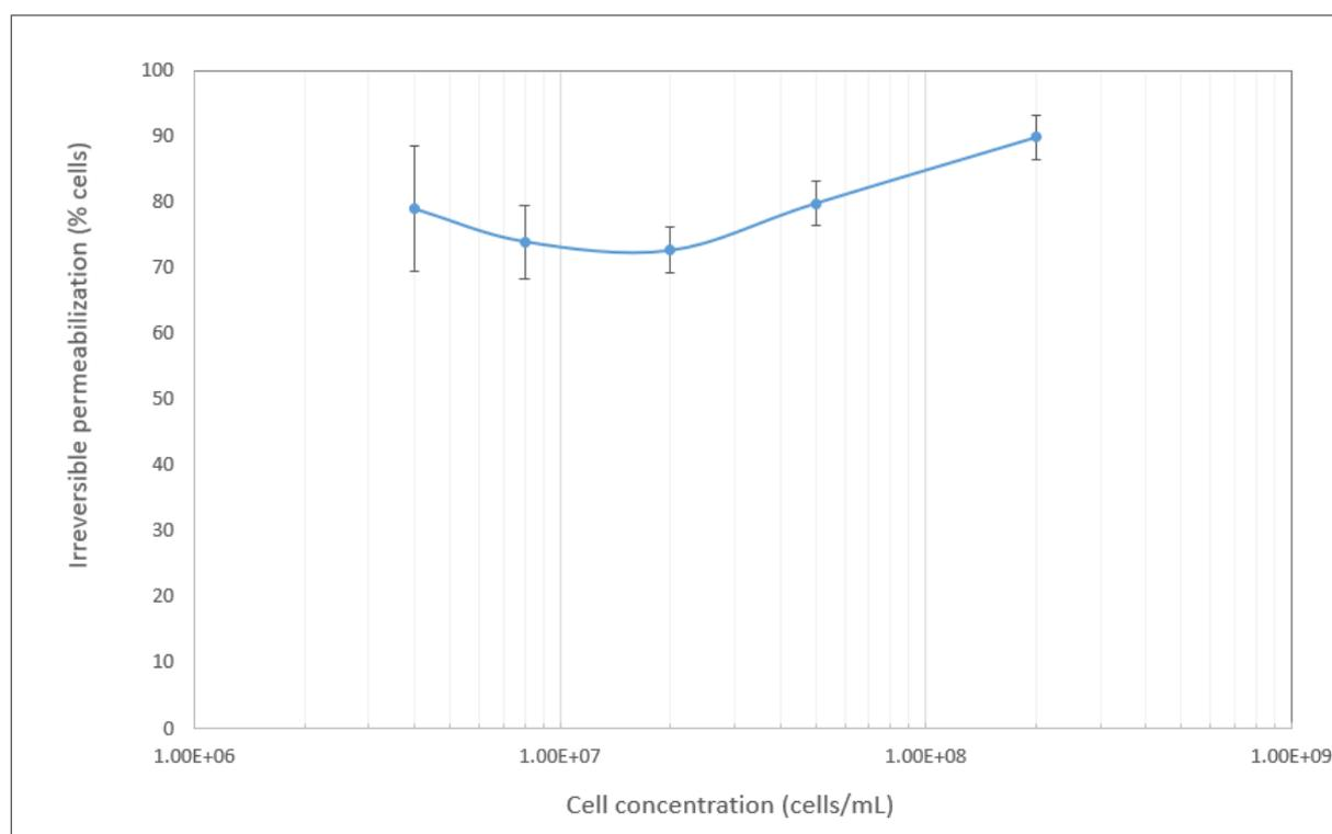
Figure 4: Effect of the cell concentration (from 4·10<sup>6</sup> to 2·10<sup>8</sup> cells·mL<sup>-1</sup>) on the irreversible permeabilization (IP cells) obtained after a treatment of 10 pulses of 5 µs and 7 kV/cm. Experiments were performed on *Chlamydomonas reinhardtii* cells at 7 days of stress. Error bars corresponds to standard deviation (SD). Means and associated SD are obtained from two independent assays.
