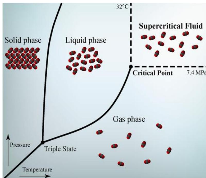
Figure 44: Phase diagram. CO<sub>2</sub> Critical point: 32°C, 7.4 MPa (Capuzzo et al., 2013).
