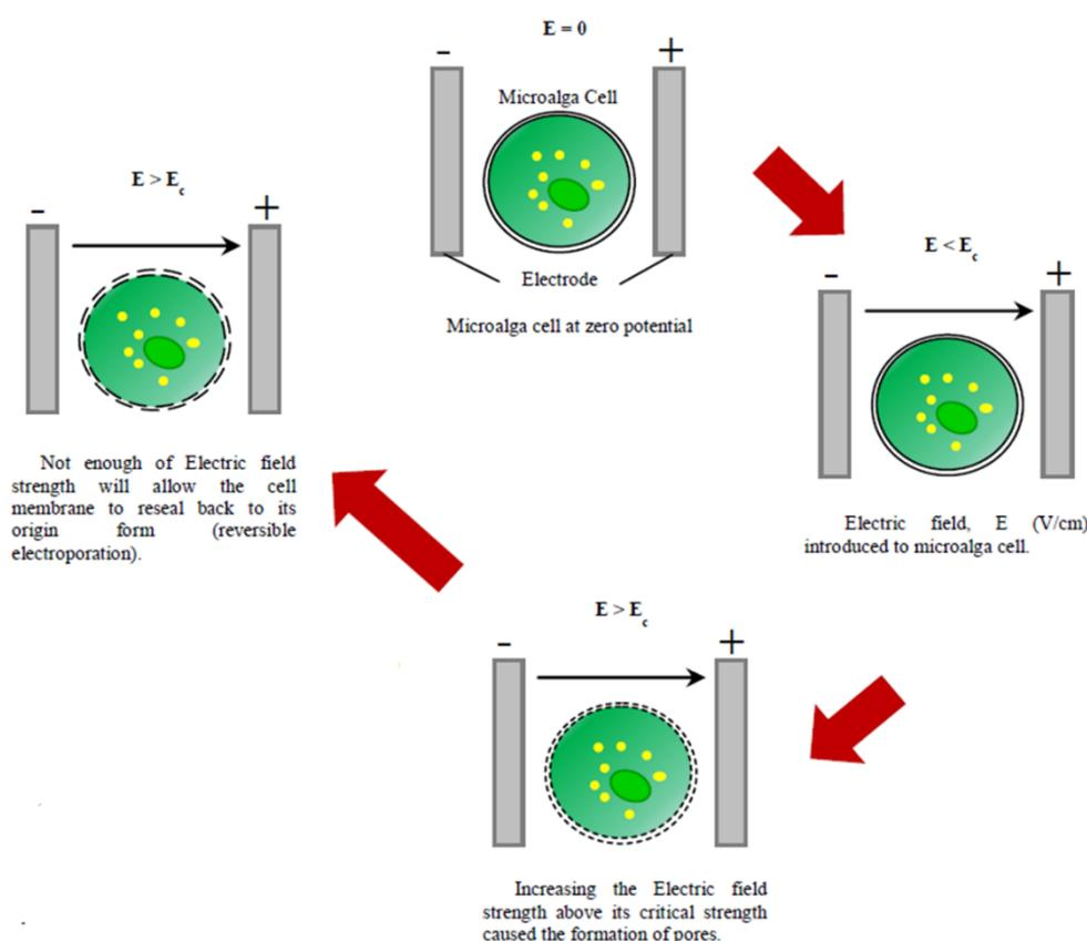
**Figure 8: Schematic representation of the permeabilization mechanism when the microalga's membrane is exposed to an electric field  $E$  (modified from Joannes *et al.*, 2015).  $E_c$ : critical electric field strength.**
