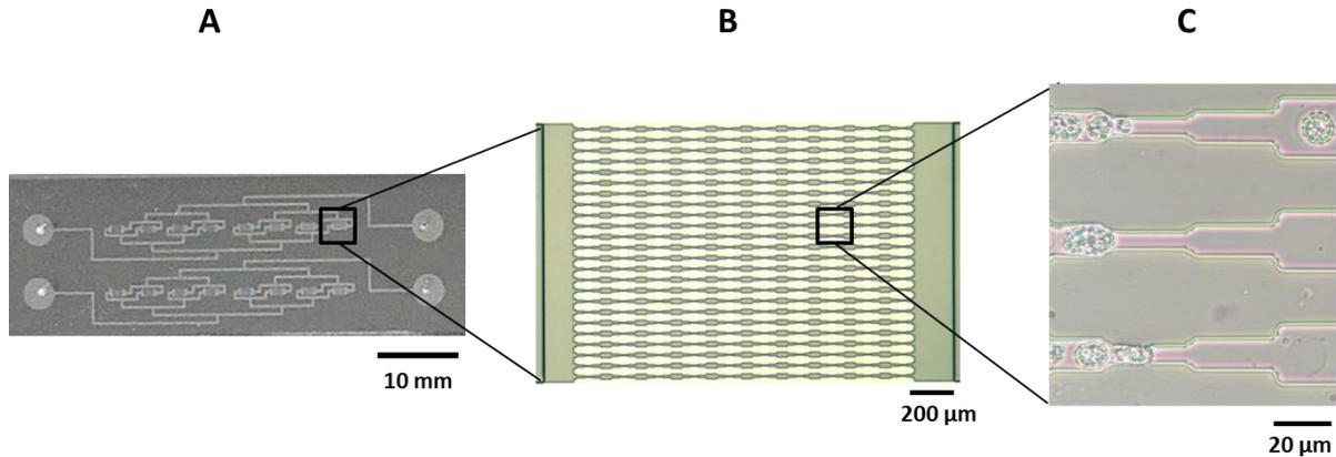
**Fig. 1** (A) image of the microfluidic device : double layer PDMS on a microscopic glass slide, (B) microscopic observation of one analysis frame, (C) microscopic observation of *Chlamydomonas reinhardtii* cells flowing through constrictions (under bright field).
