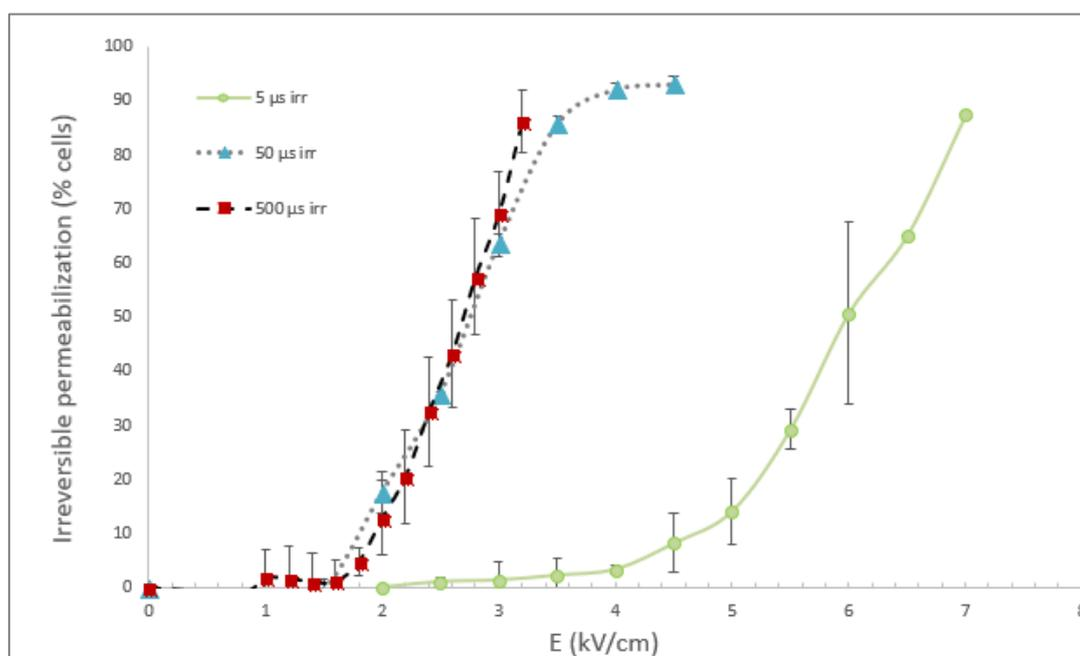
Figure 3: Impact of the electric field on the irreversible permeabilization (IP cells) obtained using 5, 50 and 500  $\mu\text{s}$  pulses respectively (burst 10 square pulses with 10 Hz frequency). Experiments were performed on *Chlamydomonas reinhardtii* cells at 7 days of stress. Error bars corresponds to standard deviation (SD). Means and associated SD are obtained from two independent assays.
