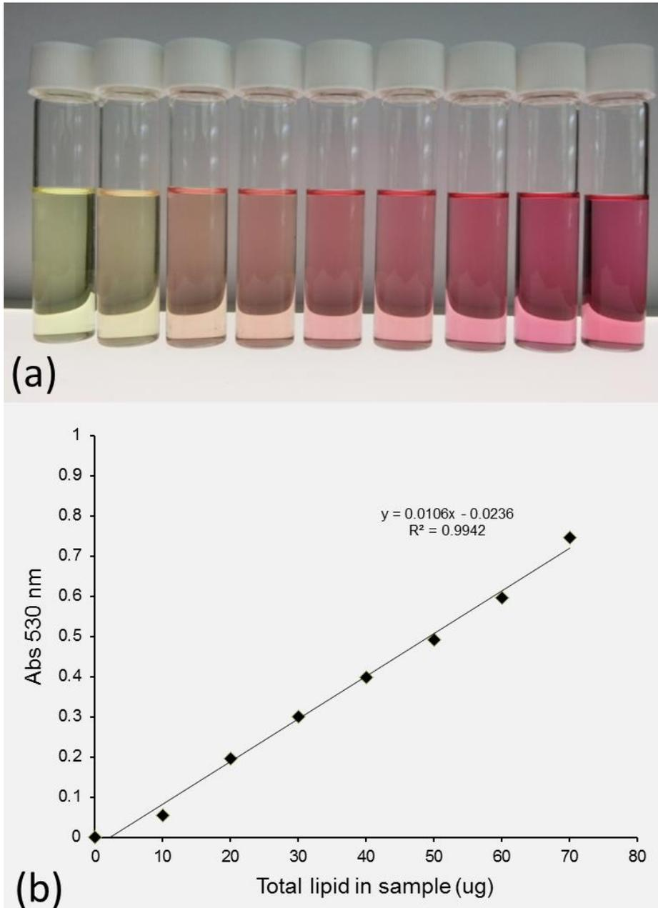
Figure 20: (a) From the left to right, the color change with the increasing concentration of lipid (Canola Oil) and (b) the corresponding linear relationship of absorption enhancement at 530 nm against lipid quantity in the sample (canola oil in the picture from (Mishra *et al.*, 2014)).
