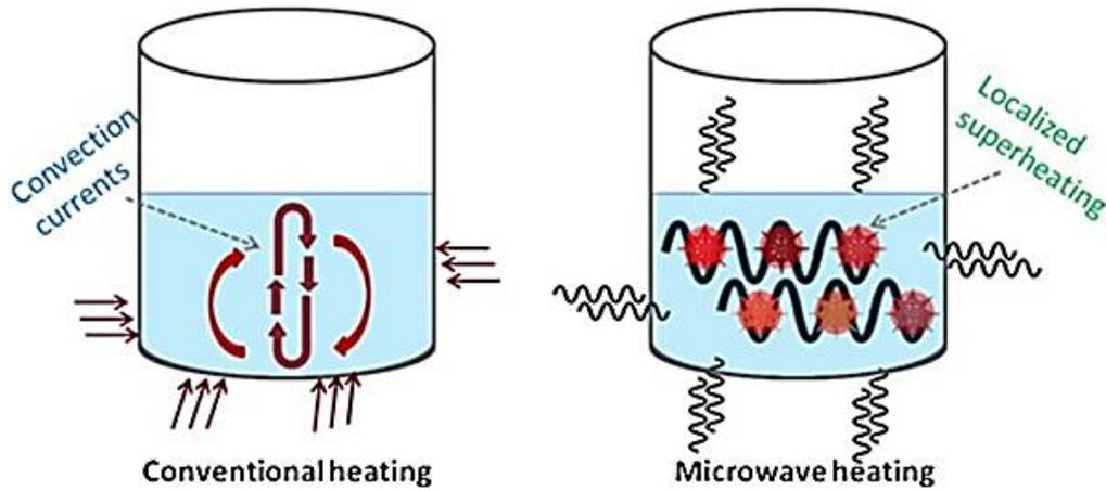
Figure 48: Conventional vs microwave heating (Gude et al., 2013).
