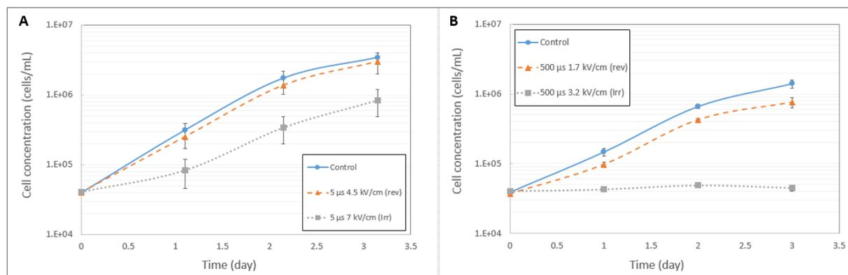
**Figure 6: Cell concentration over time after PEF treatment. A) 5  $\mu$ s pulses. B) 500  $\mu$ s pulses (straight line round marks: no PEF; dashed line triangular marks: 500  $\mu$ s, 1.7 kV/cm; dotted line square marks: 500  $\mu$ s, 3.2 kV/cm). Error bars corresponds to standard deviation (SD). Means and associated SD are obtained from two independent assays.**
