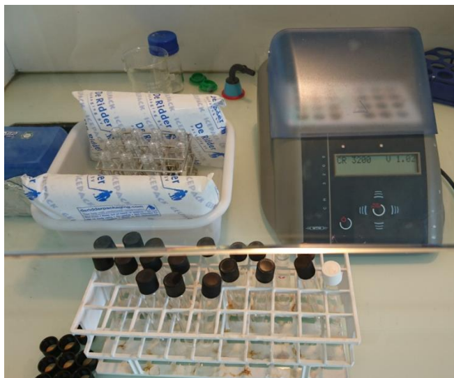
Figure 18: Tube heater (WTW CR3200) and ice cooling
