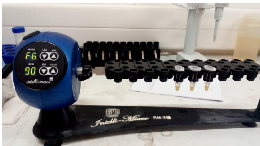
Figure 14: Agitating system used for the lipid extraction using solvents.
