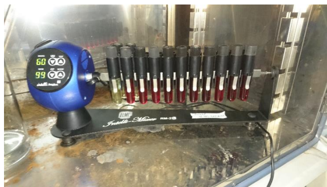
Figure 19: Mixing device (ELMI Intelli-Mixer, Mode F2, 99 Rpm) in a oven at 37°.
