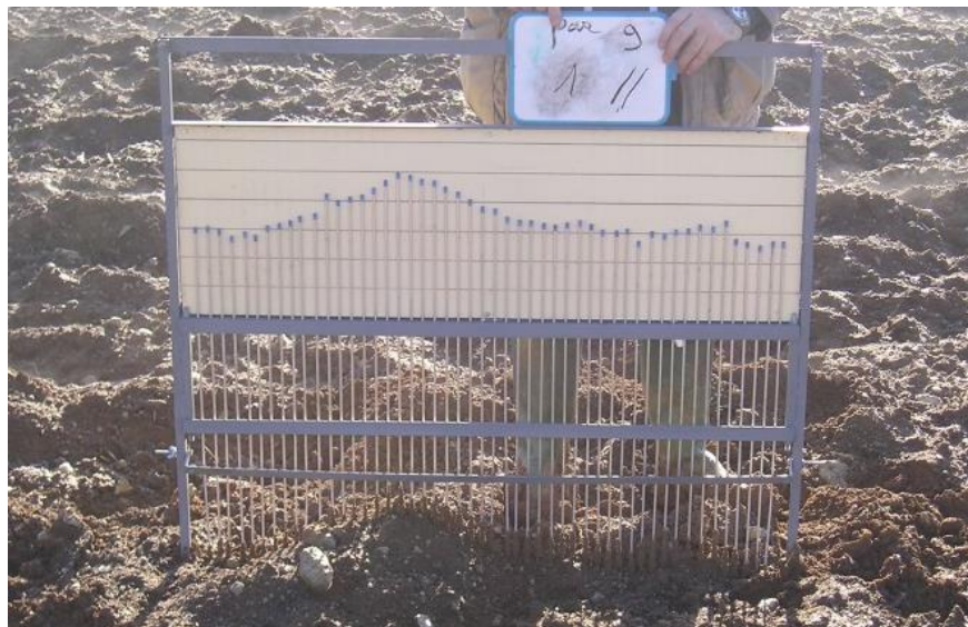
Figure II.2. Roughness profile made by a needle profile-meter in the parallel direction to the furrows (1D profile from a pin profilometer: 1 m long and a sampling interval of 2 cm) (Baghdadi and Zribi, 2016).
