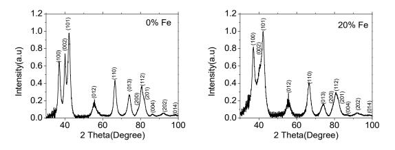
Figure 2.4. XRD diffractogram of bare ZnO (left) and  $R_{Fe} = 0.2$  (right) NPs.
