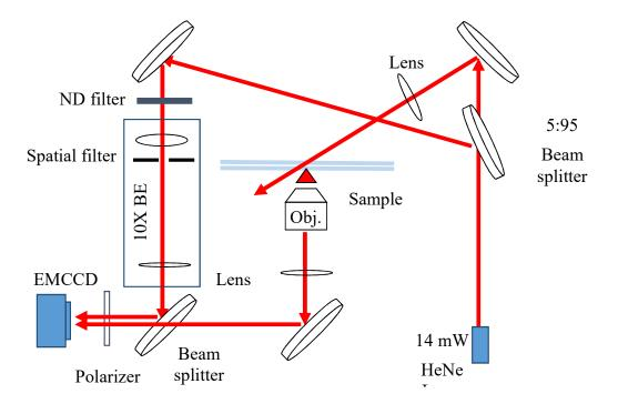
*Figure 3.3. Dark field interference microscopy configuration.*
