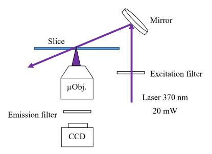
*Figure 3.1. Fluorescence microscopy configuration.*
