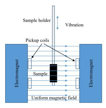
Figure A.6. Schematic diagram of a vibrating sample magnetometer.
