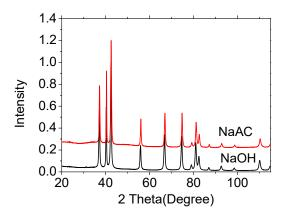
Figure E.2. XRD diffractogram of DEG-ZnO NPs synthesized with Na<sup>+</sup>.
