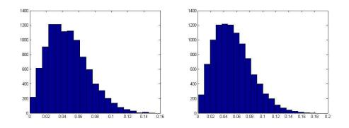
Figure K.2. Error histograms of the center of mass method algorithm (left) and of the Gaussian fitting method algorithm, without noise.
