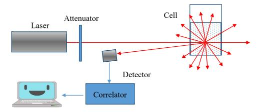
Figure A.5. Schematic diagram of DLS.
