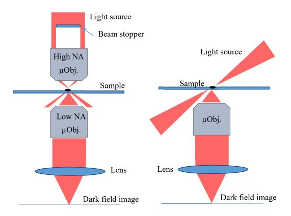
*Figure B.3. Some types of dark field illumination configuration.*
