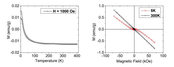
Figure 2.5. Magnetization (M) versus temperature (left) and versus applied field (H) at 5 K and 300 K (right) of  $R_{Fe}$ = 0.2 NPs synthesized in PG.
