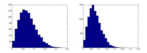
Figure K.3. Error histogram of the center of mass method algorithm (left) and the Gaussian fitting method algorithm, with shot noise.
