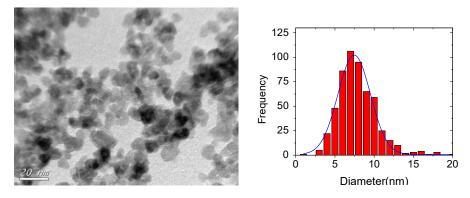
Figure 2.2. TEM images and size distribution of bare ZnO NPs.
