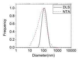
Figure 3.14. Hydrodynamic size of CMP-NPs measured by NTA and DLS.
