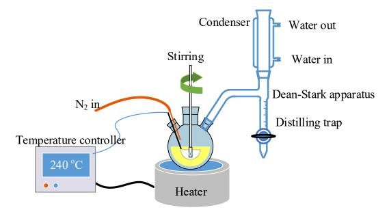
Figure 2.1. Experimental setup for synthesis of NPs with Dean-Stark apparatus.
