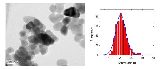
Figure E.3. TEM image and size distribution of DEG-ZnO NPs with dried salt.
