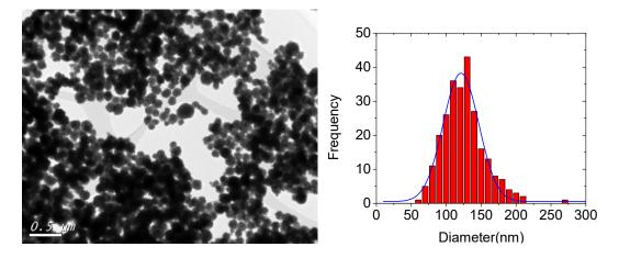
Figure D.1. TEM images and size distribution of PG-ZnO NPs with water.
