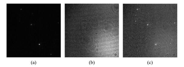
Figure 3.4. Dark field image of NP (a), reference laser beam (b) and interference image (c).
