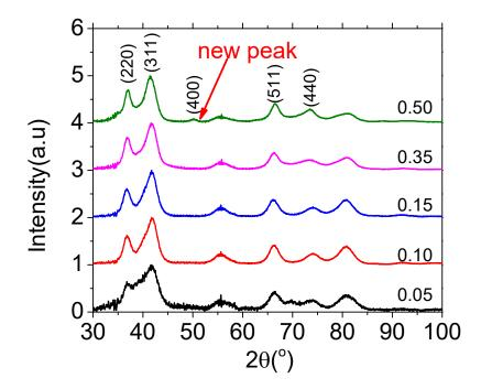
Figure 2.7. XRD diffractograms of  $R_{Fe, i} = 0.05, 0.10, 0.15, 0.35$  and 0.50.
