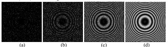
Figure L.1. Simulated interference images of NP versus SNR: 10 (a), 100 (b), 1000 (c), and 10000(d)
