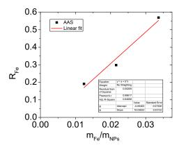
Figure N.1. Determination of relationship between  $R_{Fe}$  and  $m_{Fe}/m_{NPs}$ .
