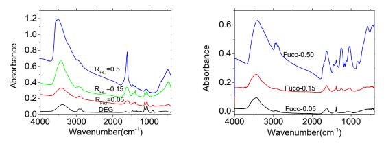
*Figure H.4. Infrared absorption spectral of bare NPs and Fu-NPs with different Fe concentration.*
