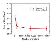
Figure K.5. Error of the Gaussian fit algorithms and the center of mass algorithms versus the number of incoming photons
