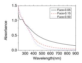
Figure H.2. Absorption spectra of fuco-NPs with different Fe concentrations.
