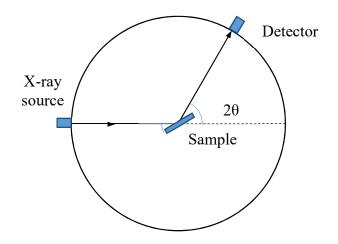
Figure A.3. Schematic diagram of X-ray diffractometer.
