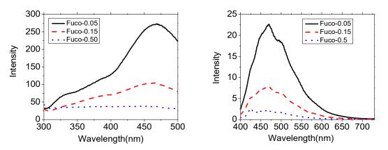
Figure H.3. Fluorescence spectra of fuco-NPs with excitation wavelengths of 270 nm (left) and 370nm (right) with different Fe concentrations.
