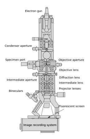
Figure A.1. Layout of optical components in a basic TEM.
