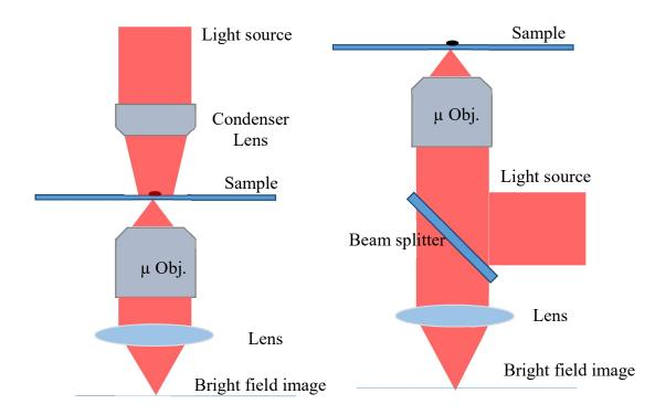
Figure B.2. Some type of bright field illumination configurations: transmission (left) and reflection (right).
