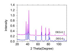
Figure E.6. XRD diffractogram of pure ZnO and DEG-0.1.
