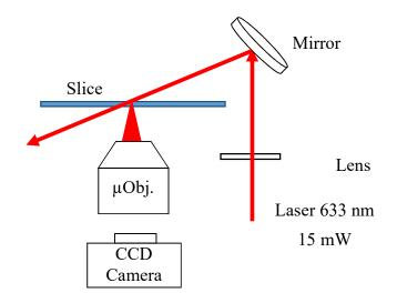
Figure 3.2. Dark field microscopy configuration.
