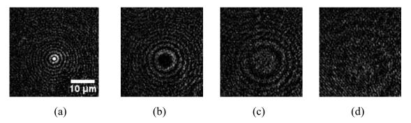
Figure 3.17. Interference images of NP as a function of z:  $0 \mu m$  (a),  $20 \mu m$  (b),  $40 \mu m$  (c), and  $100 \mu m$  (d).
