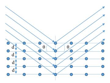
Figure A.2. X-rays scattered by crystal.
