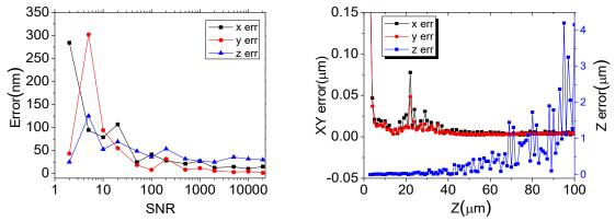
Figure L.2. Error versus SNR (left) and distance to focus plane (right).
