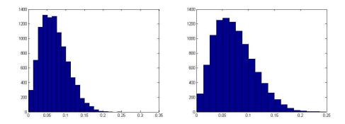
Figure K.4. Error histogram of the center of mass method algorithm (left) and the Gaussian fitting method algorithm, with shot noise and background
