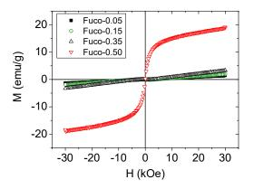
*Figure H.1. Magnetization (M) versus applied field (H) curves of fuco-NPs with different Fe concentrations.*
