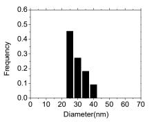
Figure 3.12. Hydrodynamic size of  $R_{Fe, i} = 0.2$  NPs measured by NTA.
