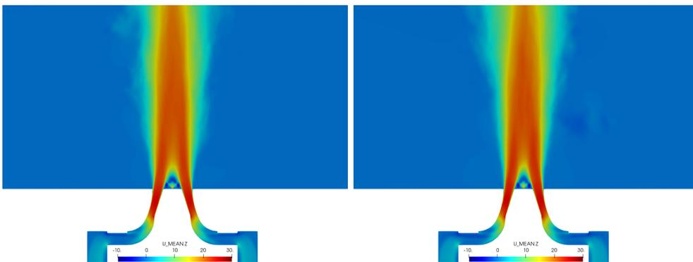
**Figure 3.7:** Mean axial velocity fields for cases A-NR (left) and B-NR (right) in the central vertical plane.
