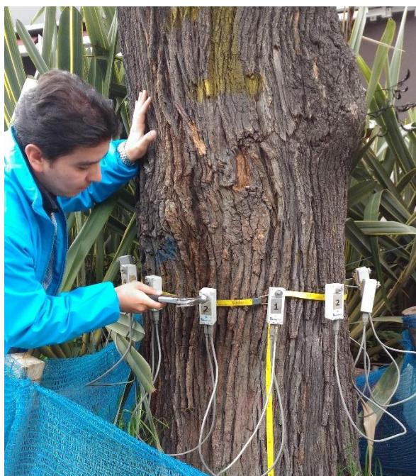
Figure 8: Acoustic testing of a standing tree in Bogota using an Arbotom device.
