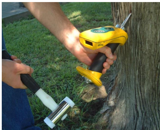
Figure 5: Example of use of acoustic hammer: Hitman ST300 for standing tree evaluation (source: https://www.fibre-gen.com/hitman-st300 )
