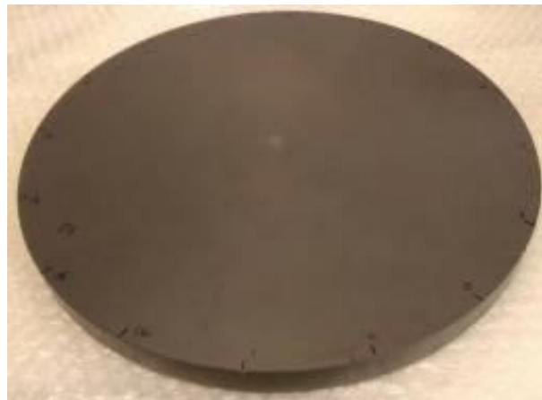
Figure 60: PVC disk for comparison with the isotropic case. Disk diameter of 30 cm and a thickness of 3 cm (Espinosa et al. 2019).
