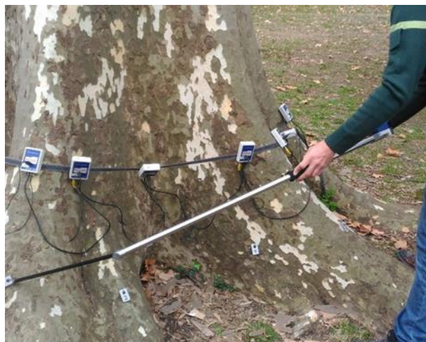
Figure 6: Picus Sonic Tomograph from Argus Electronic GmbH.
