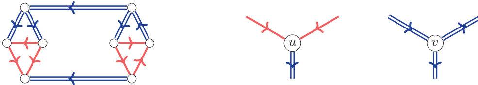
Figure 2.6: On the left, an example of an NCL machine with a valid orientation. Double edges in blue are weight 2 edges, the red ones are weight 1 edges. On the right an example of an AND node u , and an OR node v .
