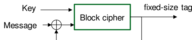
(b) Block cipher in feedback mode (similar to hash function)
