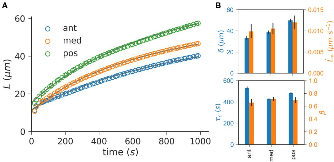
FIGURE 4.11 – Example of a series of aspirations on a PSM along the anteroposterior axis. **A:** Aspiration curves for  $\Delta P = 294 \text{ Pa}$  and  $R_p = 18.6 \mu\text{m}$ . Circle: tracked data points of the kymograph. Solid line: modified SLS fit. (ant: anterior, med: medial, pos: posterior). **B:** Fitted parameters for each curve.
