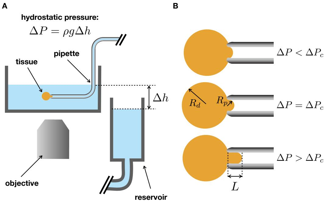
FIGURE 4.1 – Micropipette aspiration principle. **A:** Schematic of the aspiration experimental setup. **B:** Schematic of a viscous spherical drop aspirated under different regimes of pressure,  $\Delta P < \Delta P_c$ : the curvature within the pipette increases with the pressure,  $\Delta P = \Delta P_c$ : the curvature within the pipette is maximal ( $2/R_p$ ),  $\Delta P > \Delta P_c$ : the curvature within the pipette is maximal and stays constant, and the drop flows into the pipette.
