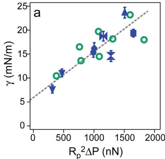
FIGURE 4.4 – Dependency of tension on the force of aspiration in cellular aggregates. Blue: calculated using relation 4.18. Green: calculated using the mean value of  $\eta$  and the measured value of  $\dot{L}_\infty^a$  with relation 4.16. Adapted from Guevorkian et al., 2010
