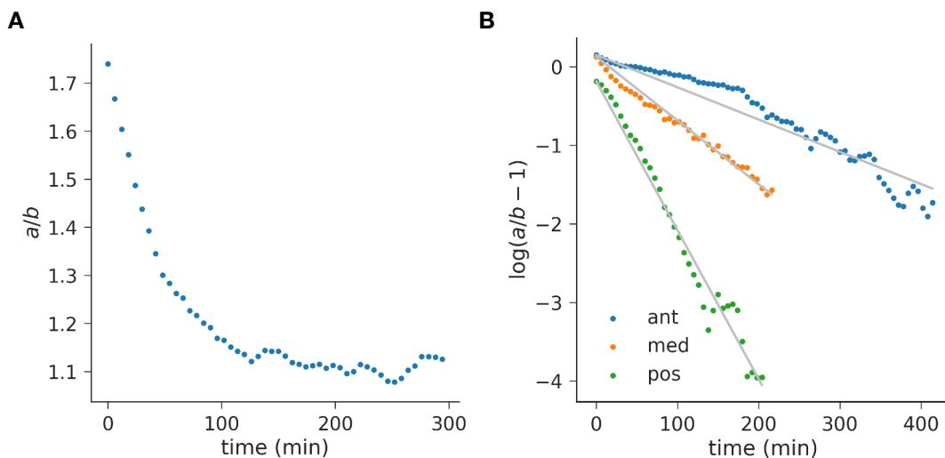
FIGURE 3.4 – Measurement of the rounding dynamics along the anteroposterior axis. **A:** Typical exponential decay of the aspect ratio  $a/b$  for a medial explant. **B:** Semilog plots of  $a/b$  along the antero-posterior axis (ant: anterior, med: medial, pos: posterior). Solid lines: linear fits with  $a_0/b_0$  fixed.
