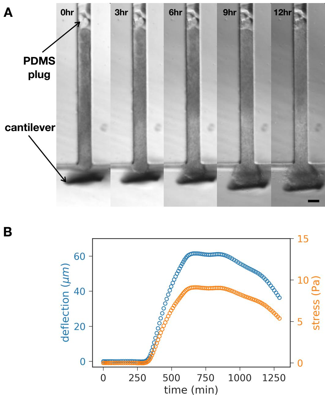
FIGURE 5.19 – PSM explant stress production over time. **A:** Snapshots during an elongation of a full PSM explant deflecting a cantilever. Scale bar: 75  $\mu\text{m}$ . **B:** Deflection and stress measurement over time.
