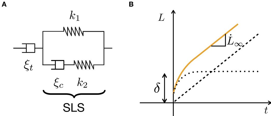
FIGURE 4.3 – The modified Standard Linear Solid model. **A:** Schematic of the modified Standard Linear Solid (SLS) model comprising a dashpot element in series with a SLS element. **B:** Schematic of the strain response of the modified SLS model (solid orange line) to a sudden stress: the sum of the response of the SLS element (dotted line) and the response of the dashpot element (dashed line).
