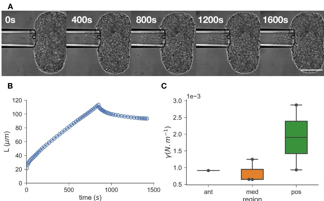
FIGURE 4.19 – Aspiration of blebbistatin treated explants. **A:** Series of snapshots of an aspiration and retraction (starting at 900s) of a medial region explant at 294 Pa. Scale bar: 100  $\mu\text{m}$ . **B:** Aspiration dynamics of the same explant. Solid line: modified SLS fit. **C:**  $\dot{L}_\infty$ -based measurement of surface tension.
