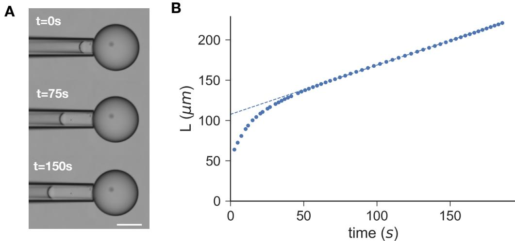
FIGURE 4.6 – Aspiration of an oil drop. **A:** Snapshots of an aspiration within a sodium hydroxide treated pipette at  $\Delta P = 2.65 \text{ kPa}$ . Scale bar:  $100 \mu\text{m}$ . **B:** Length  $L$  of the aspirated tongue over time.
