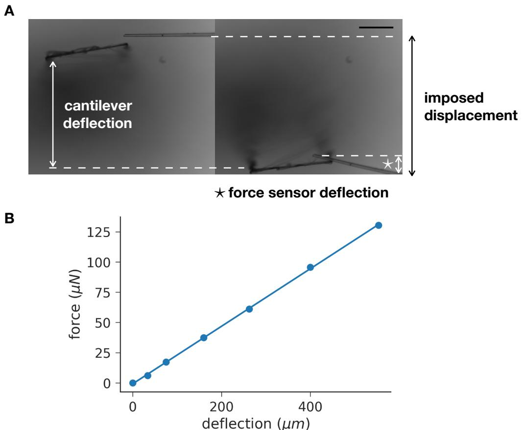
FIGURE 5.4 – Mica cantilever calibration. **A:** Snapshots of a deflection experiment (left picture: before deflection, right picture: deflected). Scale bar: 250  $\mu\text{m}$ . **B:** Force-deflection curve. Linear regression yields a stiffness of  $0.24 \text{ N} \cdot \text{m}^{-1}$ .
