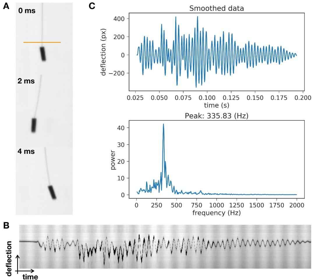
FIGURE 5.6 – Calibration of a glass rod cantilever. A: Snapshots of a high speed camera movie during oscillations of the cantilever. B: Kymograph along the orange line (top panel of A). C: Top panel: smoothed deflection data by moving average subtraction. Bottom panel: power spectrum obtained by Fourier transform.
