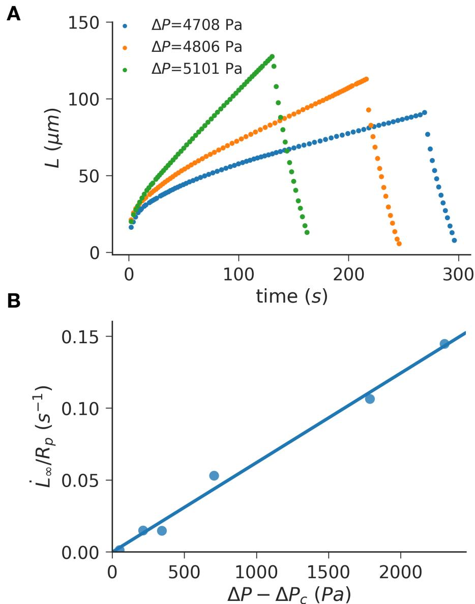
FIGURE 4.8 – Measurement of the oil standard viscosity. **A:** Aspiration and retraction curves of an oil drop at three different pressures.  $R_p = 21 \mu\text{m}$ . **B:** Linear regression of the scaled aspiration rate by the applied stress.
