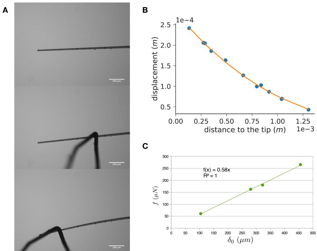
FIGURE 7.2 – Glass rod calibration. **A:** Snapshot of the rod deflection for a hanging weight at different positions. **B:** Deflection with respect to the weight distance to the tip, fitted by Equation B.5. **C:** Extrapolated deflection  $\delta_0$  with respect to the load.
