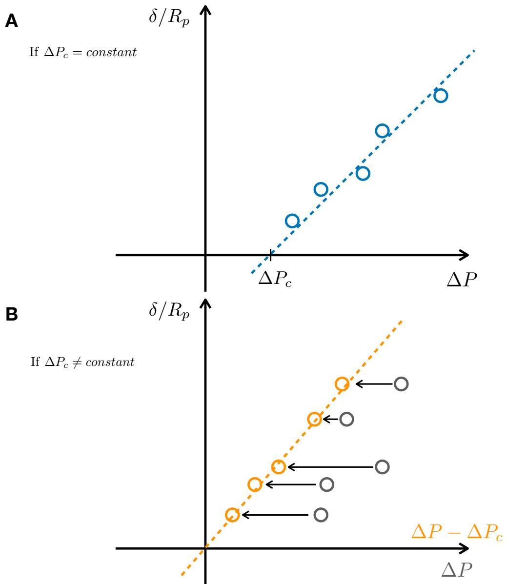
FIGURE 4.5 – Linear dependency of the fitting parameters  $\delta$  and  $\dot{L}_\infty$  with respect to the applied pressure  $\Delta P$ . **A:** Schematic of the linear dependency of the fitting parameter on  $\Delta P$ , if  $\Delta P_c$  is constant. **B:** Schematic of the linear dependency of the fitting parameter on  $\Delta P - \Delta P_c$  (orange points), if  $\Delta P_c$  is not constant. There is no linear relation with  $\Delta P$  (gray points).
