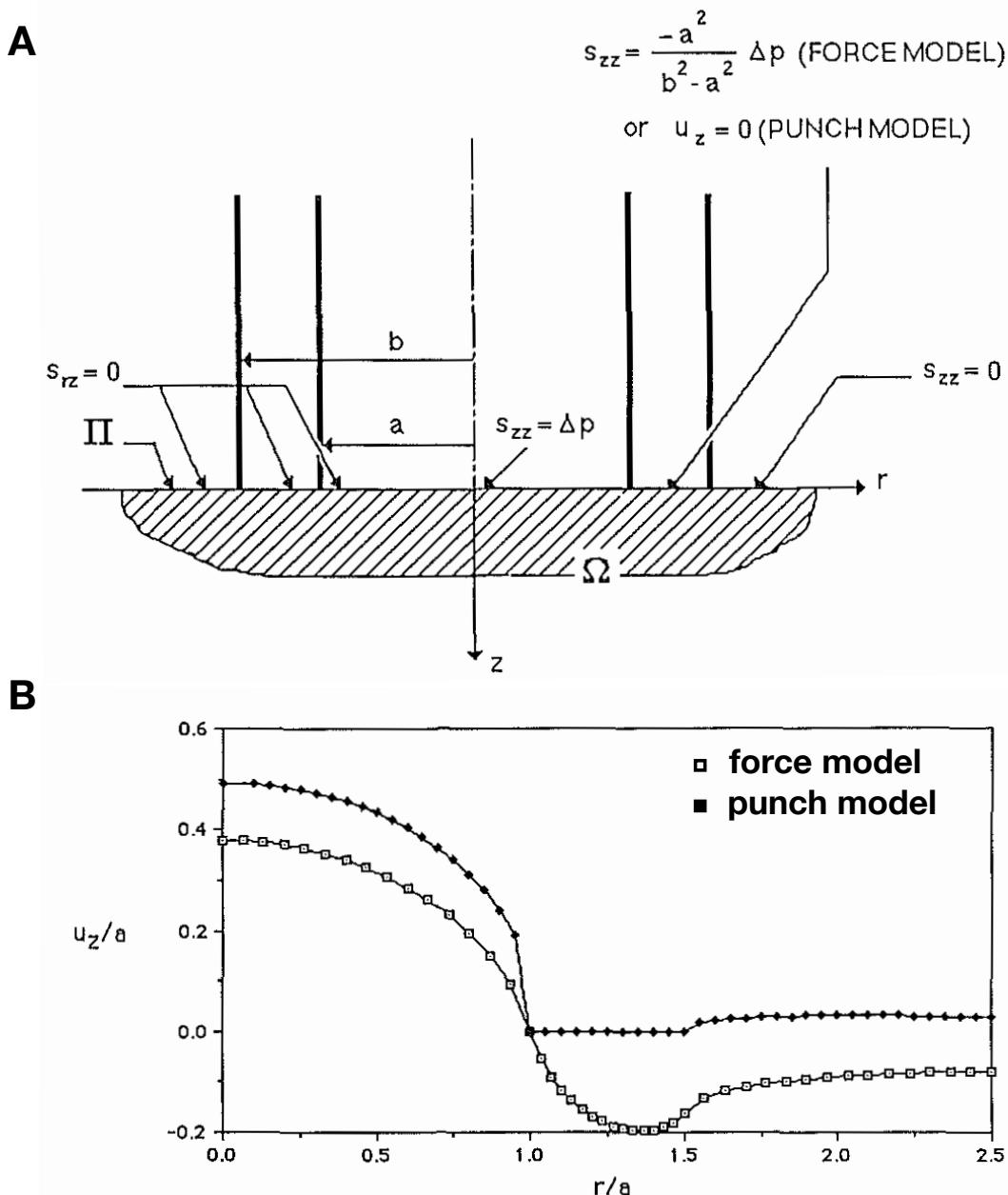
FIGURE 4.2 – Theory of elasticity measurement by pipette aspiration.
