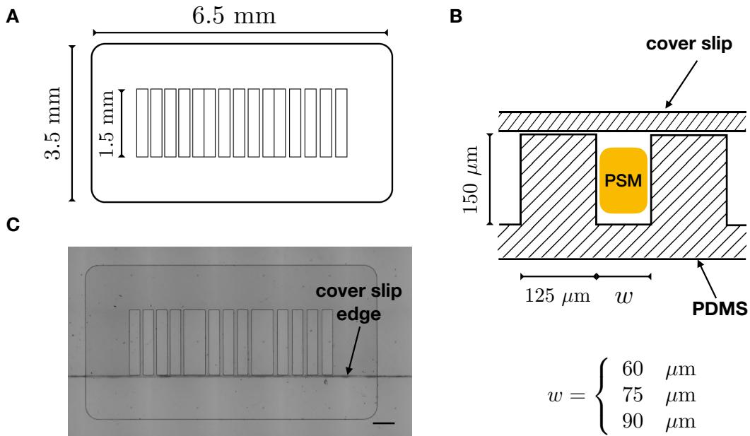
FIGURE 5.11 – Microchannels array fabrication. Schematic of the microchannels array in top view (A) and zoomed side view (B). C: Picture of the microchannels array. Scale bar: 250  $\mu\text{m}$ .
