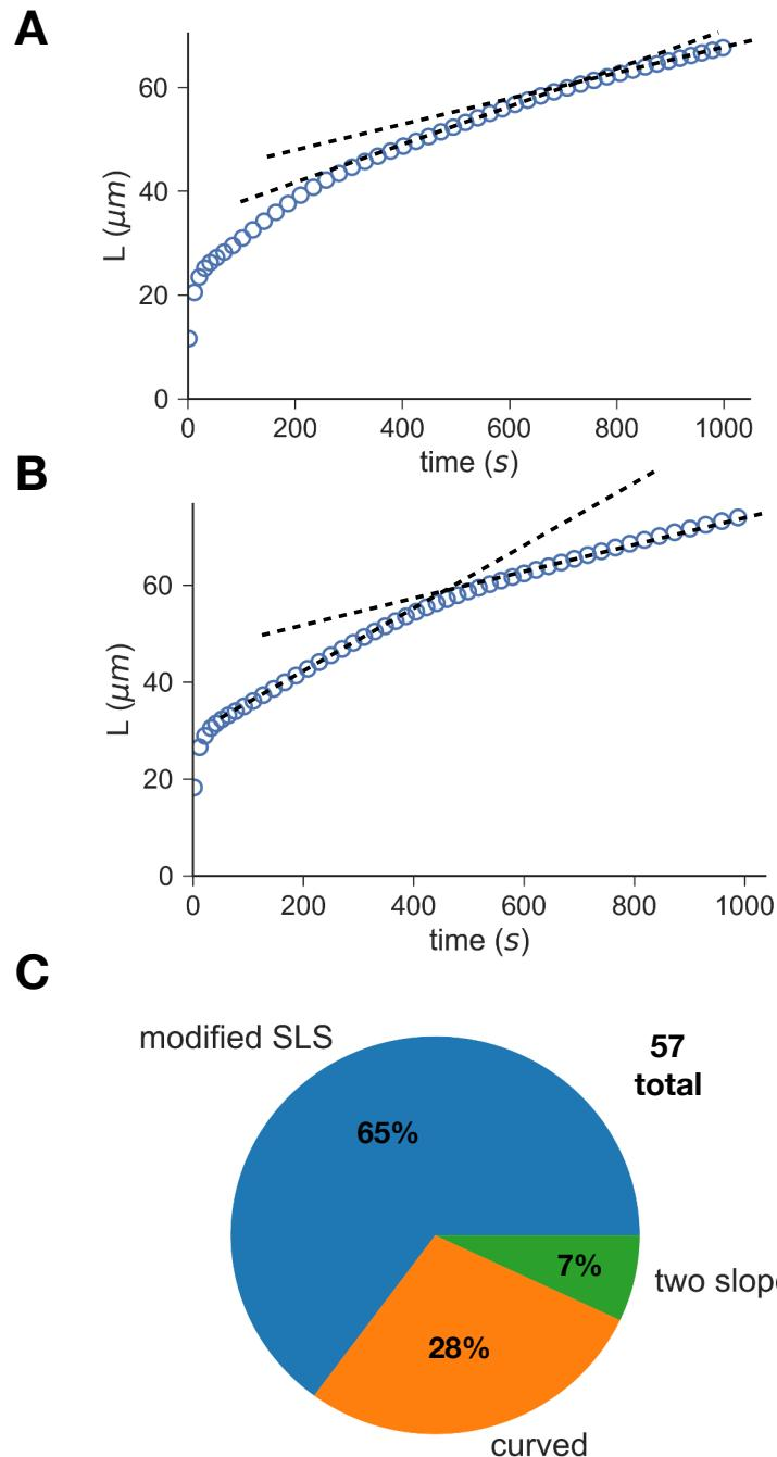
FIGURE 4.10 – Various kinds of aspiration curves. **A:** "Curved" shape aspiration for a posterior explant with  $\Delta P = 588$  Pa. **B:** "Two slopes" shape aspiration for a posterior explant with  $\Delta P = 588$  Pa. The dashed lines show the tangents to the curve at different times. **C:** Statistics of the different kinds of curve shapes.
