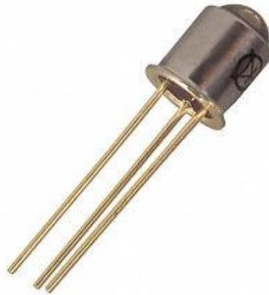
Figure 4.12 Fermionics Photodiode FD100L with lens cap [27].
