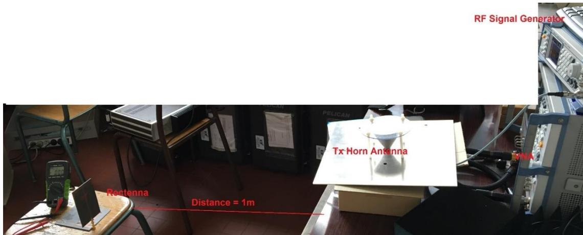
Figure 2.48 Experimental setup of the rectenna system.
