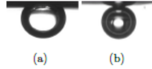
Figure 13: Apparent contact angle using a captive bubble method: (a) for flat control aluminium surface, (b) after 3h of pore opening
