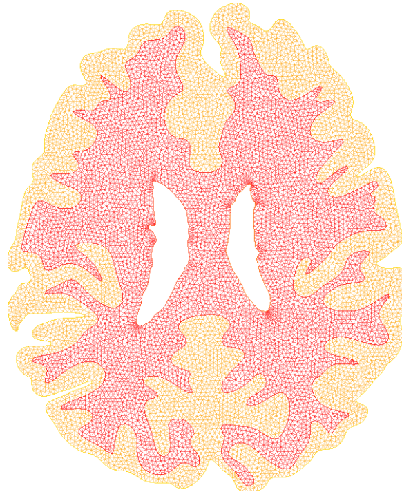
Figure 5.4: Grey and white matter segmentation and corresponding meshing (via FreeFem++), in view of a PDE resolution.
