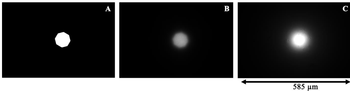
Figure 5.2: Knife edge illumination measurements: (A) perfect specular mirror, (B) glossy coated paper, (C) Epson standard proofing paper.
