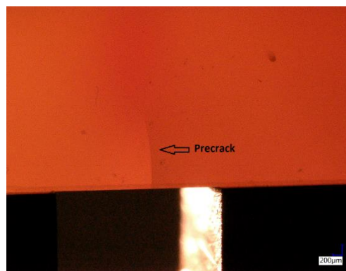
Figure 5.12 Sample with generated precrack.
