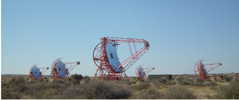
Figure 2.4: H.E.S.S. telescope array. The phase two large telescope CT5 is at the center of the array. The four first phase smaller telescopes CT1-4 are at the corners of the array. Figure extracted from Ref. [31].
