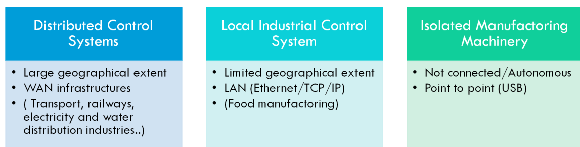
Figure 2.2 – The types of ICS systems according to geographical distribution.
