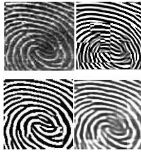
Figure 6.9: Fingerprint enhancement results (clock-wise from up-left): original fingerprint, Gabor filtered image, modified Gabor filtered image, and final anisotropic filter fingerprint.
