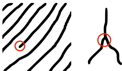
Figure 6.1: An example of fingerprint ridge ending (left) and bifurcation (right). Figures reproduced from [8].
