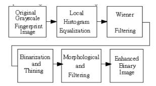
**Figure 6.7:** Flowchart of the binarization-based method. Figure reproduced from [152].
