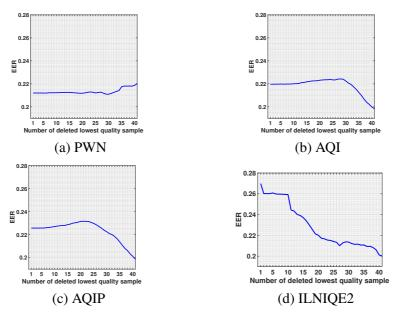
**Figure 8.18:** Examples of EER values with omitting low quality iris samples one by one until the best quality sample left for reflex camera.
