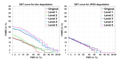
**Figure 5.6:** DET curve for blur and JPEG degradations in five levels of the NBIS system (D2O).
