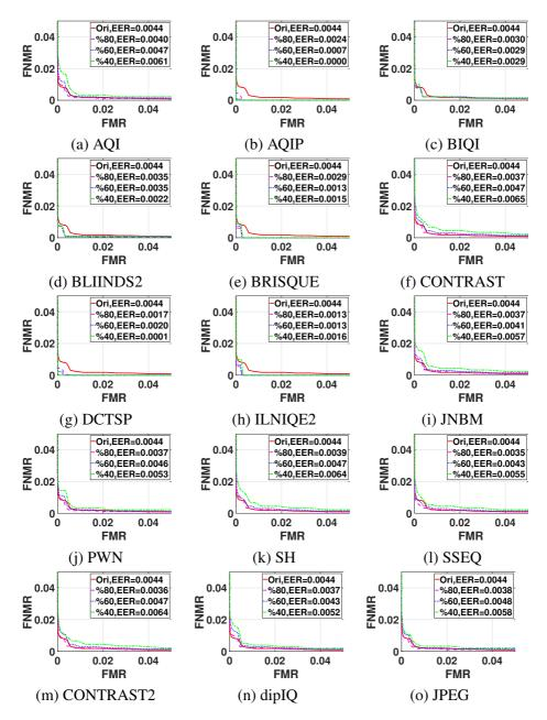
**Figure B.3:** DET curves with EER for comparison score with and without omitting low quality face samples for reflex camera by using GF+KFA face recognition algorithm.
