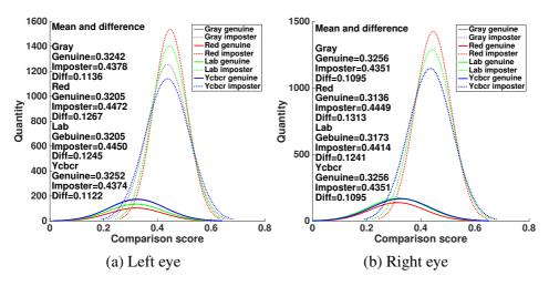
**Figure 7.5:** Comparison score and the difference of their mean values from left and right eye for reflex camera.
