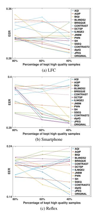
Figure 8.15: Tendency of EER values with and without omitting low quality samples.
