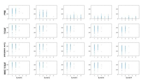
**Figure 5.7:** The scatter plots of the NFIQ quality measurement values (x axis) versus the comparison scores (y axis) for four degradations in five levels.
