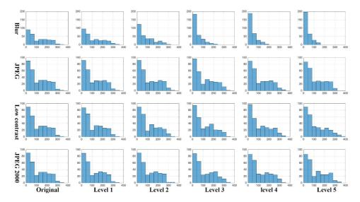
**Figure 5.3:** The histogram of genuine comparison score for original and degraded finger-prints. The scores of degraded fingerprints are the comparison between degraded finger-prints (probe) and degraded fingerprints (reference). The x axis represents the comparison score and y axis represents the number of score.
