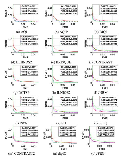
**Figure B.1:** DET curves with EER for comparison score with and without omitting low quality face samples for LFC by using GF+KFA face recognition algorithm.
