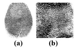
**Figure 6.2:** An example of (a) high quality fingerprint sample, and (b) low quality fingerprint sample.
