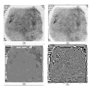
**Figure 6.14:** An example of experimental result from fingerprint enhancement approach proposed by Hatami *et al.*[163]. (a) is the original fingerprint, (b) is smoothed image, (c) is the Gabor filtered image, and (d) is the final enhanced binary fingerprint image.
