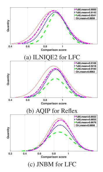
**Figure 8.2:** Examples of comparison scores and their mean values with omitting low quality samples by using GF+KFA recognition algorithm. The x-axis represents the comparison score, and the y-axis represents the quantity of the genuine comparison.
