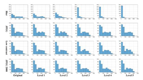
**Figure 5.2:** The histogram of genuine comparison score for original and degraded fingerprints. The scores of degraded fingerprints are the comparison between degraded fingerprints (probe) and original fingerprints (reference). The x axis represents the comparison score and y axis represents the number of score.
