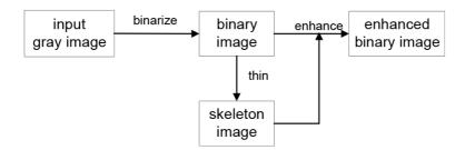
Figure 6.11: Flowchart of fingerprint enhancement method proposed by Luo et al.[159].
