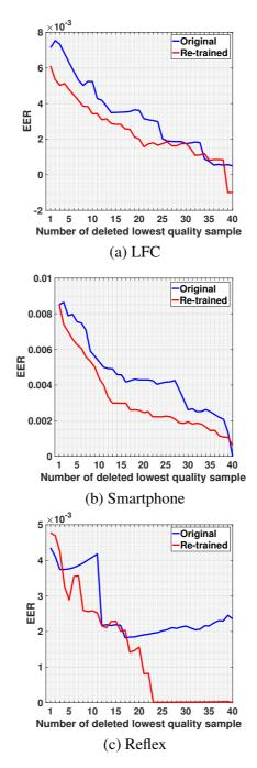
**Figure 8.9:** Comparison of EER by omitting lowest quality sample one by one using ILNIQE2 for each subject between the original method and the re-trained method.
