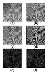
**Figure 6.8:** Experimental results of the binarization-based method. (a) is the original fingerprint, (b) is the contrast enhanced image, (c) is the Wiener filtered image, (d) is the binarized image, (e) is the thinned image, and (f) is the final enhanced fingerprint sample.
