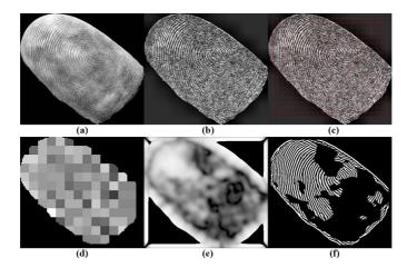
**Figure 6.26:** An example of the enhancement result after the second step. (a) represents the enhanced fingerprint after the step 1, (b) represents the normalized fingerprint, (c) represents the estimated orientation fingerprint, (d) represents the estimated ridge frequency fingerprint, (e) represents the orientation reliability, and (f) represents the final masked Gabor filtering fingerprint.
