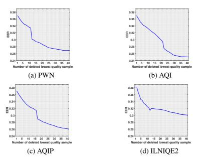
**Figure 8.17:** Examples of EER values with omitting low quality iris samples one by one until the best quality sample left for smartphone.
