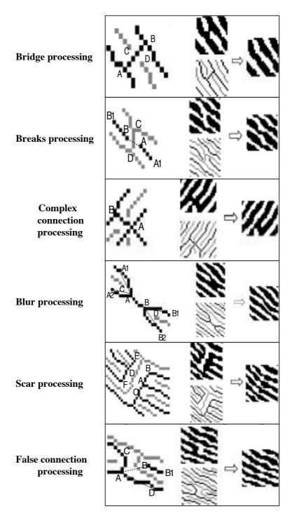
**Figure 6.10:** Demonstration of rules for method 4. Figures reproduced from Luo *et al.* [159].
