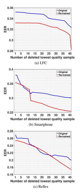
**Figure 8.19:** Comparison of EER by omitting lowest quality sample one by one using ILNIQE2 for each subject between the original method and the re-trained method.
