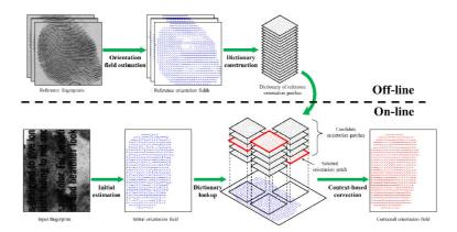
**Figure 6.18:** The flowchart of the proposed method by Feng *et al.*[168]. This approach contains an off-line dictionary construction stage and an on-line orientation field estimation stage.
