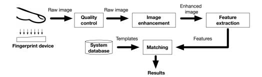
**Figure 2.3:** Flow chart of a fingerprint recognition system. Reproduction inspired by Maltoni *et al.* [23].
