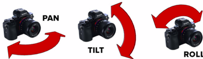
Figure 4.9: The rotation composed by three degrees of freedom on pan tilt roll (\alpha, \beta, \gamma) .
