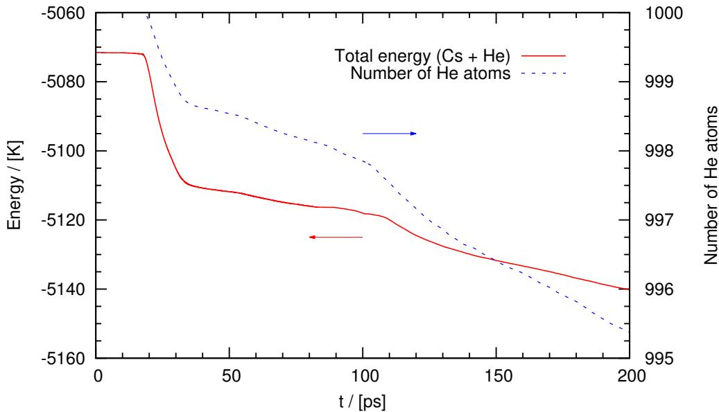
**Figure 8.5:** Total energy (left scale) and number of atoms in the droplet (right scale) as a function of time for the  $\text{Cs}@\text{He}_{1000}$  system at  $v_0 = 200$  m/s. (Color figure online.)
