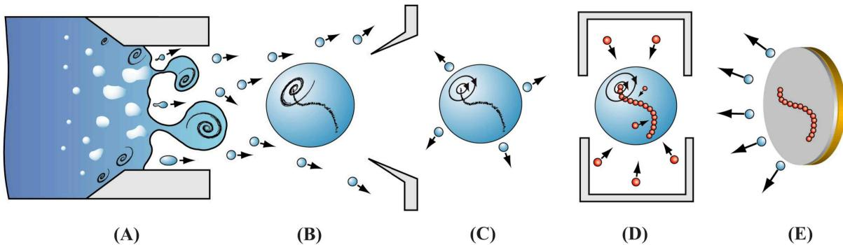
**Figure 7.1:** Schematic of the experiment. (a) He fluid expands in vacuum and (b) breaks up into rotating droplets. (c) A quantum vortex is formed as a consequence of fast evaporative cooling of the droplet to below  $T_\lambda$ . (d) The droplet is doped with Ag atoms, which are attracted to the vortex core. (e) The droplet then collides with the carbon surface leaving behind the Ag trace, whereas the He evaporates. (Illustration courtesy of Gomez *et al.* 2012, see Ref. [103])
