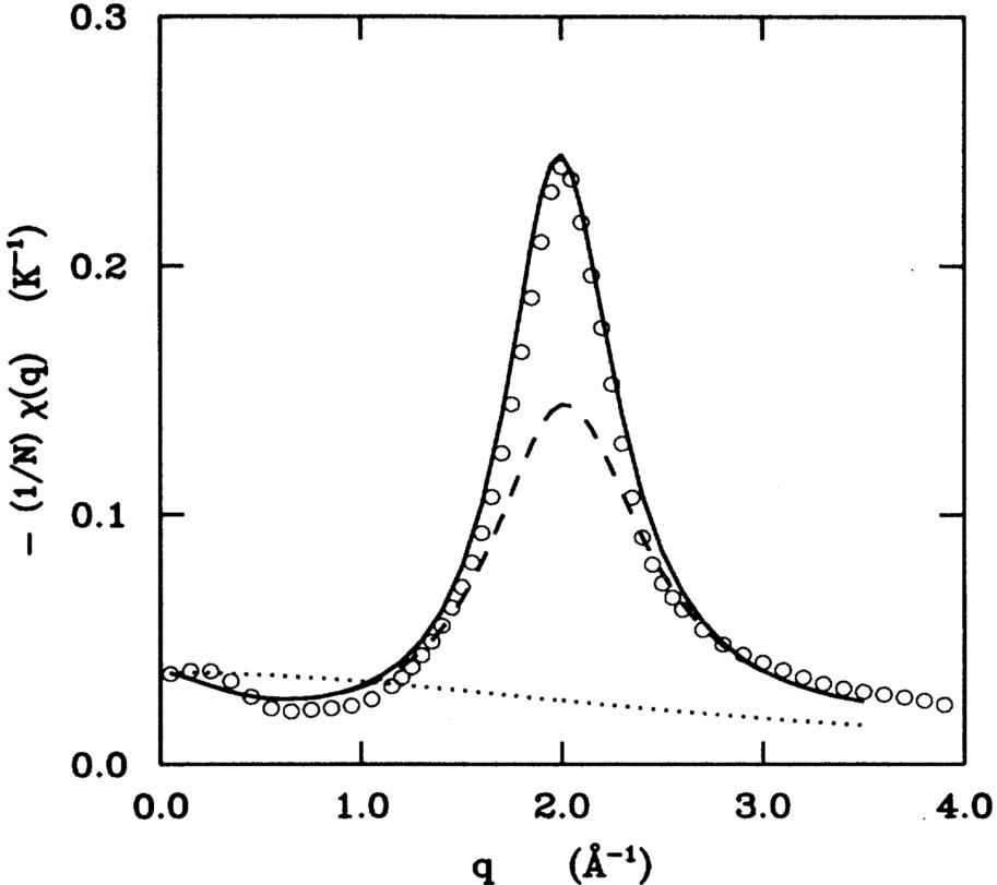
**Figure 2.1:** Static response  $-\chi$  (see Ref. [29], Eqn. (11)) per atom of liquid  ${}^4\text{He}$  at zero pressure. Points: experimental data; dotted line: from the functional of Refs. [51, 52]; dashed line: Orsay-Paris (OP) functional<sup>[57]</sup>; solid line: OT functional.
