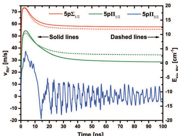
Fig. 6 Velocity (solid lines, left scale) and kinetic energy (dashed lines, right scale) of the Rb atom excited to the 5p-state as a function of time. The kinetic energy of the  $5p^2\Pi_{3/2}$ -state is not given as this state remains bound to the droplet.
