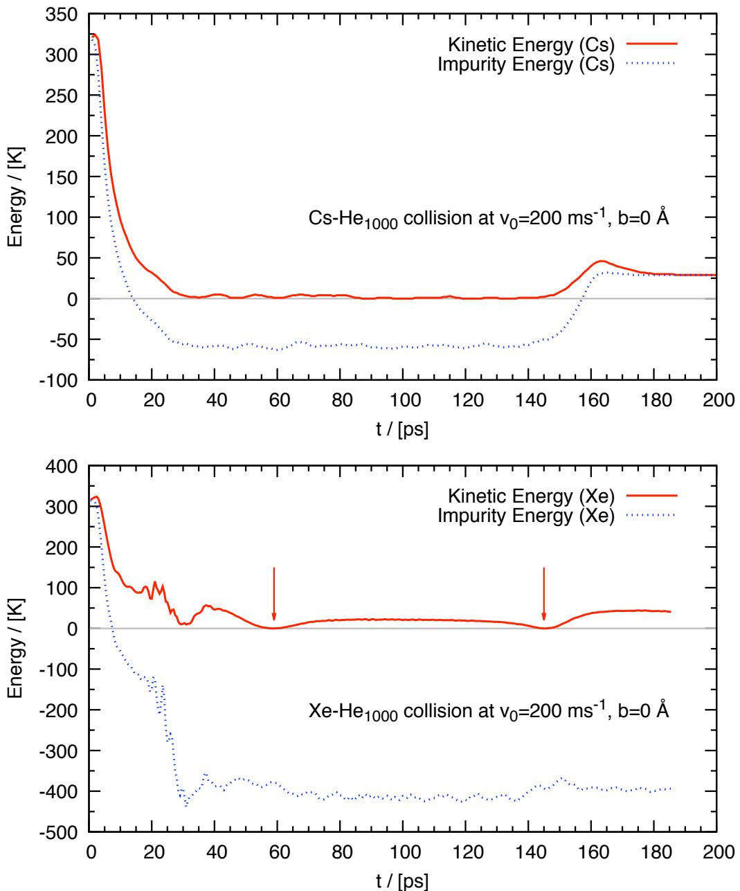
**Figure 8.3:** Top figure: Kinetic and total (kinetic plus potential) energy as a function of time of a Cs atom head-on colliding against a  ${}^4\text{He}_{1000}$  droplet at  $v_0 = 200$  m/s. Bottom figure: same as top figure for a Xe atom. The vertical arrows indicate the first two turning points at 59 and 145 ps, whose corresponding helium densities are shown in the right Figure 8.2. (Color figure online.)
