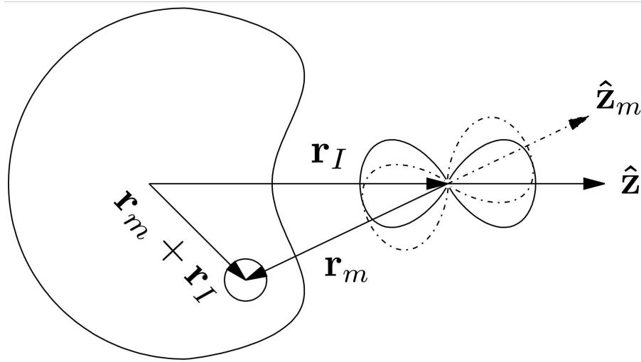
**Figure 2.3:** The set of axis defined in the DIM description. (Illustration courtesy of M. Martinez<sup>[61]</sup>.)
