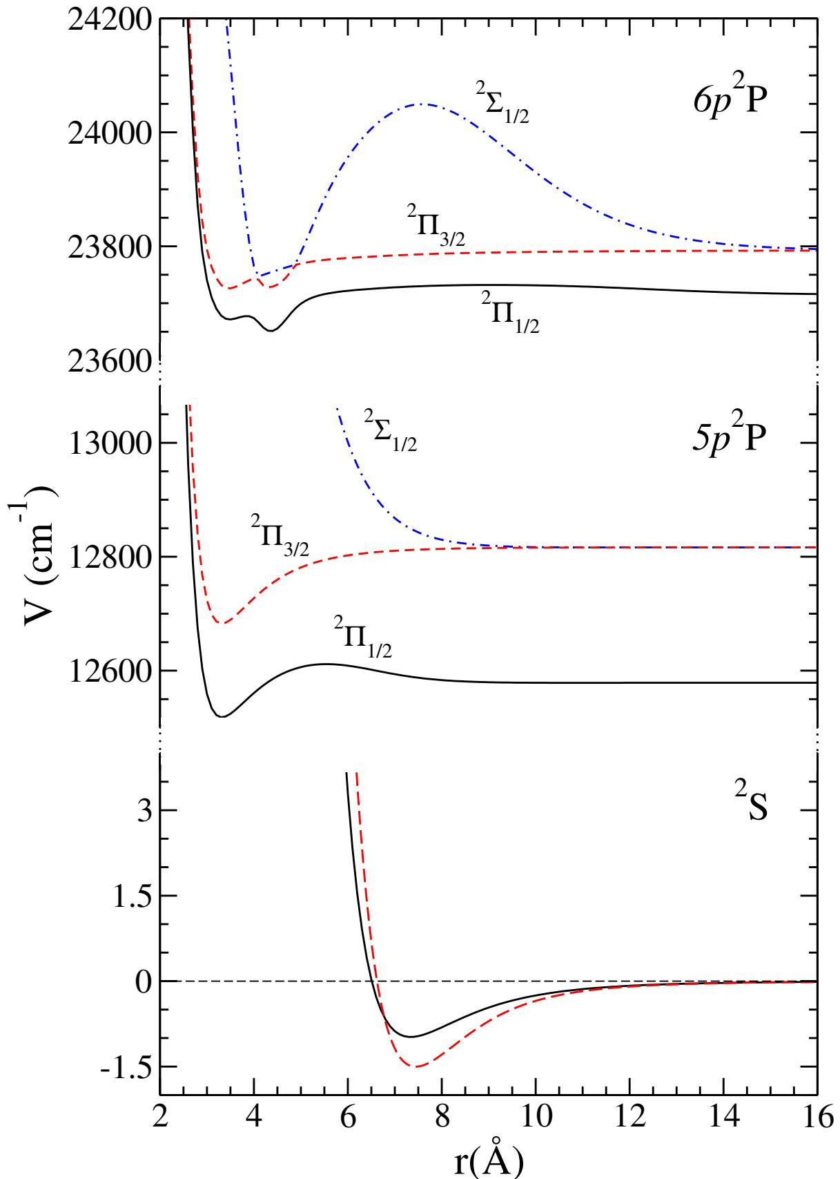
**Figure 5.1:**  $^2S$ ,  $5p^2P$ , and  $6p^2P$  Rb-He pair potentials used in this work. The splitting introduced by the spin-orbit interaction has been included. The  $^2S$  He-Rb pair potential of Ref. [99] is also displayed (bottom dashed line).
