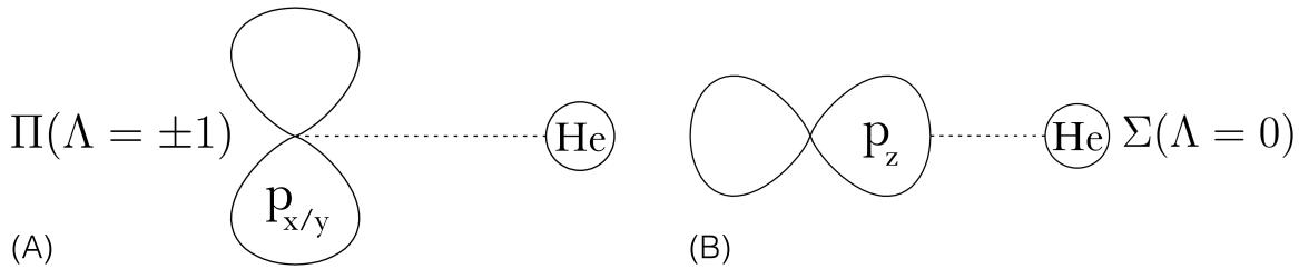
**Figure 2.2:** Level splitting of the p-orbitals in the presence of helium, that breaks the spherical symmetry. (A) A double degenerate  $n'p_{x/y}$ -orbital and (B) a single  $n'p_z$ -orbital. (Illustration courtesy of M. Martinez<sup>[61]</sup>.)
