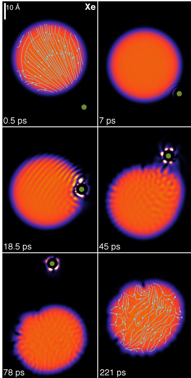
**Figure 9.6:** The same process as in Figure 9.5 but with an impact parameter  $b = 22.2 \text{ \AA}$  instead of  $b = 20.3 \text{ \AA}$ . Note that in this case, after about 78 ps (bottom left panel), the Xe atom is ejected with some helium density attached to it. See the ESI<sup>[139]</sup> for the movie of the complete evolution.
