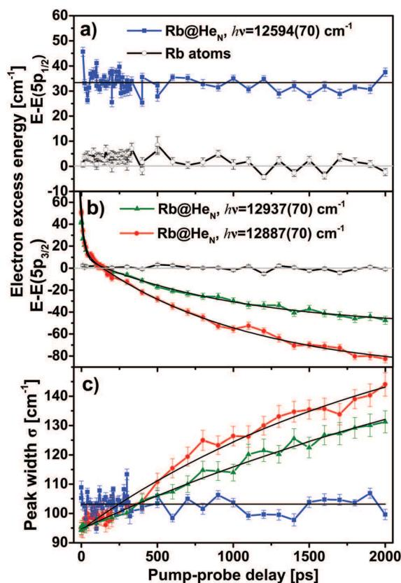
Fig. 4 Photoelectron energies as a function of pump–probe delay (filled circles) recorded at laser wavelengths  $\lambda = 794$  nm ( $12\,594\text{ cm}^{-1}$ ,  $5p^2\Pi_{1/2}$ ) (a),  $\lambda = 773$  nm ( $12\,937\text{ cm}^{-1}$ ,  $5p^2\Sigma_{1/2}$ ), and  $\lambda = 776$  nm ( $12\,887\text{ cm}^{-1}$ ,  $5p^2\Pi_{3/2}$ ) (b). Open circles indicate the electron energies measured for atomic Rb background signal. The widths of electron distributions are depicted in (c).
