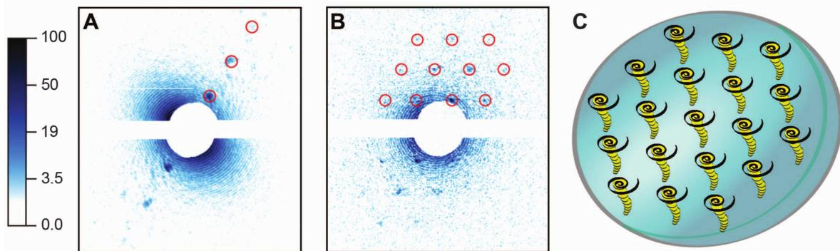
**Figure 7.2:** He droplets doped with Xe atoms. (A and B) X-ray diffraction images of doped droplets, displayed in a logarithmic intensity scale. (C) Droplet and embedded Xe clusters. Images in (A) and (B) correspond to tilted and parallel alignments of the vortex axes with respect to the incident x-ray beam, respectively. (Illustration courtesy of Gomez *et al.* 2014, see Ref. [104])
