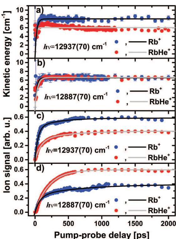
**Fig. 3**  $\text{Rb}^+$  and  $[\text{RbHe}]^+$  ion kinetic energies [(a) and (b)] and signal yields [(c) and (d)] recorded at laser wavelengths  $\lambda = 773\text{ nm}$  [ $12\,937\text{ cm}^{-1}$ , (a) and (c)] and  $\lambda = 776\text{ nm}$  [ $12\,887\text{ cm}^{-1}$ , (b) and (d)]. The smooth gray and black lines are fit curves (see text for details).
