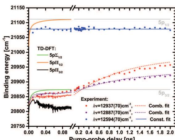
**Fig. 10** Comparison of experimental and simulated electron binding energies. Thick solid lines: TD-DFT results. Dashed lines: combined TD-DFT and analytical model. Thin solid lines: biexponential fits of the experimental data.
