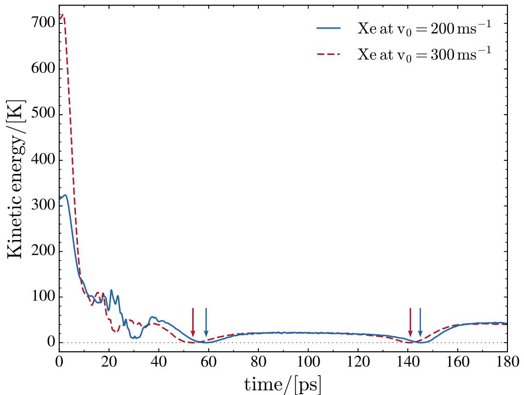
**Figure 9.2:** Kinetic energy of the Xe atom in the center of mass (COM) frame of the  ${}^4\text{He}_{1000}$  droplet as a function of time for a head-on collision at  $v_0 = 200$  and  $300$  m/s. The kinetic energy increase during the first few picoseconds is due to the acceleration produced by the attractive part of the Xe-He potential. The vertical arrows indicate the first two turning points inside the droplet.
