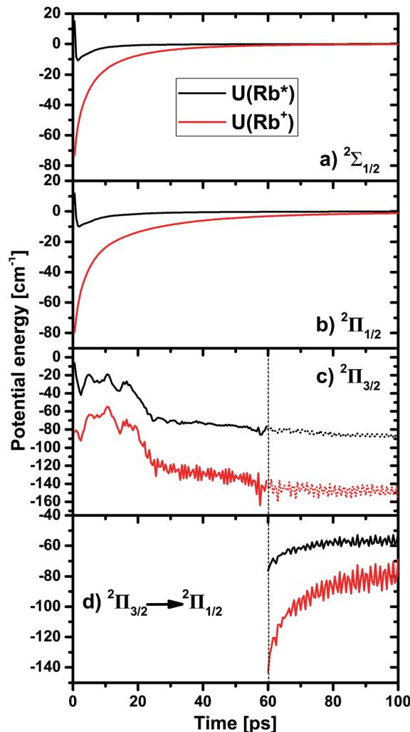
**Fig. 9** (a)–(c) Simulated interaction energies of the Rb-atom excited into various states interacting with the surrounding He distribution (black lines), and of the Rb<sup>+</sup> ion for the same instantaneous geometry (red lines). In (d), the excited state of Rb is suddenly switched from  $^2\Pi_{3/2}$  to  $^2\Pi_{1/2}$  to simulate the dynamics initiated by spin-relaxation.
