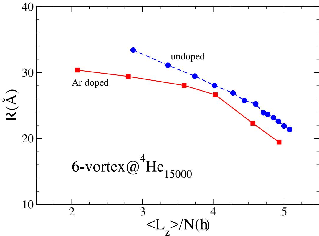
**Figure 7.4:** Calculated equilibrium distance of the 6-vortex ring from the droplet center as a function of the angular momentum per He atom in units of  $\hbar$ . The dots represent the results for undoped vortices, while the squares are the results for Ar-doped vortices. The lines are drawn as a guide to the eye.
