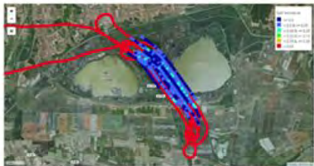
Figure II.24 – H2020 MISTRALÉ project to facilitate farming and monitoring of flooded areas from an iGNSS-R on board a RPAS ( www.mistrale.eu ), first results of the Scamandre air Campaign (South France) over a flooded pond, in red airplane trajectory, light blue to dark blue power ratio between reflected and direct waves which corresponds to moisture changes.
