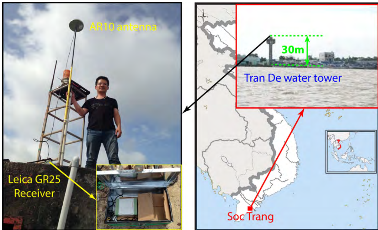
Figure IV.4 – The GNSS receiver with a single antenna set up at about 30 m above sea level, on the top of the Tran De water tower ( 106^{\circ}12'1.96''\text{E} ; 9^{\circ}31'38.37''\text{N} , MeKong Delta - Vietnam).
