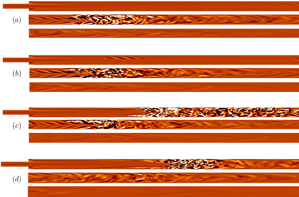
Figure 5.6: x - z cross sections of streamwise vorticity contour plot for Re = 2000 with \delta = 0.1 at (a) t = 1000 , (b) t = 1025 , (c) t = 1050 and (d) t = 1100 . Each triad represents the full pipe length, truncated at every 50d for simple visualization purpose. Here black and white corresponds to the maximum and minimum of vorticity and orange (grey) represents zero vorticity.
