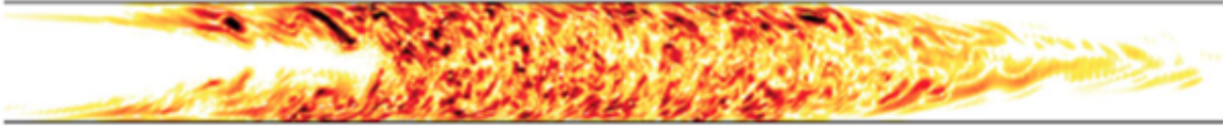
Figure 1.2: Axial vorticity plot showing a numerical puff evolution at Re=3000 . Image taken from Duguet et al. 2010 [4]
