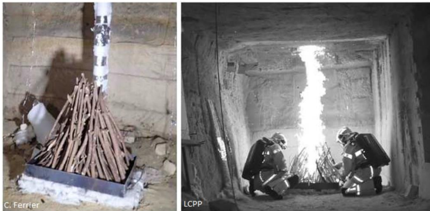
Fig. 2. On the left: Initial hearth in a tepee configuration at the back of the gallery 2. The wood is placed on a weighing scale. On the right: Wood supply by firemen with security equipment.
