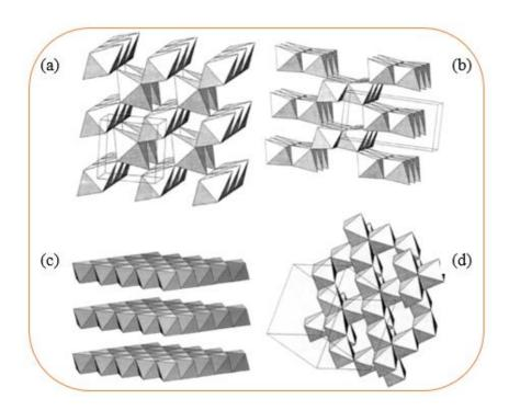
**Figure I.13.** Schematic representation of various crystal structure of MnO<sub>2</sub>: (a) pyrolusite-MnO<sub>2</sub>, (b) ramsdellite, (c) birnessite δ-MnO<sub>2</sub> and (d) spinel  $\lambda$ -MnO<sub>2</sub><sup>57</sup>.
