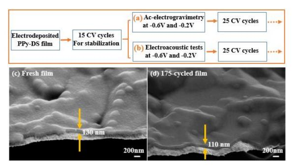
**Figure III.1.** Schematic illustration of the measurement procedures for (a) *ac*-electrogravimetry and (b) electroacoustic tests during film electrochemical cycling. The panels (c) and (d) are the morphological observations of electrodeposited fresh and 175-cycled PPy-DS film by FEG-SEM, respectively.
