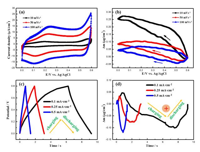
Figure V.2. Cyclic voltammetry (a) and galvanostatic charge/discharge (c) measurements of ZnO
