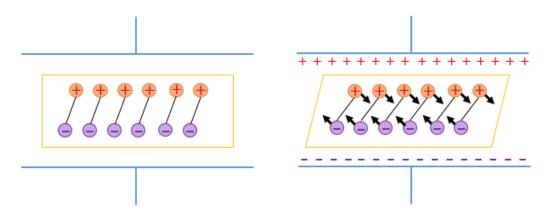
**Figure I.17.** Schematic representation of the converse piezoelectric effect for shear motion. The electric field induces reorientation of the dipoles of the acentric material, resulting in a lattice strain and shear deformation of the material. Direction of shear is dependent upon the applied potential while the extent of shear strain depends on the magnitude of the applied potential <sup>165</sup>.
