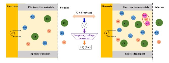
**Figure I.20.** The working mechanism of *ac*-electrogravimetry.
