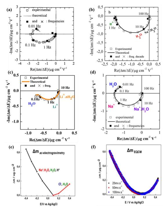
**Figure I.21.** Electrogravimetric TFs for a polypyrrole film in 0.25 M NaCl at -0.55 V vs. SCE (a), <sup>182</sup> a CNT film in 0.5 M NaCl (pH=7) at -0.4 V vs. Ag/AgCl (b), <sup>185</sup> an ERGO film in 0.5 M LiCl
