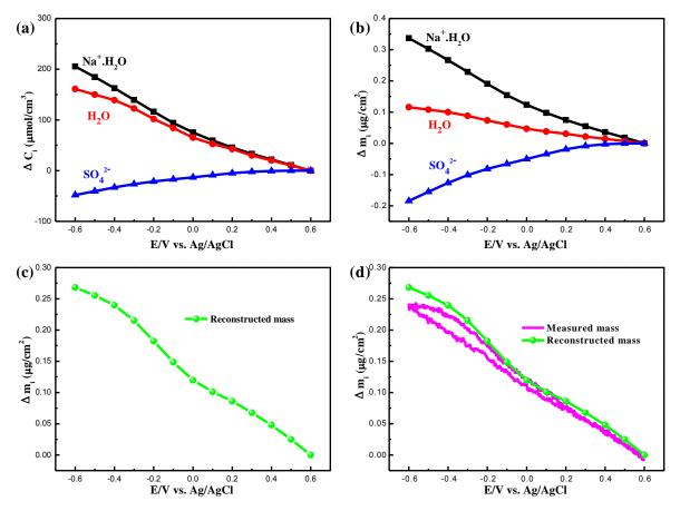
**Figure VI.4.** Relative concentration change (a) and the corresponding mass change (b) of each species as a function of potential; mass variation reconstructed from *ac*-electrogravimetry (c) and the comparison of mass variations obtained from EQCM and *ac*-electrogravimetry (d).
