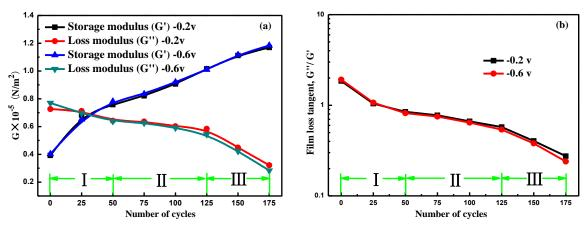
**Figure III.7.** (a) Evolution of real and imaginary components of complex shear modulus and (b) film loss tangent, G"/G', during cycling at -0.2 V and -0.6 V, respectively.
