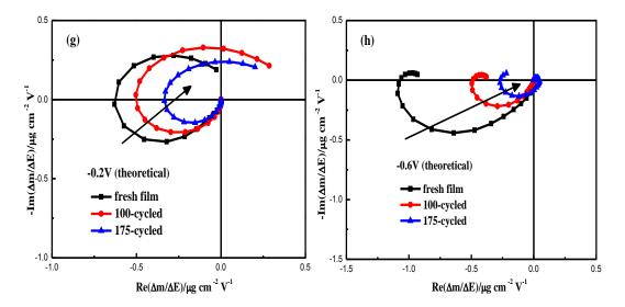
**Figure III.4.** Evolution of transfer function of  $\frac{\Delta m}{\Delta E}(\omega)$  with film cycling: (a), (c) and (e) were measured for fresh film, 100-cycled and 175-cycled film at -0.2 V, (b), (d) and (f) at -0.6 V, (g) and (h) theoretical TFs of  $\frac{\Delta m}{\Delta E}(\omega)$  as film is cycled at -0.2 V and -0.6 V, respectively.
