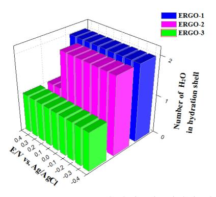
**Figure IV.12.** The evolution of number of H<sub>2</sub>O molecules in cation's hydration shell at different polarized state from -0.4 to 0.4 V for ERGO electrodes.
