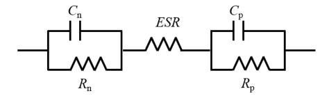
**Figure I.6.** Representation of the equivalent circuit of a symmetric EDL capacitor.  $R_{n/p}$  represents resistors and  $C_{n/p}$  denotes capacitance.
