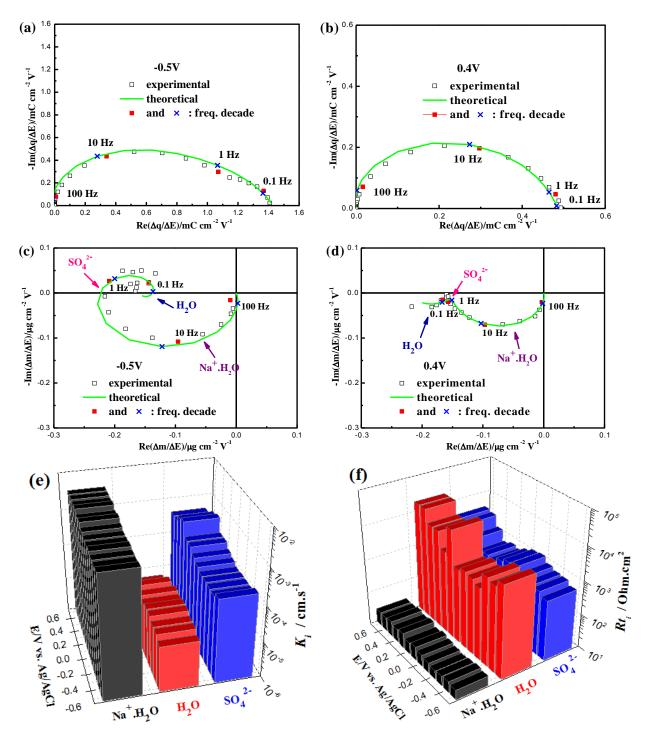
**Figure VI.3.**  $\frac{\Delta q}{\Delta E}(\omega)$  (a and b) and  $\frac{\Delta m}{\Delta E}(\omega)$  (c and d) transfer functions at -0.5V and 0.4V vs.
