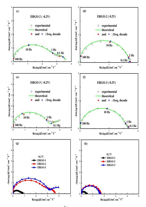
**Figure IV.9.** Experimental and theoretical  $\frac{\Delta q}{\Delta E}(\omega)$  TFs for ERGO electrodes. Panels (a), (c) and (e) are for ERGO-1, -2 and -3 at -0.2 V, while (b), (d) and (f) at 0.2 V, respectively. Panels (g) and (h)
