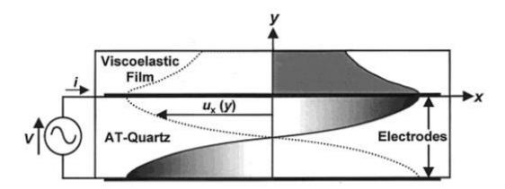
**Figure I.23.** Cross-sectional view of a quartz resonator with a viscoelastic film coating the upper surface. The thickness of the film is exaggerated relative to that of the quartz. The potential, V, creates the shear deformation in the crystal<sup>192</sup>.
