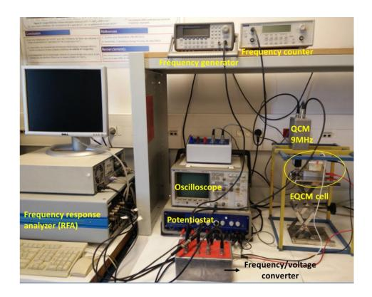
**Figure II.9.** *Ac*-electrogravimetry setup.
