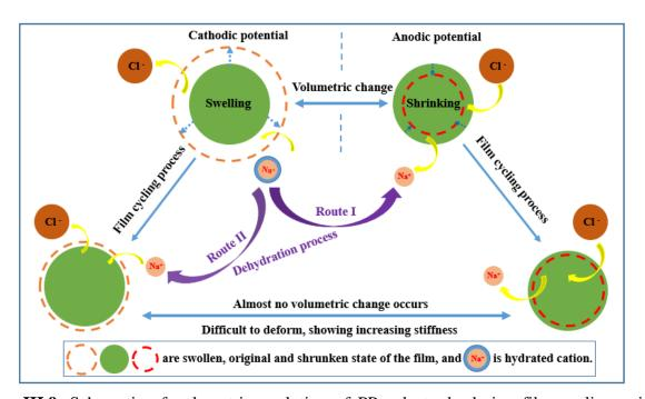
**Figure III.9.** Schematic of volumetric evolution of PPy electrode during film cycling, without considering the exchange of free H<sub>2</sub>O molecules.
