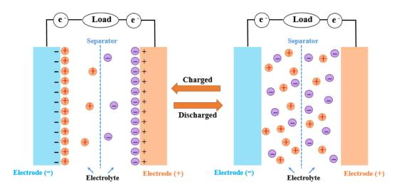
Figure I.1. Schematic illustration of a SC in a charged and discharged state.
