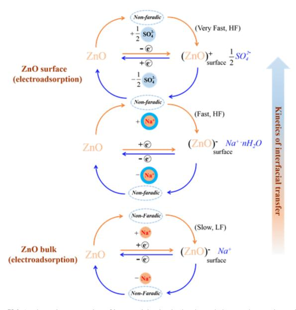
**Figure V.6.** A schematic presentation of ions participating in the charge balance, where cations with blue shell (1<sup>st</sup> step) represent the hydrated cation, i.e., Na<sup>+</sup>·nH<sub>2</sub>O (n=5).
