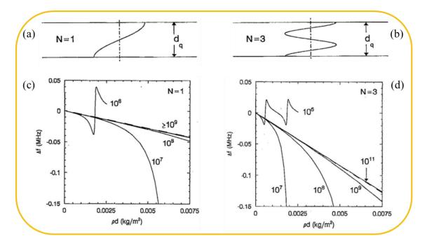
**Figure I.24.** Side cross-sectional view of AT-cut quartz wafer, showing shear displacement profiles for the fundamental (a) and third-harmonic resonances (b). Calculated effect of polymer stiffness for lossless polymers in contact with water at fundamental quartz resonance (c) and third-harmonic quartz resonance (d)<sup>191</sup>.
