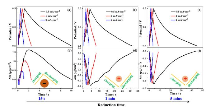
**Figure IV.6.** Galvanostatic charge-discharge of ERGO-1 (a, b), -2 (c, d) and -3 (e, f) at a current density of 0.5, 1 and 2 mA·cm<sup>-2</sup>, respectively.
