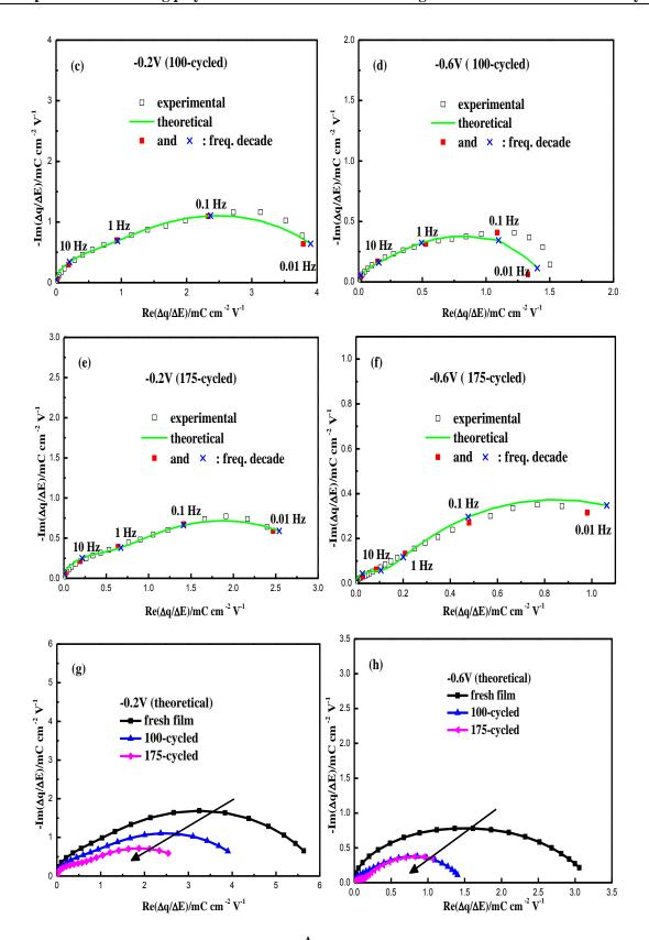
**Figure III.3.** Experimental and theoretical  $\frac{\Delta q}{\Delta E}(\omega)$  transfer functions for PPy film at different cycled state: (a), (c) and (e) were measured for fresh film, 100- and 175-cycled film at -0.2V, while
