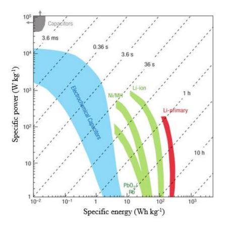
Figure I.7. Ragone plot of various electrical energy storage devices<sup>14</sup>.
