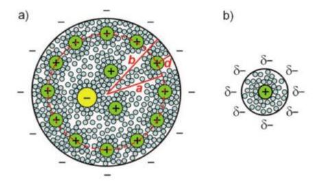
**Figure I.4.** Schematic diagrams (top views) of (a) a negatively charged mesopore with solvated cations approaching the pore wall to form an EDCC and (b) a negatively charged micropore with solvated cations lining up to form an EWCC<sup>25</sup>.
