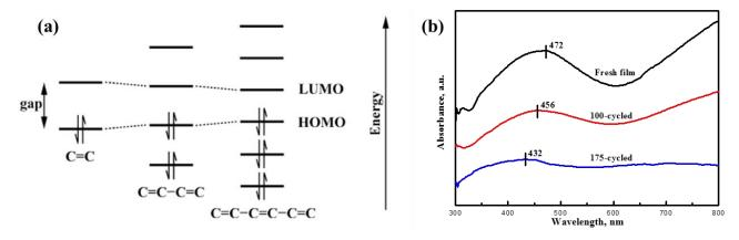
**Figure II.2.** (a) The relationship between the conjugated length in the molecule and the corresponding HOMO-LUMO gap<sup>8</sup>. (b) UV-vis spectra of fresh, 100- and 175-cycled PPy-DS film<sup>9</sup>.
