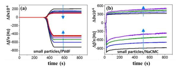
**Figure I.25.** EQCM-D data for composite LFP electrodes with PVdF (a) or NaCMC (b) containing small LFP particles. Dashed arrows show the direction of increasing  $n^{195}$ .
