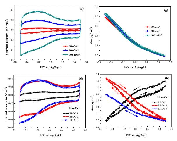
**Figure IV.7.** Cyclic voltammetry (a, b and c), mass change ( $\Delta m$ ) (e, f and g) of ERGO electrodes in 1 M NaCl aqueous solution between -0.5 V and 0.5 V vs. Ag/AgCl at different scan rates. Panels (d) and (h) are CV and mass change of ERGO electrodes obtained at 10 mV·s<sup>-1</sup>.
