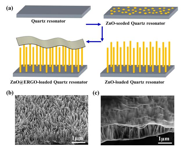
**Figure VI.1.** Schematic representation of synthetic process for ZnO@ERGO composites (a) and FEG-SEM images of ZnO nanostructures (b) and ZnO@ERGO composites (c) synthesized on the gold electrode of the quartz resonator.
