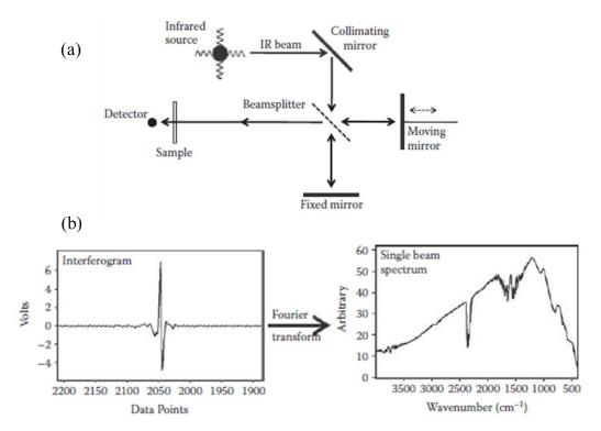
**Figure II.1.** (a) The optical diagram of a Michelson interferometer and (b) the Fourier transformation of an interferogram to a single beam spectrum<sup>1</sup>.
