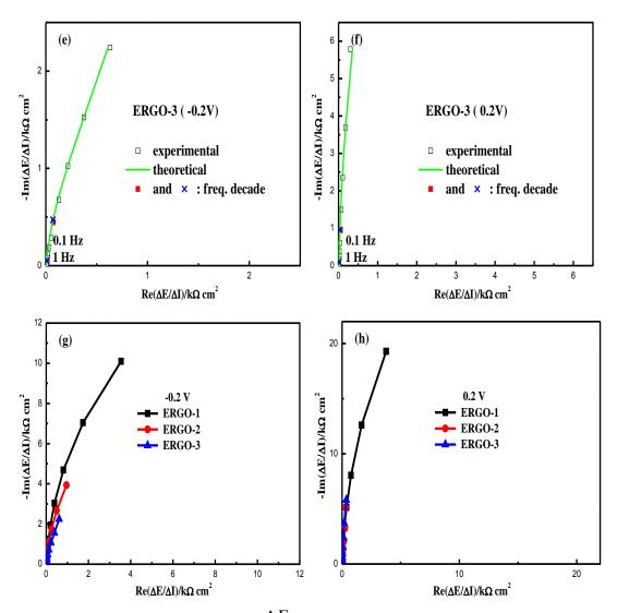
**Figure IV.8.** Experimental and theoretical  $\frac{\Delta E}{\Delta I}(\omega)$  transfer functions (TFs) for ERGO electrodes. (a), (c) and (e) were measured for ERGO-1, -2 and -3 at -0.2V, while (b), (d) and (f) at 0.2V, respectively. Panels (g) and (h) are theoretical  $\frac{\Delta E}{\Delta I}(\omega)$  TFs of ERGO electrodes at  $\pm 0.2$  V.
