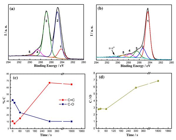
**Figure IV.4.** XPS spectra of GO (a) and ERGO-3 (b), where the curves were fitted considering the following contributions: C=C (sp<sup>2</sup>; peak 1), C-C (sp<sup>3</sup>; peak 2), C-O (epoxy and hydroxyl; peak 3), C=O (carbonyl; peak 4), O-C=O (carbonyl; peak 5) and  $\pi$ - $\pi$ \*. The panel (c) presents the relative percentage of C=C and C-O groups and the panel (d) is the C/O ratio from XPS as a function of polarization time. The lines are a guide to eyes.
