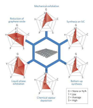
**Figure I.10.** Schematic of the most common graphene production methods. Each method has been evaluated in terms of graphene quality (G), cost aspect (C; a low value corresponds to high cost of production), scalability (S), purity (P) and yield (Y) of the overall production process<sup>112</sup>.
