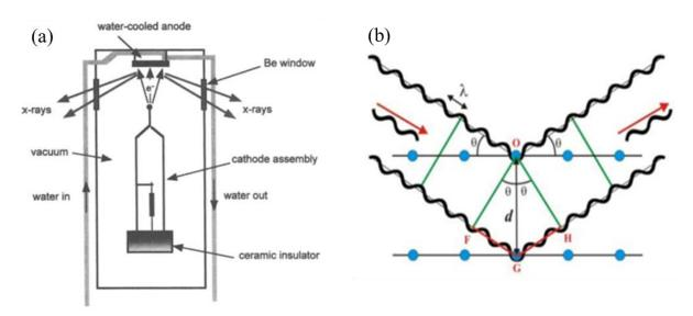
**Figure II.4.** (a) Schematic showing the essential components of a modern x-ray tube<sup>12</sup> and (b) illustration for the Bragg's law<sup>4</sup>.
