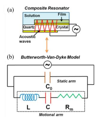
**Figure I.18.** (a) An oscillating mass-loaded quartz crystal immersed in a liquid medium acting as a composite resonator. (b) The corresponding equivalent electrical circuit as per the Butterworth-Van-Dyke Model<sup>170</sup>.
