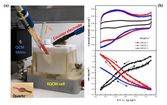
**Figure II.6.** (a) A lab-made EQCM cell and (b) EQCM results of ERGO electrodes with the different content of oxygen functionalities. The inset in (a) is the picture of quartz resonator used in the present work. The upper curve in (b) is the current response whereas the lower curve is the corresponding mass *vs.* potential profile during cycling.
