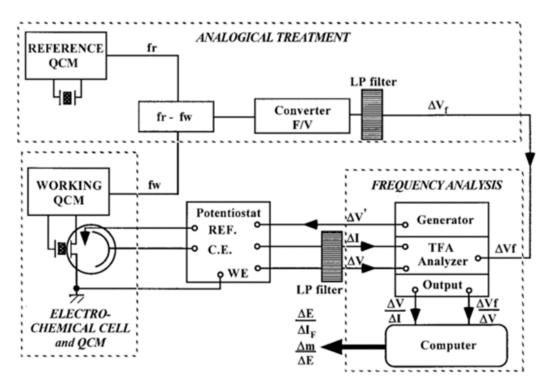
Figure II.7. Block diagram of the experimental set-up.<sup>26</sup>
