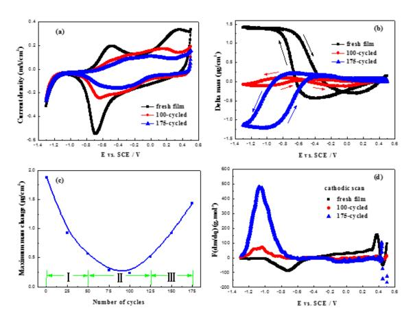
**Figure III.2.** Cyclic voltammetry (a), mass change ( $\Delta m$ ) (b), the maximum mass change (c) and F(dm/dq) function calculated from the reduction branch (d) of PPy-DS film in 0.25 M NaCl aqueous solution between -1.3 V and 0.5 V vs. SCE at a scan rate of 50 mV·s<sup>-1</sup>.
