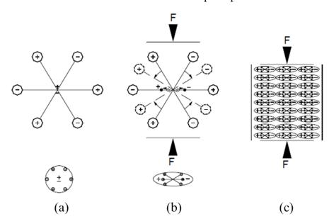
**Figure II.5.** Simple molecular model for explaining the piezoelectric effect: (a) unperturbed molecule; (b) molecule subjected to an external force, and (c) polarizing effect on the material surfaces<sup>21</sup>.
