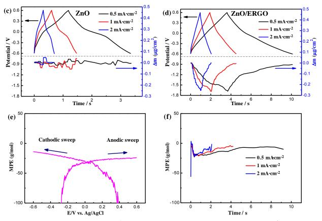
**Figure VI.2.** CV curves at 100 mV·s<sup>-1</sup> (a, b) and GCD curves at 0.5, 1 and 2 mA·cm<sup>-2</sup> (c, d) in 0.25 M Na<sub>2</sub>SO<sub>4</sub> solution; (e) and (f) are the corresponding *MPE* of ZnO@ERGO-loaded electrode calculated from a CV and GCD cycle, respectively.
