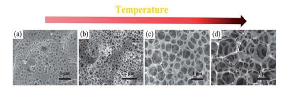
**Figure I.8.** SEM images of the samples obtained by annealing the slurry of PPy and KOH at various temperatures: (a) 500 °C, (b) 600 °C, (c) 700 °C and (d) 750 °C<sup>93</sup>.
