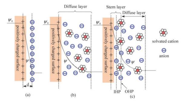
**Figure I.2.** EDL models at a positively charged surface: (a) the Helmholtz model, (b) the Gouy-Chapman model and (c) the Stern model, showing the inner Helmholtz plane (IHP) and outer Helmholtz plane (OHP). The IHP refers to the distance of closest approach of specifically adsorbed ions and OHP refers to that of the non-specifically adsorbed ions<sup>8</sup>.
