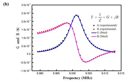
**Figure II.10.** (a) Electroacoustic impedance set-up and (b) an example for the fitting of the experimental response for ERGO-1 at -0.2 V. Fitting parameters:  $G' = 6.29 \times 10^5 \text{ N.m}^{-2}$ ,  $G'' = 0.84 \times 10^5 \text{ N.m}^{-2}$ ,  $d_f = 146 \text{ nm}$  and  $\rho_{f=2} \text{ g.cm}^{-3}$ .
