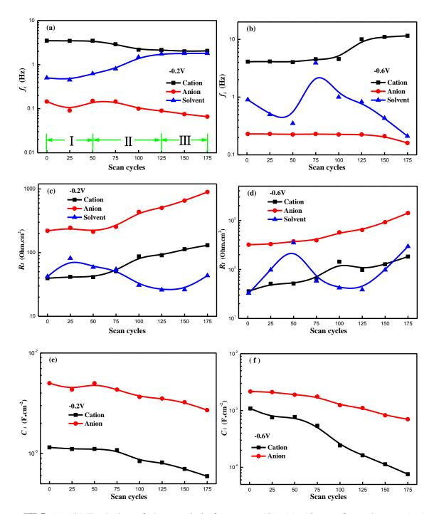
**Figure III.5.** (a), (b) Evolution of characteristic frequency  $(f_i)$ . (c), (d) transfer resistance  $(Rt_i)$  and (e), (f) instantaneous capacitance  $(C_i)$  for each species at two different potentials as the film is electrochemically cycled. Herein, anion only refers to  $Cl^-$ .
