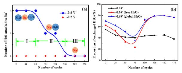
**Figure III.6.** (a) Dehydration process for hydrated cations (Na·2H<sub>2</sub>O) transferred at the film/solution interface at -0.6 V as the film is electrochemically cycled, and (b) proportion of exchanged H<sub>2</sub>O (calculated using **Equations III.12** and **III.13**) participating in charge compensation at both potentials. Global H<sub>2</sub>O represents the sum of free H<sub>2</sub>O and the H<sub>2</sub>O molecules within the hydration shell of cations.
