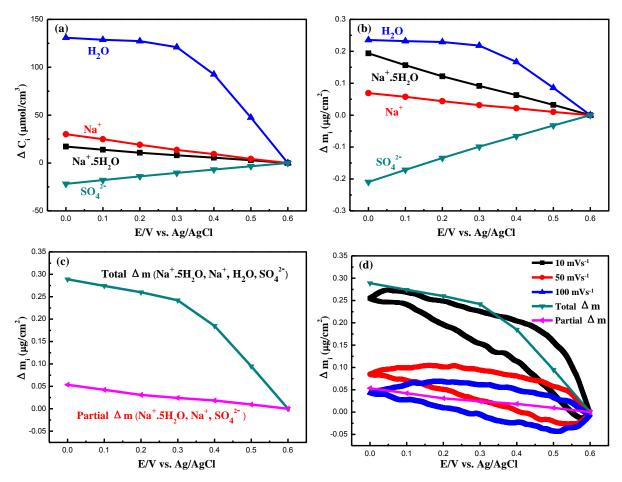
**Figure V.7.** Relative concentration change (a) and the corresponding mass change (b) of each species as a function of potential; mass variation (total and partial  $\Delta m$ ) reconstructed from ac-electrogravimetry (c) and the comparison of mass variation between ac-electrogravimetry and EQCM (d).
