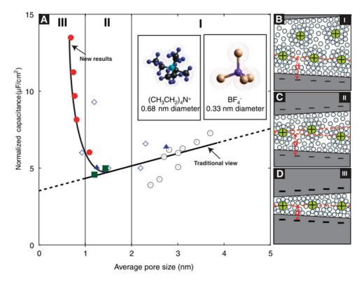
**Figure I.3.** (A) normalized capacitance for the carbons; B to D schematically illustrate the solvated ions in electrode pores with distance between adjacent pore walls (B) greater than 2 nm, (C) between 1 and 2 nm, and (D) less than 1 nm<sup>6</sup>.
