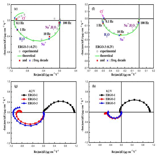
**Figure IV.10.** Evolution of  $\frac{\Delta m}{\Delta E}(\omega)$  TFs with progressive reduction of the ERGO electrodes: (a), (c) and (e) were measured for ERGO-1, -2 and -3 at -0.2V, while (b), (d) and (f) at 0.2V, respectively. Panels (g) and (h) are theoretical  $\frac{\Delta m}{\Delta E}(\omega)$  TFs of ERGO electrodes at  $\pm 0.2$  V.
