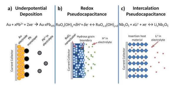
**Figure I.5.** Different types of reversible redox mechanisms that give rise to pseudocapacitance: (a) underpotential deposition, (b) redox pseudocapacitance, and (c) intercalation pseudocapacitance<sup>26</sup>.
