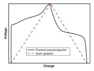
**Figure I.15.** Schematic galvanostatic charge/discharge response of supercapacitor devices: pseudocapacitor and ideal EDLC<sup>162</sup>.
