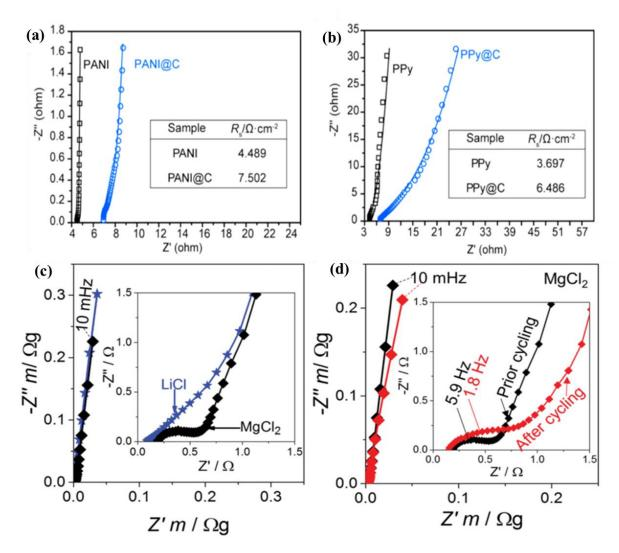
**Figure I.16.** (a, b) Nyquist plots of polymer and carbonaceous shell-coated polymer electrodes measured in 1 M  $H_2SO_4$  at open circuit potential. Insets show the  $R_s$  values of the electrodes<sup>27</sup>; (c, d) impedance spectra of  $Ti_3C_2Tx$  electrode (inset presents enlarged view of high-frequency domain)<sup>164</sup>.
