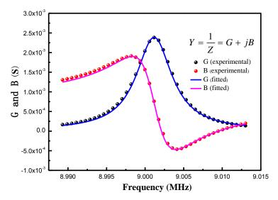
**Figure IV.1.** Electroacoustic admittance measurements: experimental and fitted conductance and susceptance over frequency for ERGO-1 at -0.2 V. Fitting parameters:  $G' = 6.29 \times 10^5 \, \text{N.m}^{-2}$ ,  $G'' = 0.84 \times 10^5 \, \text{N.m}^{-2}$ ,  $d_f = 146 \, \text{nm}$  and  $\rho_f = 2 \, \text{g.cm}^{-3}$ .
