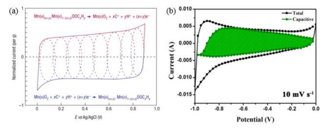
**Figure I.14.** (a) Schematic of CV for a  $MnO_2$  electrode cell in mild aqueous electrolyte (0.1 M  $K_2SO_4$ ) shows the successive multiple surface redox reactions leading to the pseudocapacitive charge storage mechanism<sup>14</sup>. (b) CV of  $Fe_2O_3$ /nitrogen-doped graphene composite tested in 2 M KOH solution at 10 mV s<sup>-1</sup>, and the shadowed areas represent the capacitive contribution<sup>155</sup>.
