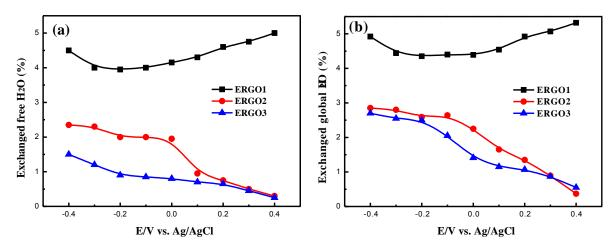
**Figure IV.13.** Exchanged free H<sub>2</sub>O (a) and global H<sub>2</sub>O (b) (calculated by **Equations IV.11** and **IV.12**) participating in charge compensation at each polarized state.
