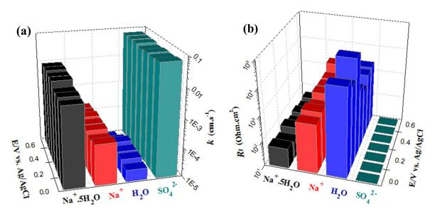
**Figure V.5.** Transfer kinetics,  $K_i$  (cm·s<sup>-1</sup>) (a) and corresponding transfer resistances,  $Rt_i$  ( $\Omega$ ·cm<sup>2</sup>) (b) for each species participating in charge balance.
