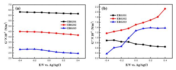
**Figure IV.5.** Evolution of real (a) and imaginary (b) components of complex shear modulus of ERGO electrodes.
