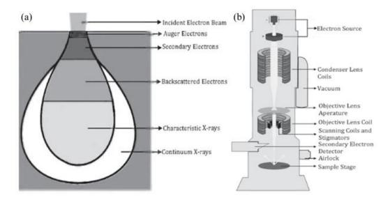
**Figure II.3.** (a) Signals generated by interaction of electron beam and specimen and regions from which each signal type can be detected. (b) Scanning electron microscope<sup>2</sup>.
