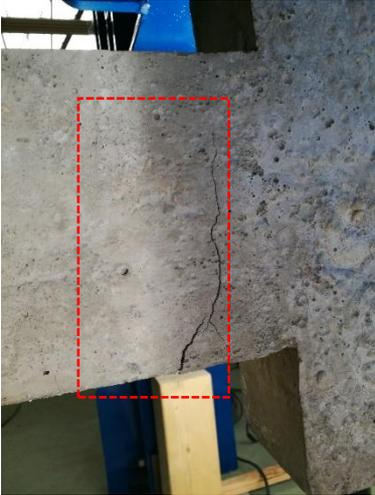
Figure 3. 33 Crack development after the first loading at 994kg
