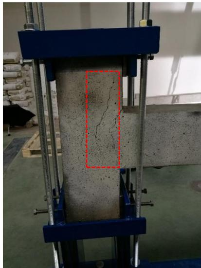
Figure 3. 35 Crack development under the third loading at 994 kg
