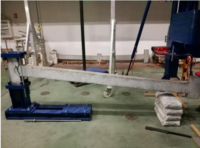
Figure 3. 38 Failure mode of the structure under the load of 2063kg
