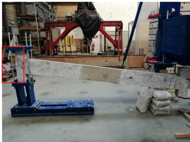
Figure 3. 47 Damage of structure under the load of 2737kg at the end of the test
