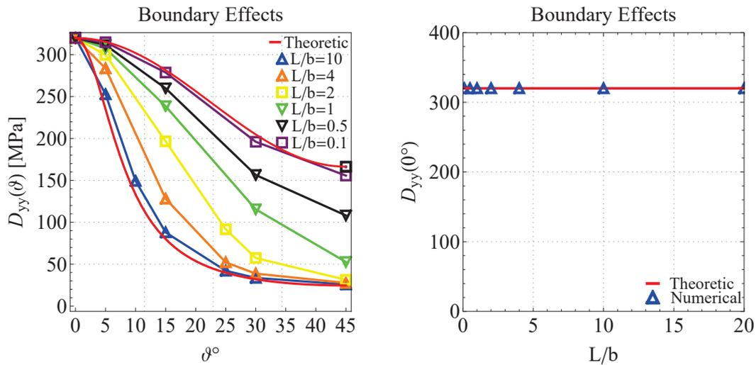
(a) Apparent elastic modulus of the specimen  $D_{yy}$  as function of the fibre direction for different aspect ratio of the specimen
