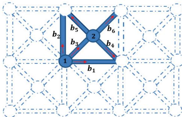
Figure 3.8: Reference cell rectangular braced with pivot
