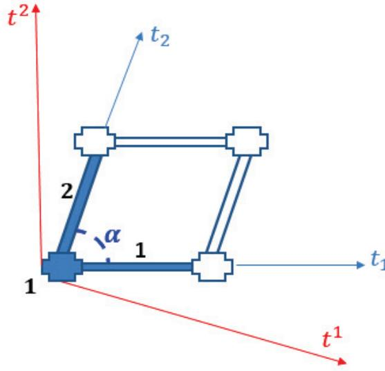
Figure 3.4: Reference cell rhomboedral case with rigid connection
