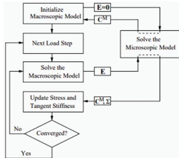
Figure 1.10: Flowchart of the multi-scale procedure. (The figure has been reproduced from [73]).
