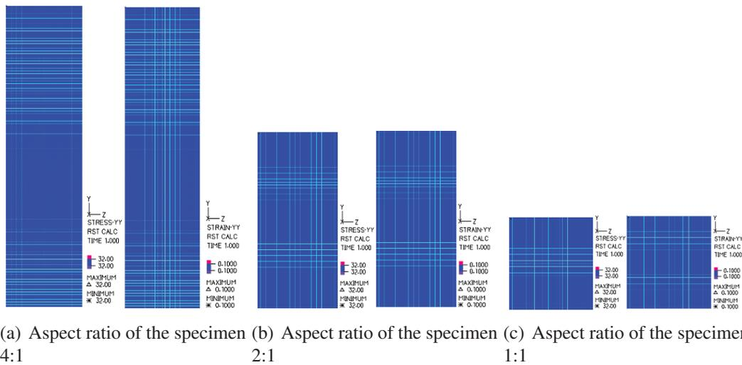
Figure 4.7: Plot of the strain  $\varepsilon_{yy}$  and the stress  $\sigma_{yy}$  for an extension test of a network with square reference cell. The fibre's axis is coincident with the axis of the specimen.
