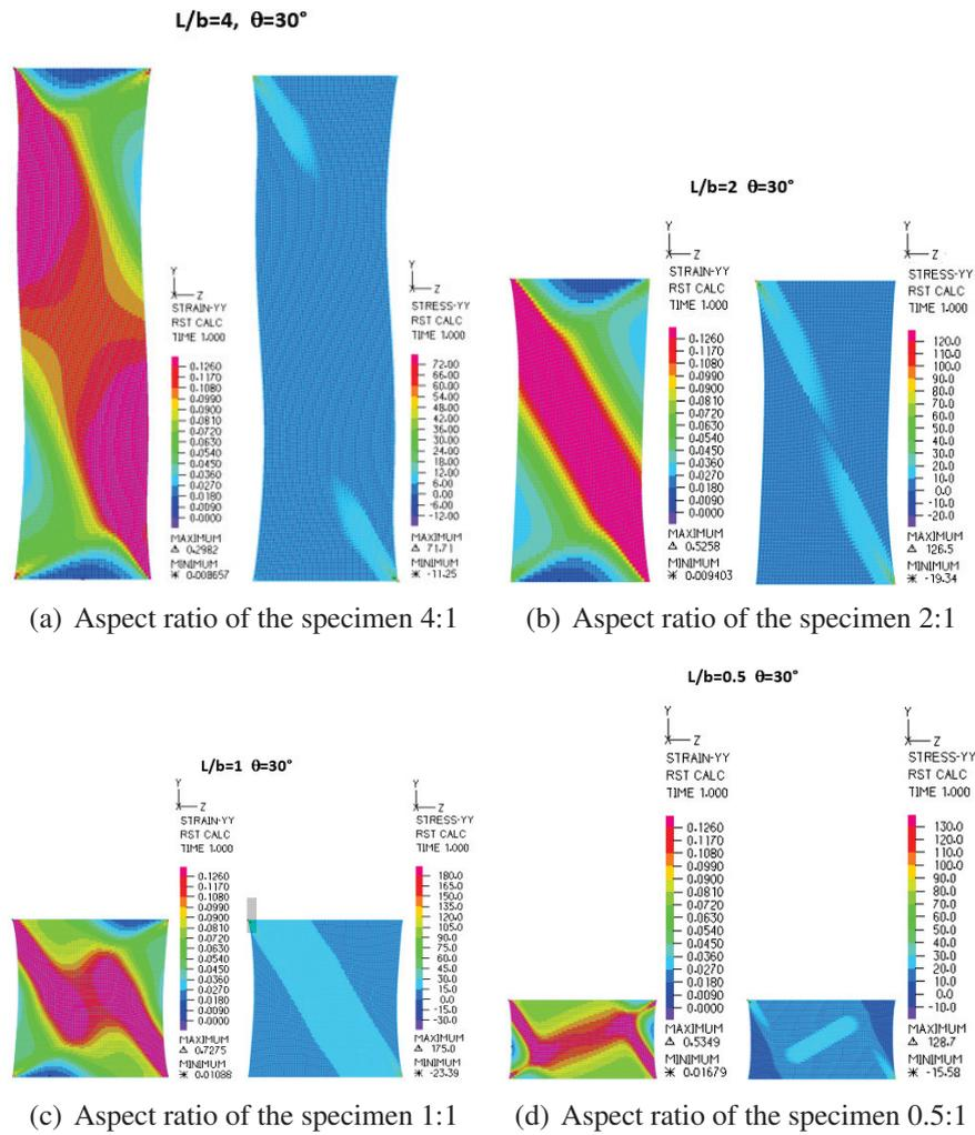
Figure 4.8: Plot of the strain  $\epsilon_{yy}$  and the stress  $\sigma_{yy}$  for an extension test of a network with square reference cell having the fibre's direction rotated by  $\theta = 30^\circ$  respect the axis of the specimen.
