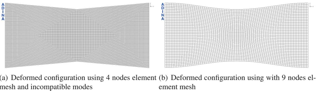
(a) Deformed configuration using 4 nodes element mesh and incompatible modes (b) Deformed configuration using with 9 nodes element mesh
