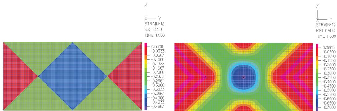
(c) Shear strain  $\gamma_{12}$  using 4 nodes element mesh and incompatible modes (d) Shear strain  $\gamma_{12}$  using 9 nodes element mesh
