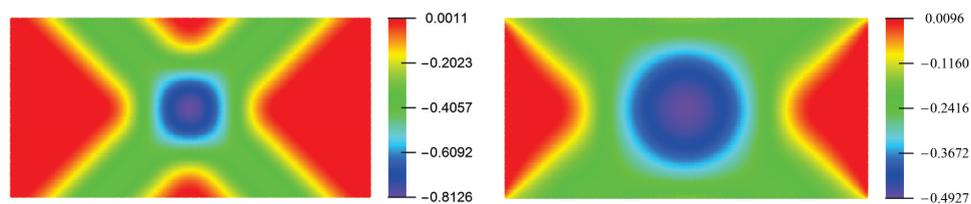
(a) Shear strain  $\gamma_{12}$ , only first gradient is considered
