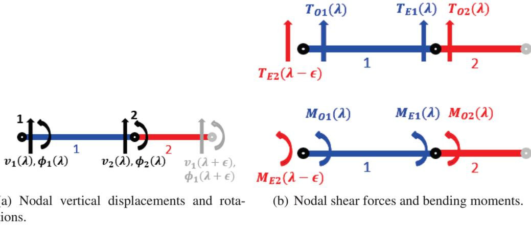
(a) Nodal vertical displacements and rotations. (b) Nodal shear forces and bending moments.
