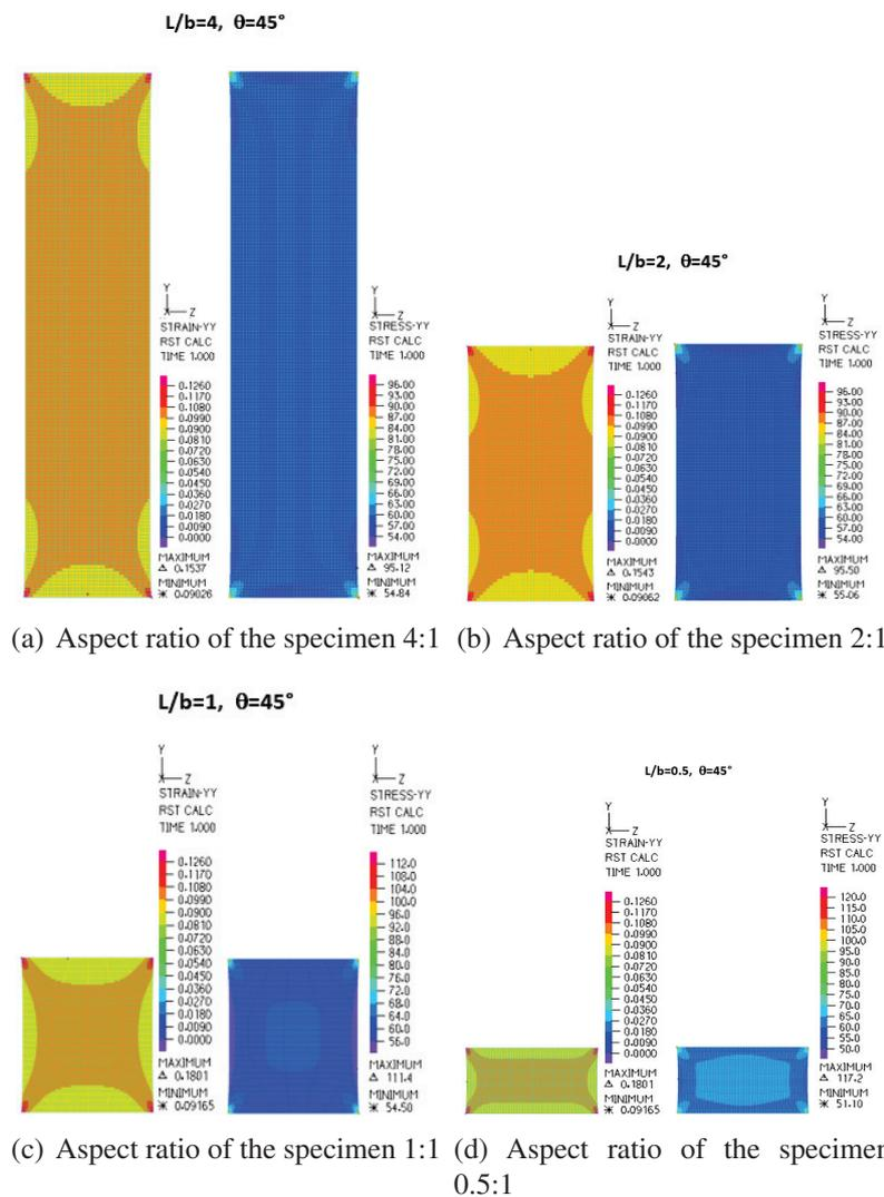
Figure 4.3: Plot of the strain  $\varepsilon_{yy}$  and the stress  $\sigma_{yy}$  for bias test of a network with square braced reference cell with rigid connections varying the aspect ratio of the specimen.
