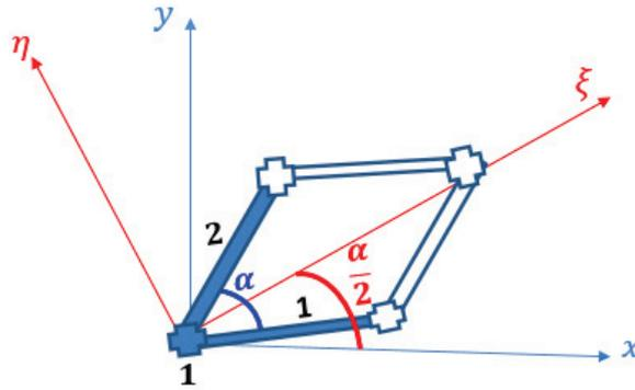
Figure 3.5: Reference cell rhombohedral case with rigid connection
