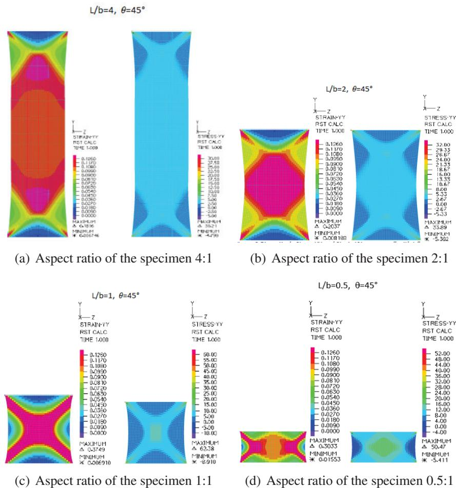
Figure 4.2: Plot of the strain  $\varepsilon_{yy}$  and the stress  $\sigma_{yy}$  of a numerical bias test of a network with square reference cell varying the aspect ratio of the specimen.
