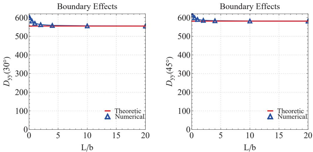
(c) Apparent elastic modulus  $D_{yy}$  as function of different aspect ratio of the specimen for the main fibre direction rotated by  $30^\circ$  respect the specimen axis.
