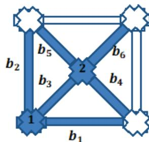
Figure 3.7: Reference cell rectangular braced with rigid connection
