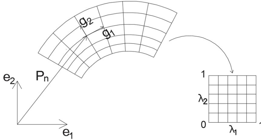
Figure 2.9: Mapping for the parametric space
