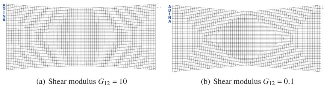
Figure 4.18: Deformed configurations for two values of the equivalent shear modulus  $G_{12}$
