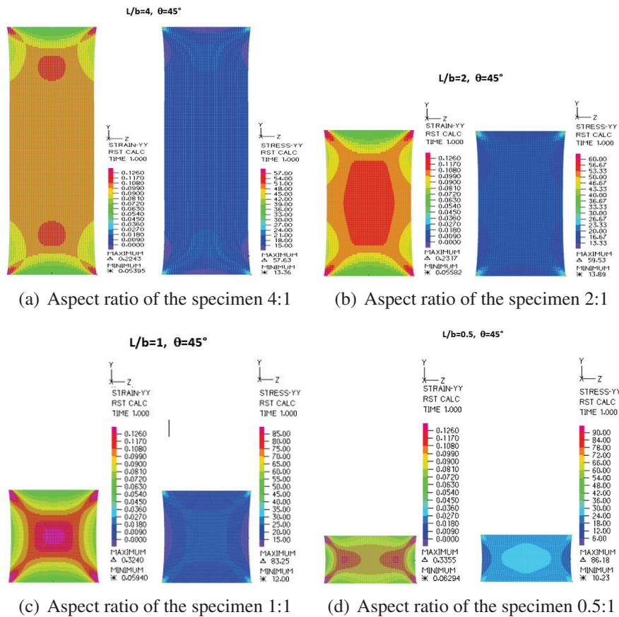
Figure 4.4: Plot of the strain  $\epsilon_{yy}$  and the stress  $\sigma_{yy}$  for bias test of a network with square braced cell with rigid connections. Ratio of the Young modulus of the internal fibres to the Young modulus of the mean fibres, equal to 1/5.
