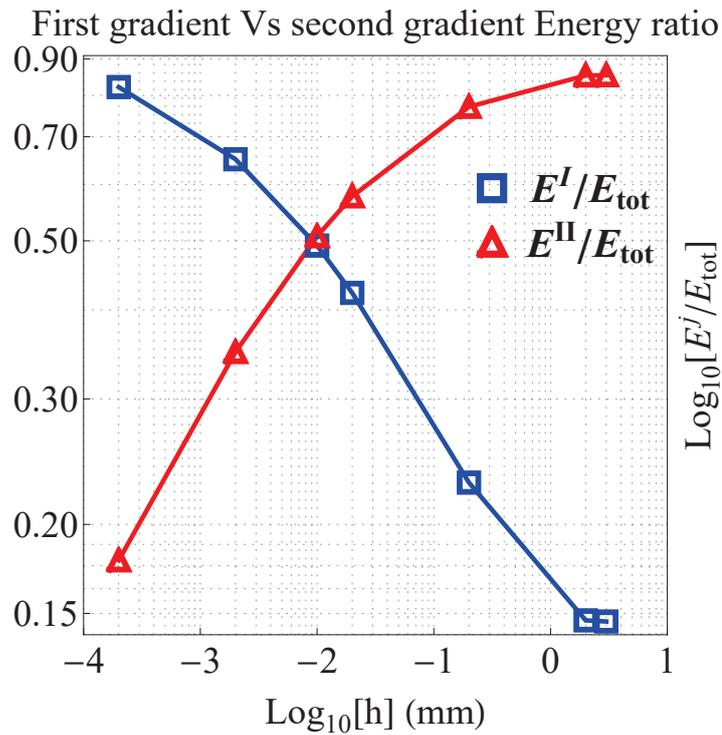
Figure 4.26: Ratio between the first gradient energy and the total energy and ratio between the second gradient energy and the total energy vs. height of the microbeams.
