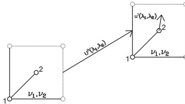
Figure 2.10: The figure show the displacement of the reference cell  $\mathbf{U}^0(\lambda_1, \lambda_2)$ , and the displacement of the internal node  $\mathbf{u}_n^1(\lambda_1, \lambda_2)$  at the first order.
