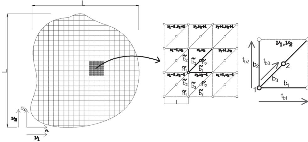
Figure 2.8: Numbering of the bars and nodes
