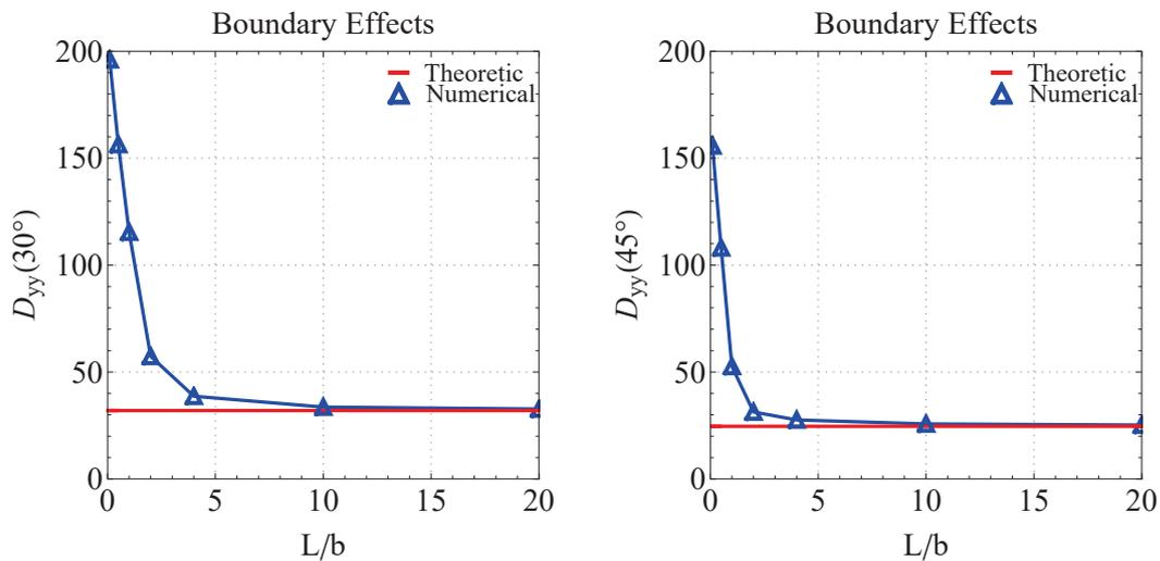
(c) Apparent elastic modulus  $D_{yy}$  as function of different aspect ratio of the specimen for the fibre direction rotated by  $30^\circ$  respect the specimen axis.
