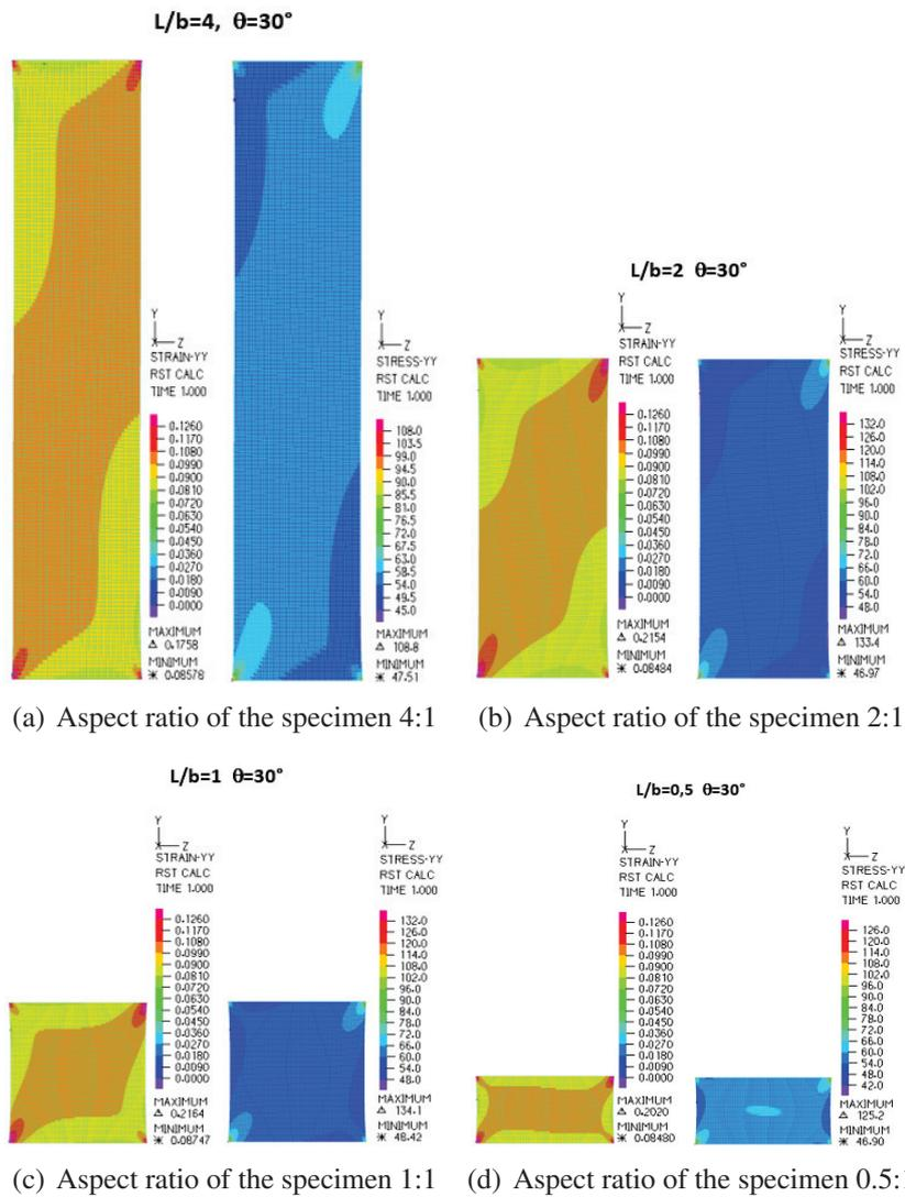
Figure 4.11: Plot of the strain  $\varepsilon_{yy}$  and the stress  $\sigma_{yy}$  for an extension test of a network with square braced cells rigidly connected having the main fibre's direction rotated by  $\theta = 30$  respect the axis of the specimen.
