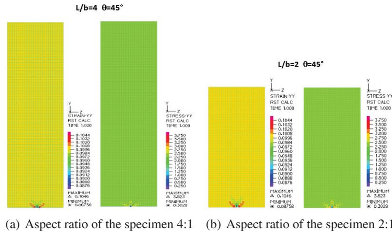
Figure 4.6: Plot of the strain  $\varepsilon_{yy}$  and the stress  $\sigma_{yy}$  for bias test of a network with square reference cell. Lateral deformation allowed at the lower edge.
