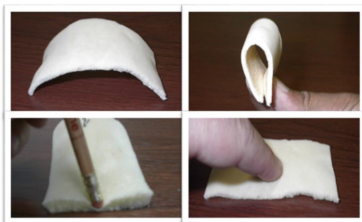
Figure 19. Flexible foam material from hemicellulose citrate chitosan. From top left clockwise: unstressed foam, folded foam, localized impression, and flattened foam. After each of these deformations the unstressed shape of the foam returns. Reproduced from [105]
