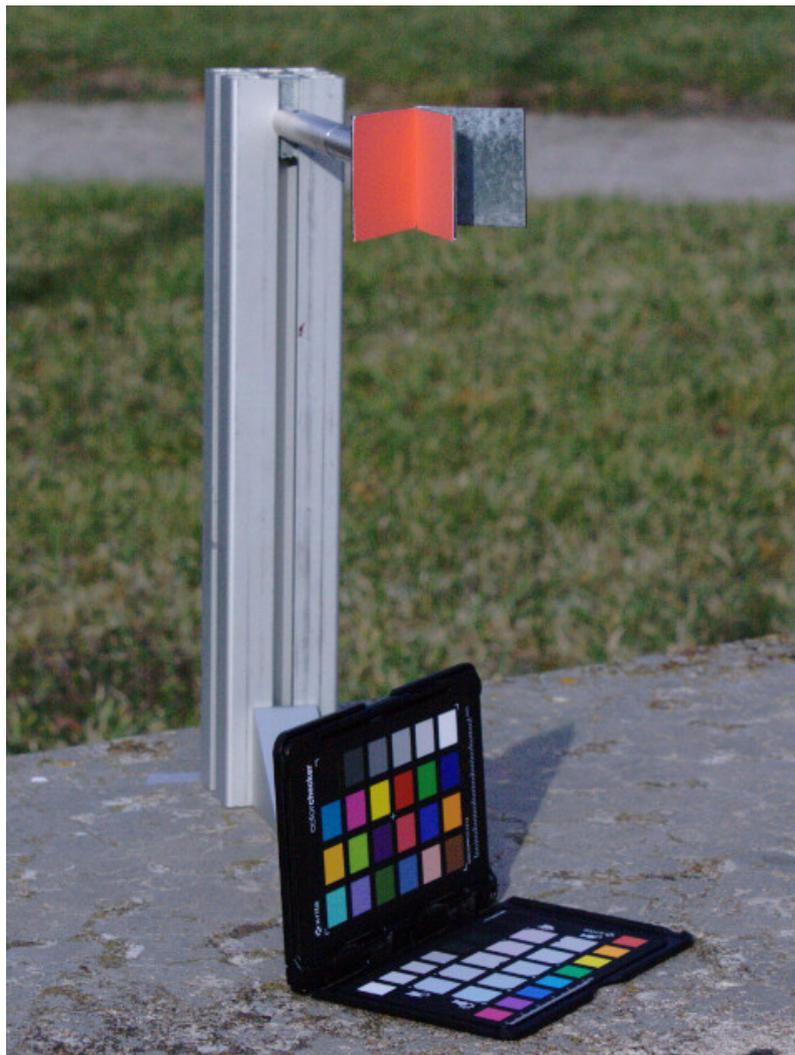
Figure 5.1: *Example of acquisition: The Munsell V-cavity on the top and the X-Rite Color Checker on the bottom under direct sun light.*
