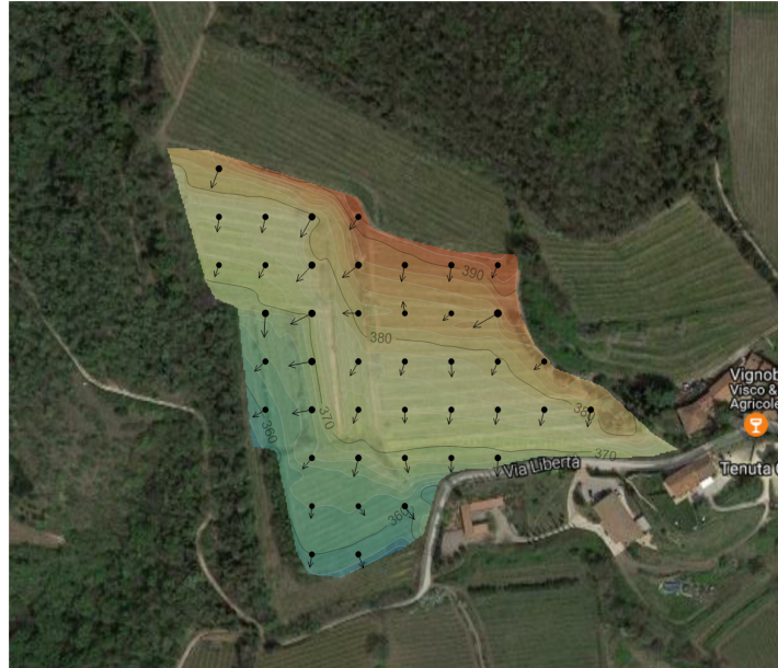
Figure 5.9 – Map of elevation and slope direction of the studied vineyard plots interpolated from differential kinetic GPS measurements.
