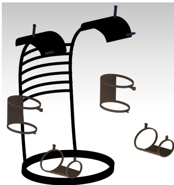
Figure 4-1. Rigid frame of the robotic suit.
