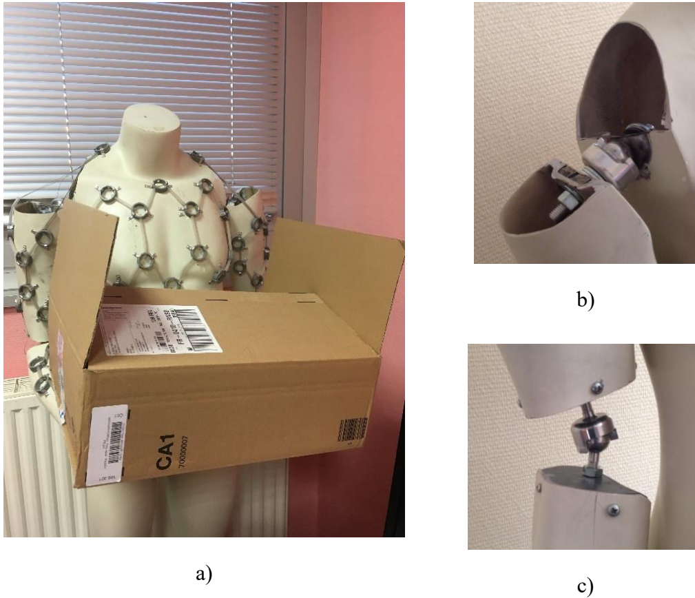
Figure 4-15. Mannequin test bench (a) and the added joints (b, c).
