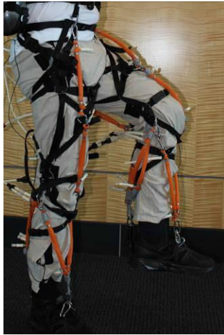
(a) Pneumatically actuated exosuit
