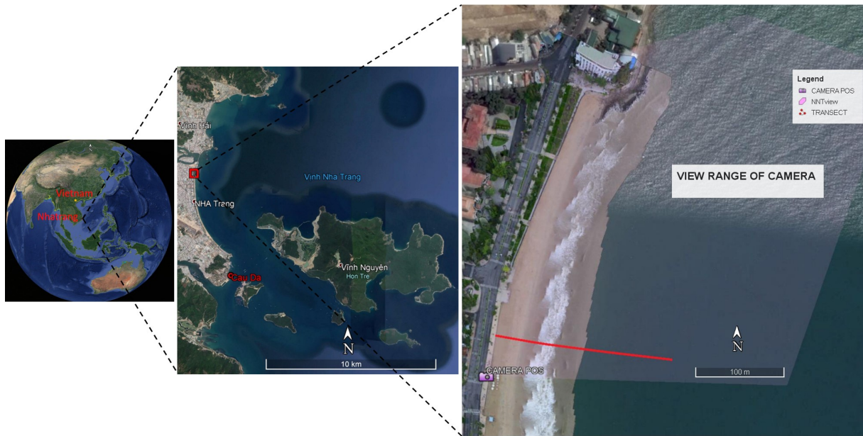
Figure 6.1: Study area in the central part of Nha Trang bay, Vietnam. The Camera view range is represented by transparent pink color, the red solid line presents the profiling location where cross-shore time stack images are created for depth inversion.
