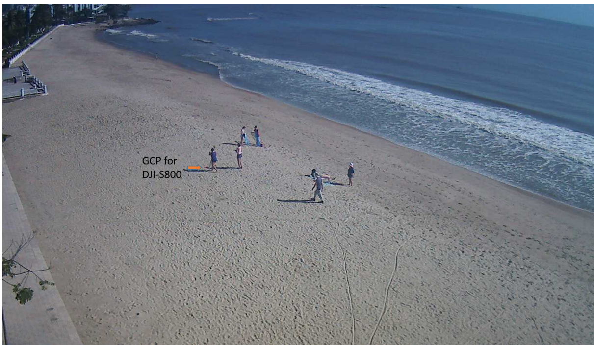
Figure 7.1: This illustrates GCPs measurement using the RTK-GPS device for transformation of SfM image-space coordinates into a physical coordinate system of the DJI-S800 drone. Images obtained from NNT camera system.
