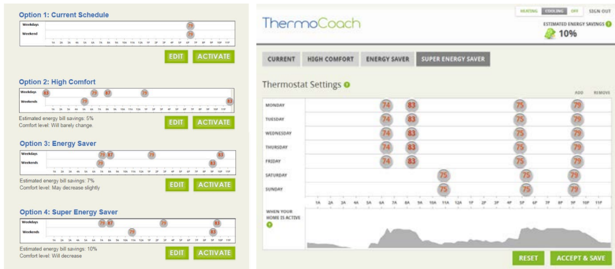
Figure 6.3. (left) Four schedule propositions from ThermoCoach, (right) Inhabitants can review/modify and activate the schedule that they found suitable
