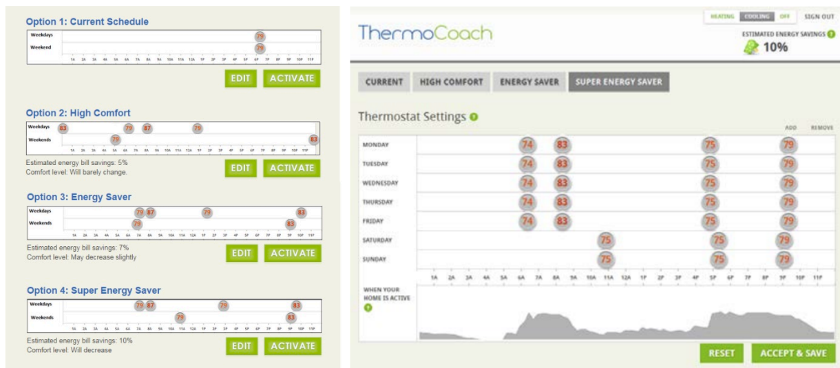
Figure 6.3. (left) Four schedule propositions from ThermoCoach, (right) Inhabitants can review/modify and activate the schedule that they found suitable
