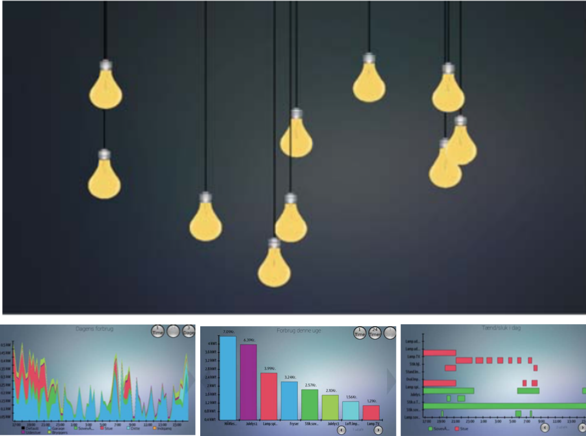
Figure 4.7. (top) PowerViz [128] screen saver: overall consumption represented by light bulbs, (bottom) in-depth analysis screens: (left to right) Usage History, Appliance Usage and Appliance history.
