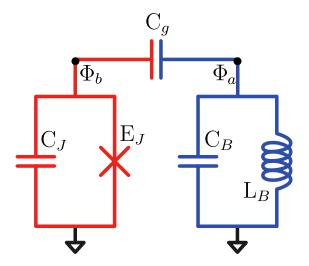
Figure 2.1: Lumped element circuit of a transmon coupled to a harmonic oscillator (microwave cavity). This lumped element circuit depicts a transmon (here in red) with a capacitance  $C_J$  and a Josephson energy  $E_J$  for the junction, capacitively coupled (through a capacitance  $C_g$ ) to a microwave cavity (harmonic oscillator, here in blue) with a capacitance  $C_B$  and an inductance  $L_B$ .
