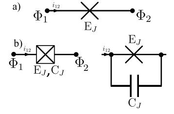
Figure 1.4: **Electrical symbols for a Josephson junction**. a) Electrical symbol of a pure Josephson junction. b) Due to the layered structure of a real Josephson junction, it always comes with an extra capacitance. Such a Josephson junction is pictured as a boxed Josephson junction, representing a junction with a capacitance in parallel.
