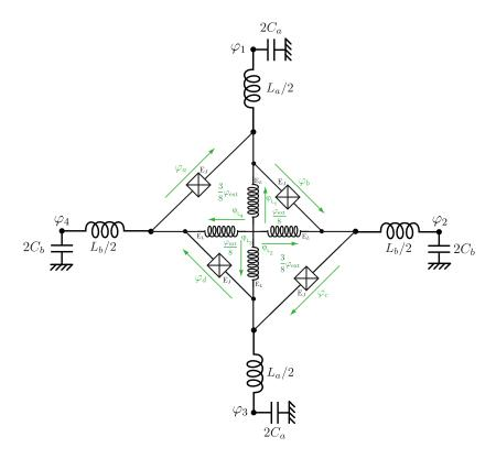
Figure 5.6: Electric circuit for the Asymmetric Josephson Ring Modulator embedded into  $\lambda/2$  resonators. The AJRM circuit from section 5.2 is embedded here into  $\lambda/2$  resonators to couple it with microwave modes of a 3D cavity. I am here considering a particular  $\lambda=3$  ratio between the areas of the inner loops, resulting in a perceived magnetic flux  $3\varphi_{\rm ext}/8$  in the larger loops and  $\varphi_{\rm ext}/8$  in the smaller loops.
