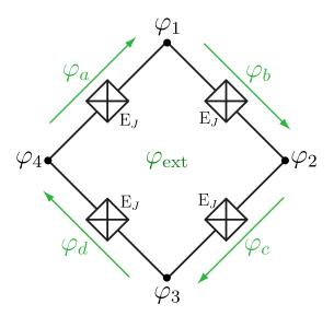
Figure 5.1: Electric circuit for the unshunted Josephson Ring Modulator. The JRM consists of a single loop of four Josephson junctions with the same Josephson energy  $E_J$  and capacitive energy  $E_C$ , all in series. An external reduced magnetic flux  $\varphi_{\text{ext}}$  is threading the loop. We denote by  $\{\varphi_{\mu}\}_{\mu=a,b,c,d}$  the flux across each of these junctions and  $\{\varphi_k\}_{k=1,2,3,4}$  the node fluxes at each vertex of the loop.
