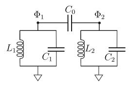
Figure 1.5: Lumped element circuit of two microwave oscillators capacitively coupled. This lumped element circuit consists of two microwave cavities (LC oscillators with parameters  $L_1$ ,  $C_1$  and  $L_2$ ,  $C_2$ ) capacitively coupled through a capacitor  $C_0$ . The node fluxes  $\Phi_{1,2}$  at each end of the coupling capacitor are shown as well.
