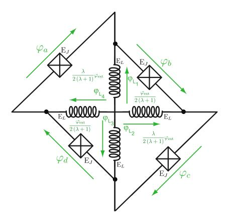
Figure 5.5: Electric circuit for the Asymmetric Josephson Ring Modulator. This circuit is the same as the Josephson Ring Modulator with shunt inductances circuit from Fig. 5.4 except that the inner loops now have different areas, in a ratio  $\lambda$ .
