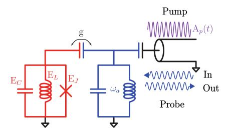
Figure 3.1: Circuit of a transmon, shunted with an inductance and coupled to a harmonic oscillator (microwave cavity) and capacitively coupled to a transmission line. A (strong) pump at frequency  $\omega_p$  is sent to the system through the transmission line, similarly to the setup presented in Fig. 2.2. The extra inductance in the transmon mode should provide an extra harmonic confinement and therefore allow for a larger span of exploitable pump strengths.
