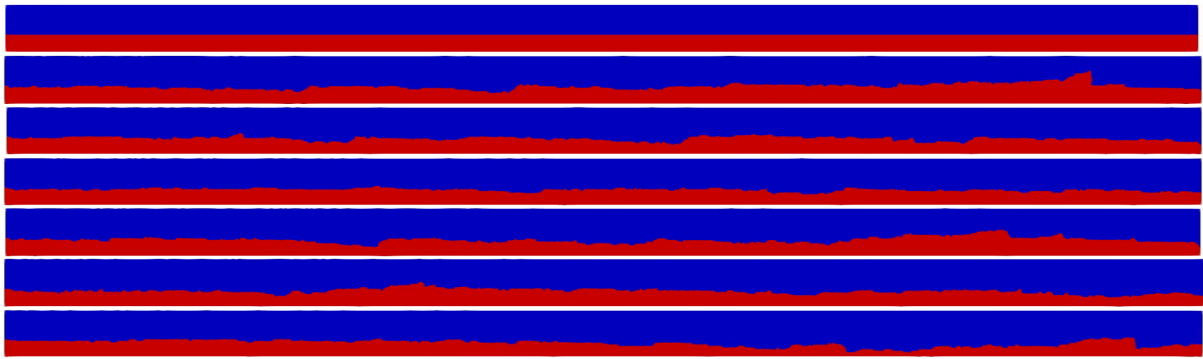
Figure 5.28: Phases distribution for the hydrodynamic slugging case (not at scale). From top to bottom, at t = 0 s, 5 s, 10 s, 15 s, 20 s, 25 s and 30 s
